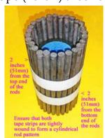
10) **Refer to the photo below**. Take the Oatey 4 inch x 4 inch (102mm x 102mm) foam closet spacer pack (Part D) and remove the label and internal staple. Unroll the foam,
