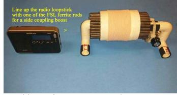
inductive coupling distance is also found, the resulting signal boost from your new FSL antenna is competitive with that of a much larger (4 foot, or 1.22 meter) air core box loop. Practice and skill in optimizing both of these adjustments will provide excellent DXing results with your new antenna.
