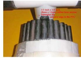
fitting edge until the glue sets. (Note: This rubber hose section will prevent unwanted rotation of the ferrite sleeve, and provide some protection against accidental bumps during airline travel).
