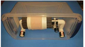
Although the design of this antenna (with the internal variable cap) can allow it to continue operating during periods of light rain, during such weather it is far preferable to place the antenna inside of its matched-size plastic tote, as **shown in the photo at left**. While protected in this way the antenna can operate in all but the most severe weather.
