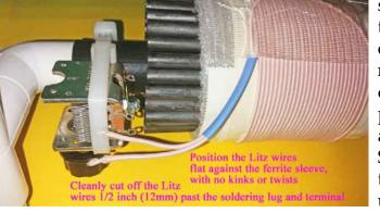
shown, and then press the two Litz wires flat against the bottom of the ferrite sleeve with the ends passing over the variable cap (as shown). Ensure that there are no twists, kinks or sharp bends in the Litz wires, then cut the Litz wires cleanly with sharp scissors (as in the previous step) 1/2 inch (12mm) past the soldering lug and variable cap terminal (that was bent outward in Step 26). As you cut the Litz wires take care to ensure that the individual wires and insulation do not unravel.
