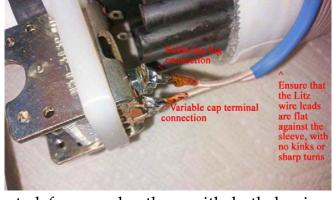
antenna, and that these two connections are well separated from each other, with both having bright, shiny solder joints, as **shown in the photo**.
