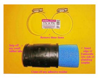
2) **Refer to the photo at left**. Place the open end of the plumbing coupler flat on a table, and push the Funnoodle as far down as possible with flat hand pressure. Then work around the edge of the
