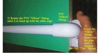
glue is applied will be to "bottom out" the pipe stub from the "Tee" fitting up into the "Elbow" fitting (which will make the two fittings touch together, since the stub is too short to fill the open space), and the second step will be to rotate the "Elbow" fitting to an exact perpendicular angle with the "Tee" fitting.
