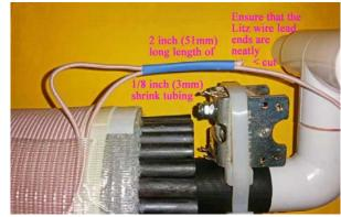
well (as shown). Finally, position the shrink tubing as shown in the **next photo**.
