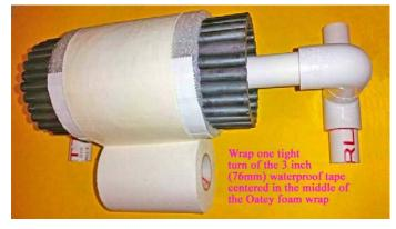
without any gaps or overlaps. During the winding of the Litz wire coil, ensure that these three tape strips remain in these interlocking positions adjacent to each other, without any gaps or overlaps.
