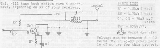
The project should be mounted in an insulated metal box.
