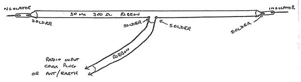
Although the antenna is resonated on 60 metres it will work satisfactorily on other bands . If required the antenna can be cut for other SW bands using the formula in the August " Times " . To test the antenna after installation use a multimeter . When connecting the meter across the feedline one should get a very low resistance. If there is a high resistance then check for an " open " wire or a faulty solder joint .
