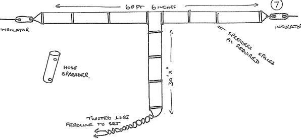
From the above diagram and measurements one can calculate that Tom's antenna is a half wave on 40 metres with a quater wave matching stub. From the bottom of the stub, a twisted wire lead in is connected. Compared with his 187 foot long wire Tom has found the folded dipole only 17 db down and against his whip it is 3 db up . For further information recarding this antenna Ken will be pleased to oblige . Kens address is 298 Ocean Beach Road , Mt. Maunganui .
