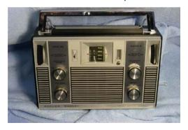
The Barlow Wadley portable solid state radio. A super performance AM and SW radio that utilizes the "Wadley Phase loop system". Manufactured by Barlows Television Co., New Germany, Natal, South Africa.
