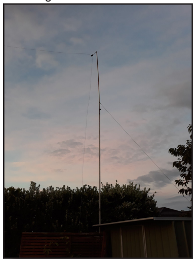
Mike's newly refurbished EWE antennae - the pole common to both EWEs (left) and the other end of one of them (right)
