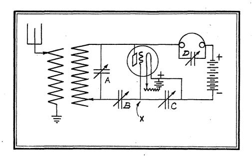
so that the Audion will oscillate. Once the Audion is generating undamped waves, the set is tuned with the loose coupler and the signals heterodyned. This merely means "beats" are produced. The operator can vary the frequency of the signals at will, as the "beat" frequency depends upon the capacity of the condensers.
