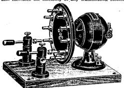
This Rotary Spark Gap emits a high musical note, more audible to the human ear, can be heard at greater distances than the note from the stationary type, and cannot be mistaken for static or other atmospheric disturbances, a fault common with the stationary gap due to its low frequency note.
