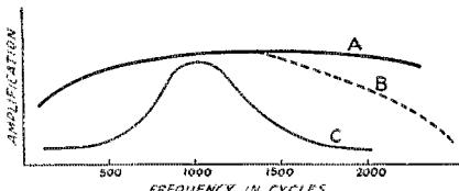
**FIG. 5. AUDIO AMPLIFYING TRANSFORMER CURVES**
