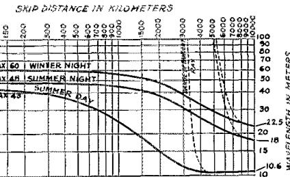
FIG. 12. CALCULATED SKIP DISTANCES BASED ON PRESENT EXPERIMENTAL VALUES
