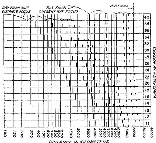
FIG. 11. ANOTHER GRAPHIC CHART TO SHOW PROBABLE PERFORMANCE OF DIFFERENT WAVES IN SUMMER DAYLIGHT AT VARIOUS DISTANCES
