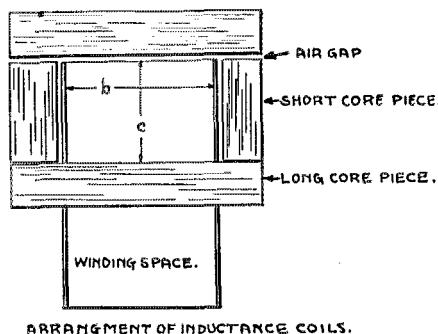
FIG. 8. ONE-HENRY IRON CORE CHOKE ON F. S. DELLENBAUGH'S DESIGNS
