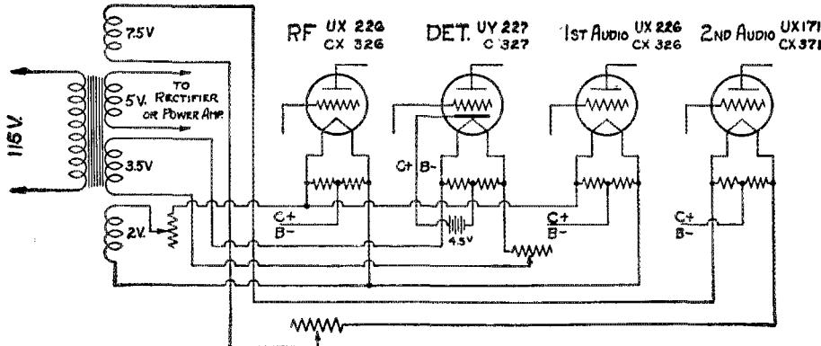
For the past several seasons the trend has been toward complete battery elimination. Many satisfactory plate supply units operating from A. C. have been developed but filament operation from an A. C. source has presented more of a problem due to the larger currents required and increased expense in the rectifier and filter circuits.
