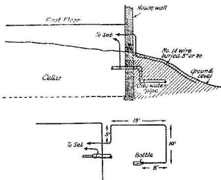
FIG. 3. THE ARRANGEMENT USED FOR RECEPTION AT 5VII, STATION OF CECIL PATTERSON AT FROST, TEXAS—WHERE THERE IS STATIC
