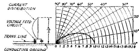
FIG. 15. AN ANTENNA SYSTEM THAT RADIATES MAINLY AT A LOW ANGLE
