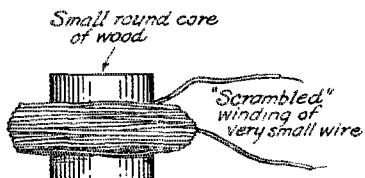
FIG. 10. CONSTRUCTION OF R.F. CHOKES USED IN THE VARIOUS CIRCUITS
