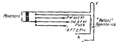
FIG. 4. FILAMENT CONTROL SWITCHES OF VARIOUS SORTS MAY BE CONNECTED AS SHOWN TO PUT OUT THE FILAMENT OF THE 3RD TUBE (2ND AUDIO STAGE) WHEN ONLY ONE STAGE IS WANTED
