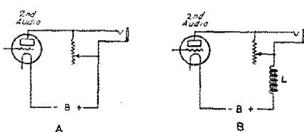
FIG. 2. OUTPUT CONTROLS
