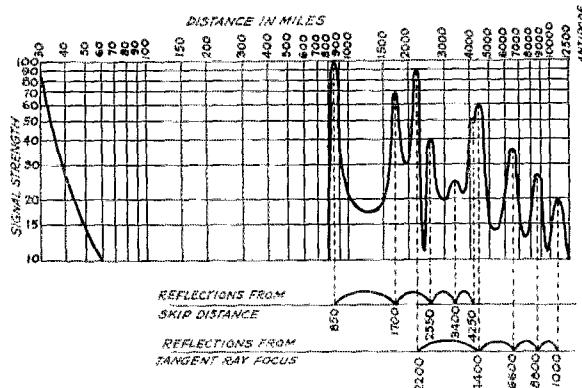
FIG. 10. CALCULATED SIGNAL STRENGTHS AT VARIOUS DISTANCES FROM A 20-METER TRANSMITTER ON A SUMMER DAY
