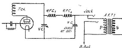
FIG. 9. AN ARRANGEMENT TO PERMIT CUTTING PHONES INTO THE DETECTOR PLATE CIRCUIT WITHOUT DETUNING THE INCOMING SIGNAL
