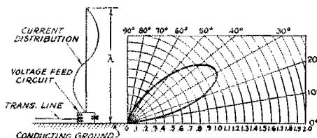
FIG. 16. AN ANTENNA GIVING MAINLY HIGH-ANGLE RADIATION
