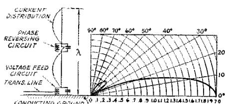
FIG. 17. A VERY LOW-ANGLE ANTENNA WHICH CAN READILY BE CONVERTED INTO THE FORM OF FIG. 16 BY SHORT-CIRCUITING THE PARALLEL-TUNED CIRCUIT AT THE CENTER
