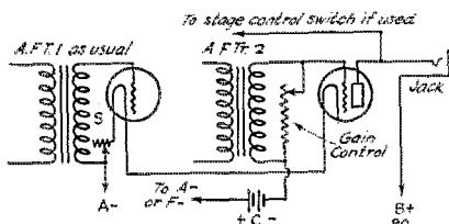
FIG. 3. HOW THE C-BATTERY SHOULD BE CONNECTED IF ONE WISHES TO USE A PLATE VOLTAGE IN EXCESS OF 60 ON THE 2ND AUDIO TUBE
