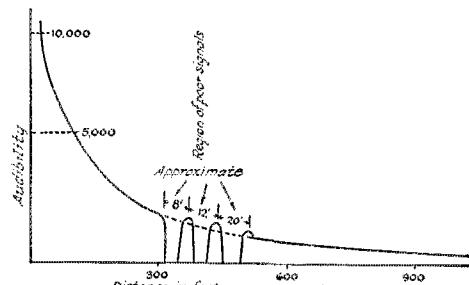
FIG. 5 CURVE SHOWING APPROXIMATE MANNER IN WHICH LOW-POWER  $\frac{3}{4}$ -METER SIGNAL VARIED IN AUDIBILITY WHEN RECEIVER WAS MOVED AWAY FROM STATION
