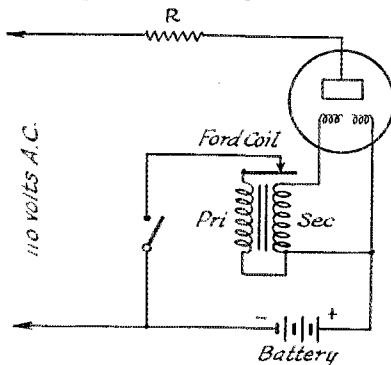
filament ends and the electrons emitted being attracted to the plate will start rectification. As the normal amount of current flowing from the plate to the filament is as large as the normal filament current, it is quite possible to let this current heat the filament. Therefore after the first spark has taken place, the tube will continue to operate even though no regular filament current is supplied.
