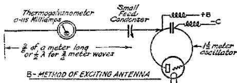
FIG. 2 THE SENDING ANTENNAS
