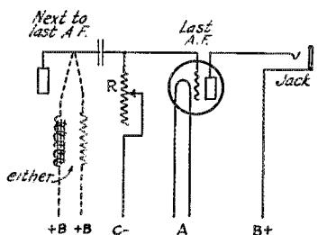
**FIG. 6. RESISTANCE AMPLIFICATION CONTROL APPLIED TO RESISTANCE-RESISTANCE OR IMPEDANCE RESISTANCE AMPLIFIER. IF ONE OF THESE IS TO BE USED**
