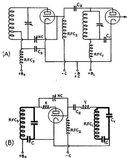
FIG. 2 — ANOTHER POSSIBLE LOW-FREQUENCY PARASITIC CIRCUIT
