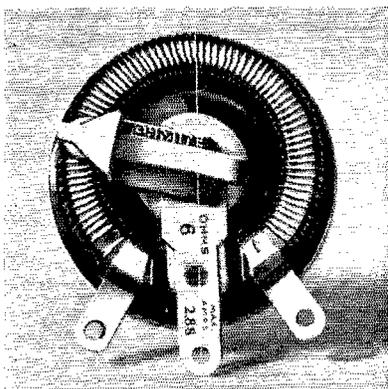
Ohmite rheostats were not selected by chance for use in W9USA but because they mark a real step forward in rheostat design. As the resistance wire is wound over a porcelain core and is covered with vitreous enamel, each turn is fused rigidly in place and is protected against both mechanical and electrical injury. The use of a metal-impregnated graphite contact insures low contact resistance and absolute freedom from arcing and sticking.
