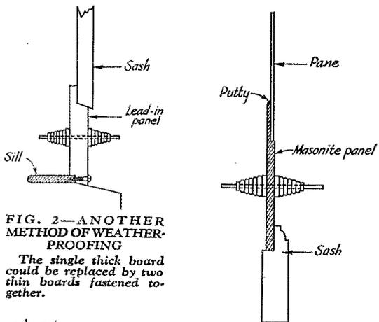
FIG. 2—ANOTHER METHOD OF WEATHER-PROOFING
