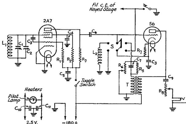
FIG. 1—COMBINED FREQUENCY METER, MONITOR, AUDIO OSCILLATOR
