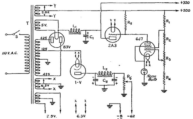
FIG. 3—REVISED POWER SUPPLY DIAGRAM, WITH BIAS SUPPLY INCLUDED
