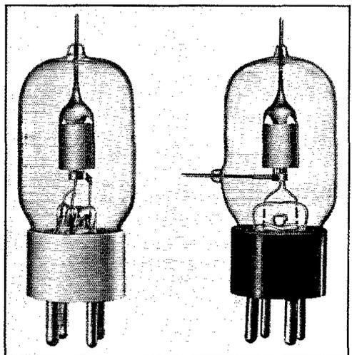
Two of the new Eimac tube types are, left, the 25T and, right, the 3C24. Data characteristics have been released on these tubes and are given in the text.
