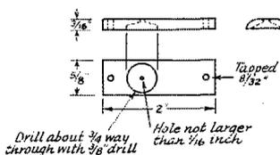
Fig. 3 — Details of sliding bar with light slit.
