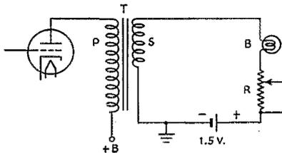
Fig. 1—Modulating circuit for light beam transmission. The resistor should be 6 ohms or larger.
