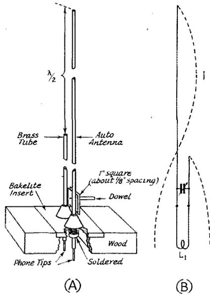
Fig. 3 — The plug-in antenna unit, complete with feed system. (A) Constructional details of vertical antenna and stub sections, trimmer tuning condenser, base, and insulators. (B) Schematic drawing of current distribution and tuning arrangement for the complete antenna system.
