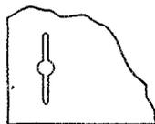
Fig. 4 — Slotted guide in the chassis for the bar, *C*, shown in Fig. 2. The hole in the center should fall directly over the window opening in the 930 tube.
