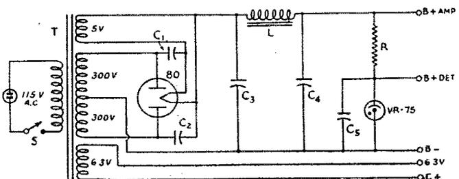
Fig. 2 — Power-supply wiring diagram and parts list.
