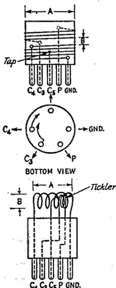
Fig. 3 — Arrangement of coil connections. The coil dimensions are given in the table at the top of the facing page.
