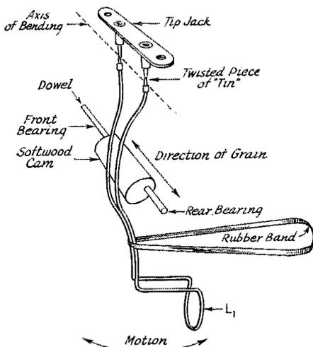
Fig. 2 — Constructional details of the antenna coupling coil.
