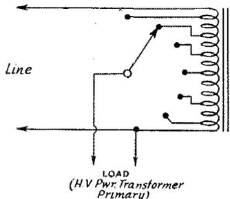
Fig. 4 — Circuit diagram of the autotransformer.
