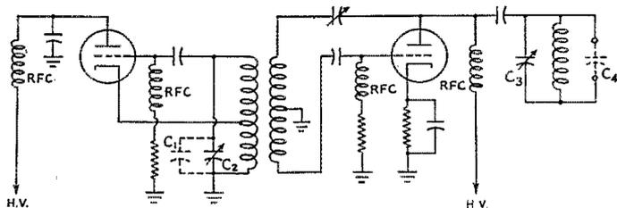
Fig. 1 — Diagram showing use of an m.o.p.a. transmitter in calibrating fixed condensers.
