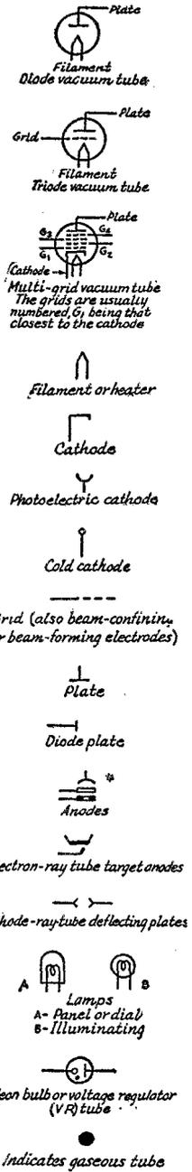
\* Alternative symbols marked with an asterisk are the conventional radio forms previously used. These are included for reference information in instances where the original symbol has undergone appreciable change under the ASA standardization program.
