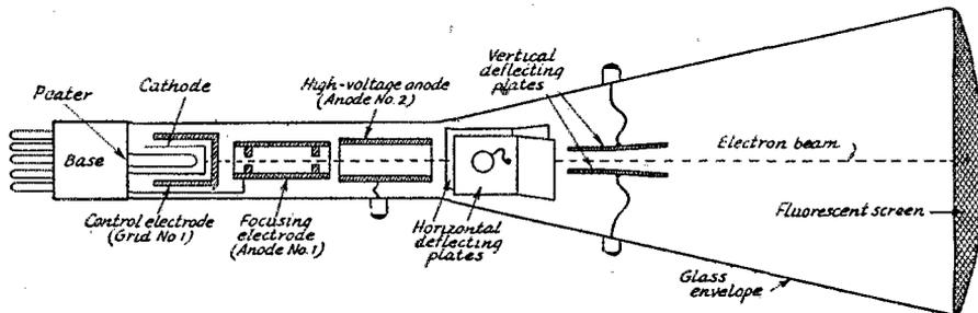
Fig. 1 — Sketch showing the construction of a typical cathode-ray tube of the electrostatic-deflection type. The envelope is usually made of glass, although at least one small type is made of metal except for the glass fluorescent screen at one end. Terminals for the high-voltage anode and for the deflectors are customarily mounted on the side of the envelope, while connections to other electrodes are made through the plug-in base.
