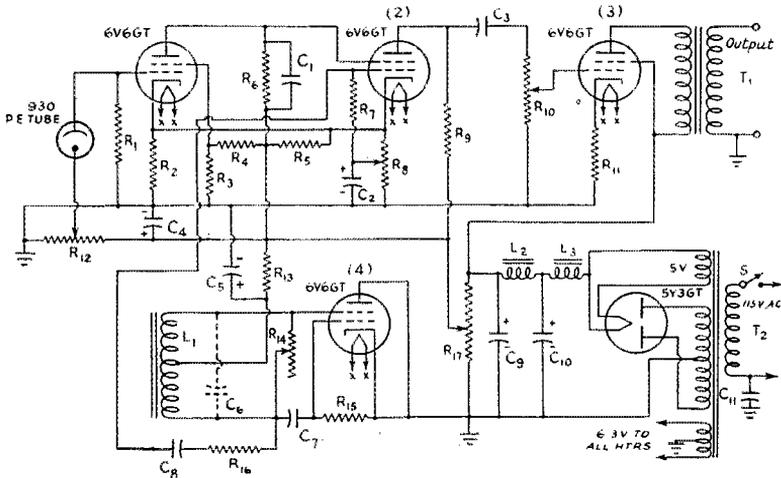
Fig. 1 — Circuit diagram of the electronic keyer.
