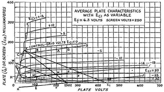
Fig. 3—Characteristic curves for 6L6. The point of origin, O, mentioned in the text is at the intersection of the vertical 250-volt line and the  $-14$ -volt bias line.
