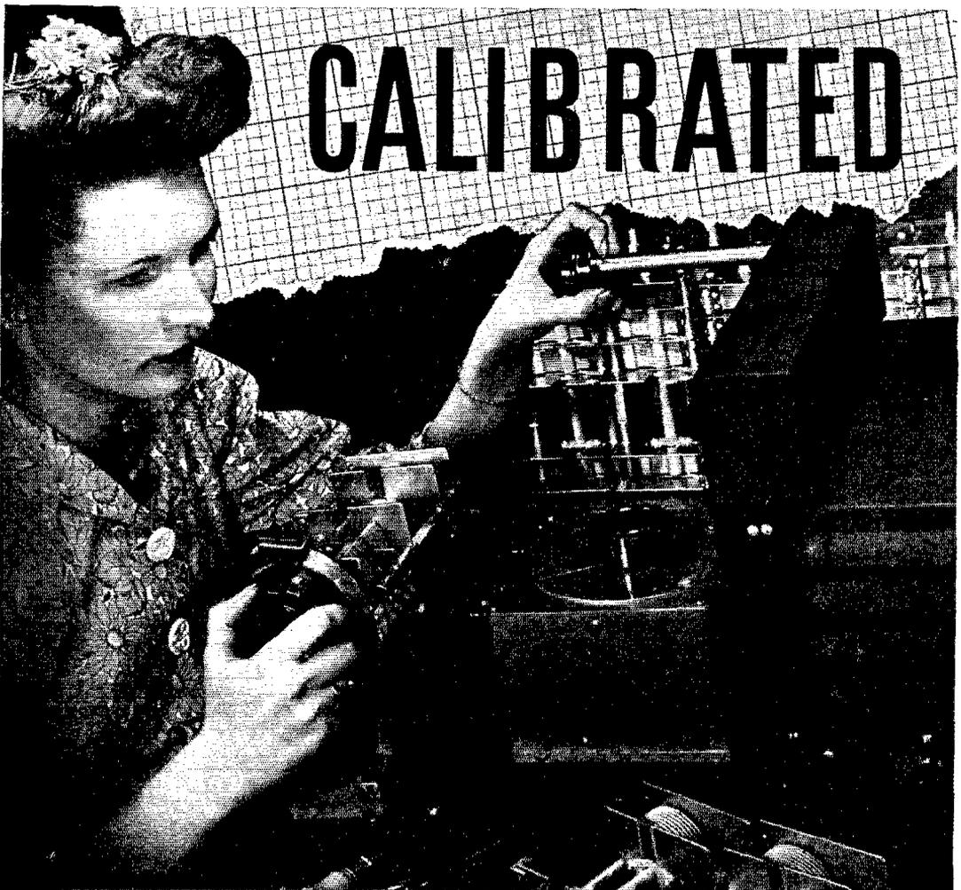
Through the development of our own highly specialized calibrating equipment Hammarlund engineers have made possible mass production of variable capacitors with accuracies comparable to laboratory standards.
