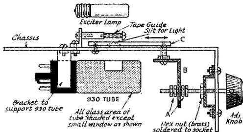
Fig. 2 — Photoelectric tube mounting and adjustable light slit. A — Dual hex nuts soldered to shaft to allow angle bracket "B" to slide freely as the adjustment knob is turned. B — Bracket bent as shown to transfer forward or backward motion of bar, C. C — Sliding bar with light slit drilled in. (See Fig. 3 for details.)
