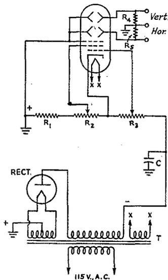
Fig. 3 — Circuit diagram showing power-supply connections to cathode-ray electrodes.
