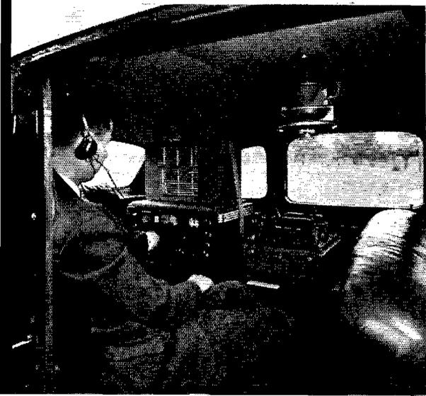
*Right*— Operating position in the intercept room where signals are recorded on tape, on wax cylinders or on disc recorders. The receiver at the extreme right is the diversity version described in the text. Note the selector switches for the rhombics. Feeders from the rhombic antennas may be seen at the top center where they enter the room.
