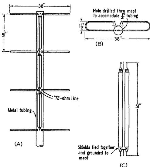
Fig. 1 — The City Slicker array for 144 Mc. described by W8UKS consists of 4 folded dipoles stacked  $\frac{5}{8}$  wavelength apart, as shown at A. Details of the individual dipoles are given in B. The phasing sections, C, are electrically one wavelength long. Their outer conductors are connected together and bonded to the mast. Feed-point impedance is 72 ohms, but any type of line may be used with a suitable matching transformer.
