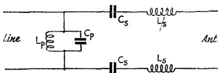
Fig. 7—Two-band network suitable when the line impedance is greater than the driving-point impedances.
