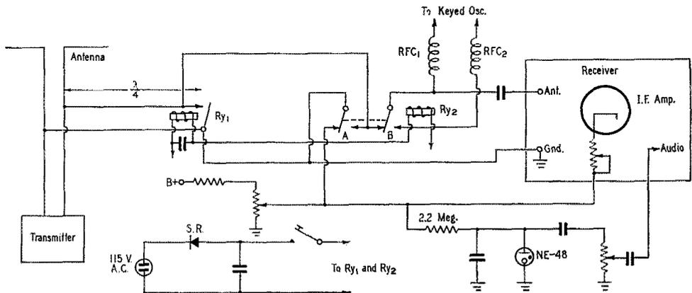
Fig. 4 — A mechanical version of the break-in system, requiring two relays. The s.p.s.t. relay *Ry*<sub>1</sub> "holds in" longer than *Ry*<sub>2</sub> because a large condenser (value depending upon coil resistance of *Ry*<sub>1</sub>) is connected across the coil. This circuit uses oscillator keying in the transmitter and a small audio oscillator of the "Monitone" variety for a keyed sidetone. W2SO uses small surplus relays (Clare Type K, 300-ohm coil) and a selenium-rectifier supply.
