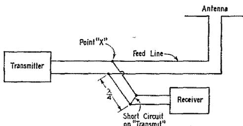
Fig. 1 — This arrangement will permit use of the same antenna for transmitting and receiving if the quarter-wavelength stub is shorted during "transmit" periods. It will be recognized as the "T-R" circuit used in radar systems.
