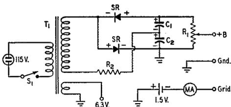
Fig. 2 — Power supply and meter circuit.
