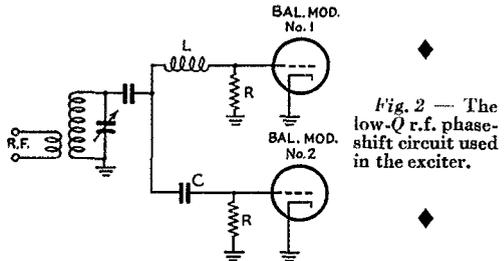
Fig. 2 — The low-Q r.f. phase-shift circuit used in the exciter.
