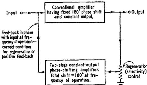
Fig. 5 — Block diagram of selective amplifier and oscillator connection.
