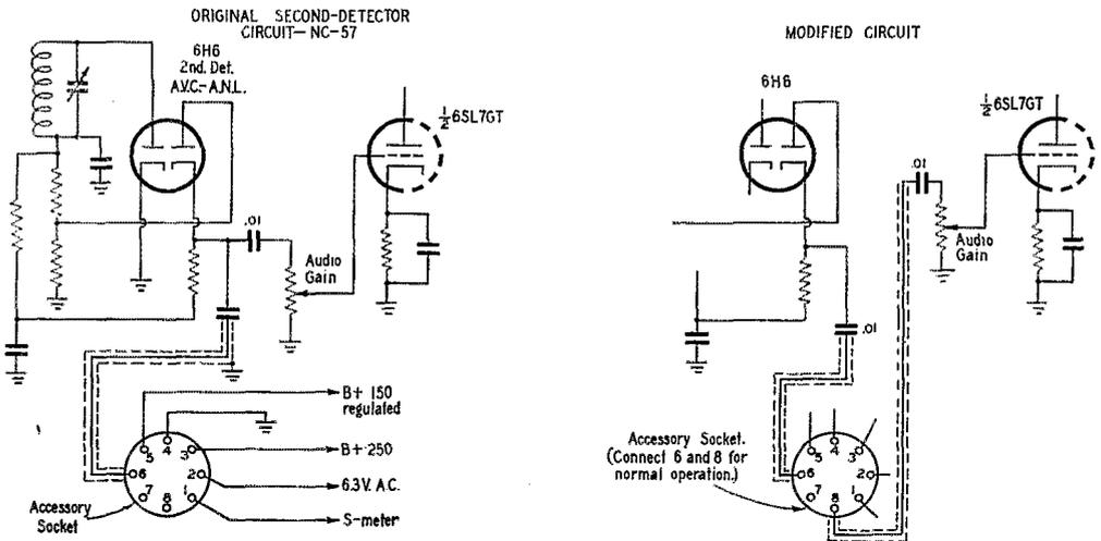
Fig. 8 — These circuit modifications to the NC-57 receiver to use the Selectoject are typical of the method of connection to the average communications receiver. The essential modification is to open an audio lead and insert the Selectoject.
