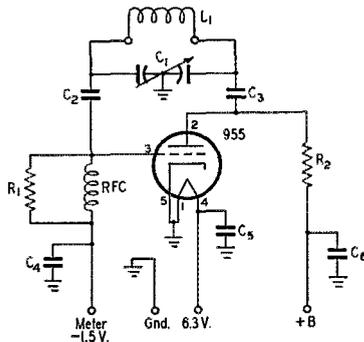
Fig. 1—Regenerative wavemeter circuit.
