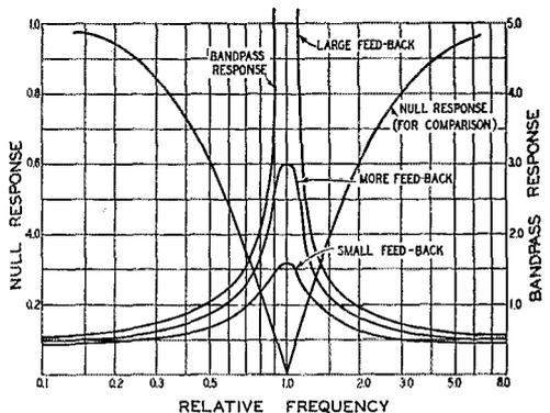
Fig. 6 — Frequency response of selective amplifier, for different degrees of selectivity.
