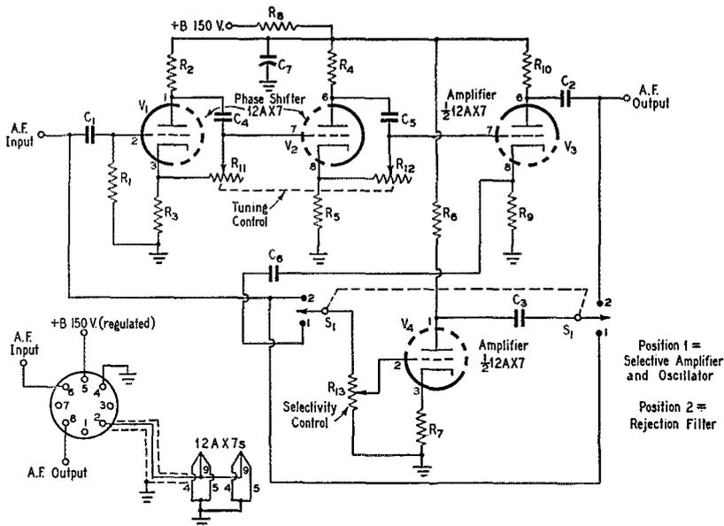
Fig. 7 — Complete schematic of Selectoject using 12AX7 tubes.
