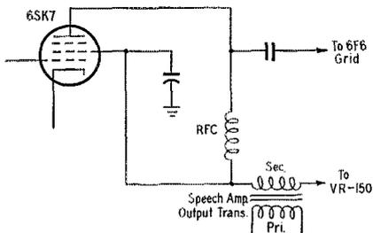
Fig. 1 — Simple method of obtaining an n.f.m. signal for 75-meter 'phone-band operation. The plate and screen of a high-C VFO are amplitude-modulated as shown. The diagram is adapted from that of the VFO described in *QST* for September, 1946.
