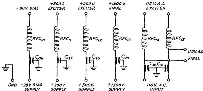
Fig. 2 — Wiring diagram of the harmonic-filter unit for the 500-watt all-band transmitter.
