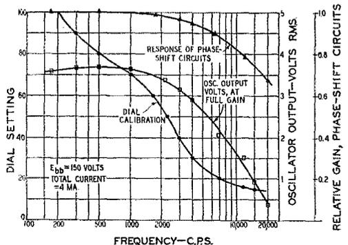
Fig. 9 — Measured performance of model using 12AX7 tubes.
