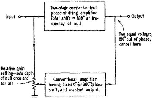
Fig. 2 --- Block diagram of rejection-filter connection.
