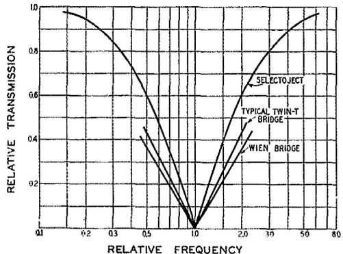
Fig. 4 — Frequency response of rejection filter compared with Wien and twin-“T” bridges,
