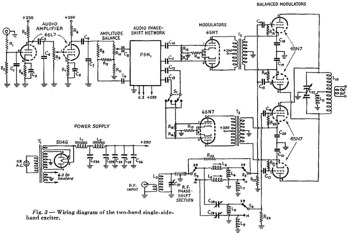
Fig. 3 — Wiring diagram of the two-band single-side-band exciter.
