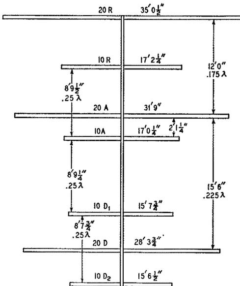
Fig. 1 — "Super-Interlaced Beam" dimensions.
