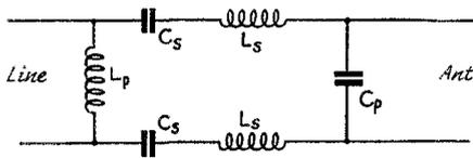
Fig. 6—Two-band network suitable when the line impedance is between the two values of driving-point impedance, the larger of which is at the higher operating frequency.
