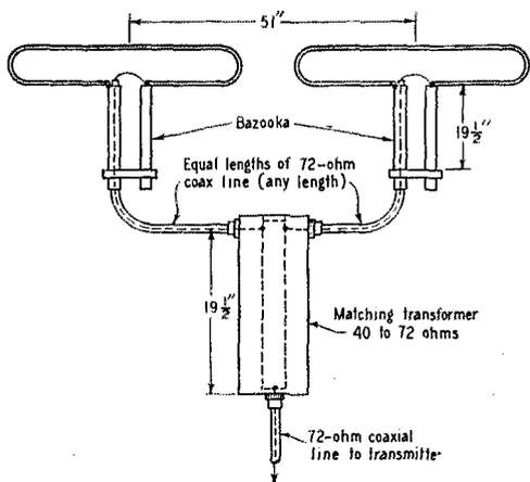
Fig. 2 — Two or more sets of dipoles may be placed side to side and fed in phase, for increased gain and directivity. A bazooka, or line balancer, is connected at the feed dipole in each set, and these are connected to the inner conductor of a coaxial matching transformer. The system may then be fed with 72-ohm coaxial line, as shown. The coaxial transformer may be built to dimensions obtained from Fig. 10-15 of the 1949 ARRL Handbook.
