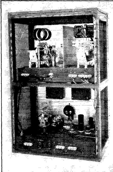
Rear view of the transmitter enclosure with the back screen panel removed. A shielding partition separates the final amplifier and the antenna tuner. Standard 2 x 4 x 4-inch steel boxes cover the final-amplifier meters. The harmonic-filter enclosure at the bottom is fastened permanently to the frame so that the power plugs on the back of the exciter chassis make connection when it is pushed into place from the front.
