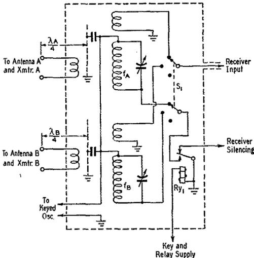
Fig. 3 — For operation on several bands, with separate antennas and transmitters for each band, the circuit of Fig. 2 can be modified to include separate tuners for each band. The 2-pole switch makes band-changing a simple matter. The circuit is shown here for oscillator keying.
