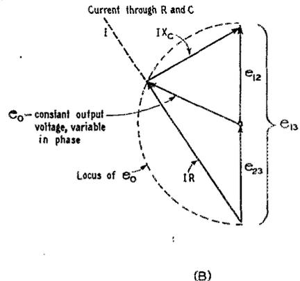
therefore remains constant in strength as its phase position is varied. Instead of a transformer, in the circuit of Fig. 1A, it is more convenient to use a phase-inverter tube.
