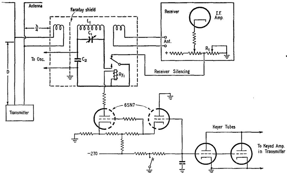
Fig. 2 — A practical amateur application of the "T-R" system. The short circuit is obtained with relay  $Ry_1$ , and the job is made easier by the step-up in impedance.  $L_1C_1$  tunes to the frequency in use,  $C_2$  is a 0.001- $\mu$ fd. mica receiving-type condenser. Constants associated with the 6SN7, keyer tubes and receiver can be found in the reference under footnote 1 or on page 255 of the 1949 edition of *The Radio Amateur's Handbook*.
