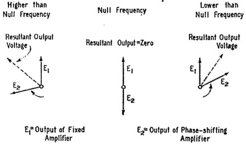
Fig. 3 — How the null is achieved, for a given setting of the tuning control.
