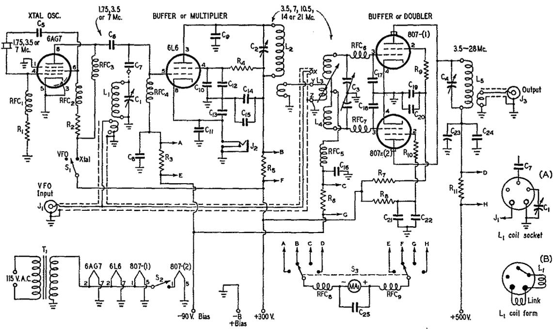
Fig. 1 — Circuit diagram of the exciter for the 500-watt all-band transmitter.
