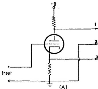
Fig. 1 — A — Basic phase-shifting circuit. B — Vector diagram of basic phase-shifting circuit.
