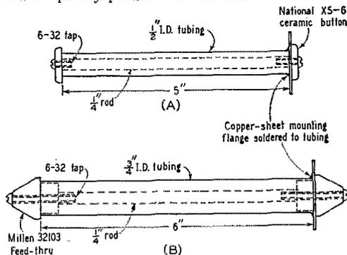
Fig. 4 — Sketches showing method of constructing the tubular air condensers. A for the 807 plate by-pass condenser and B for the plate-to-ground condensers in the final amplifier. The outer tubing and the inner rod may be of aluminum or copper.
