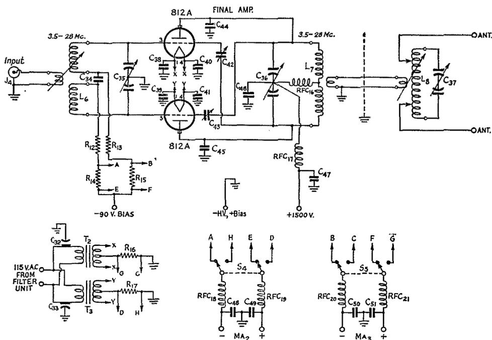
Fig. 3 — Circuit diagram of the final amplifier and antenna tuner of the 500-watt all-band transmitter.
