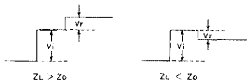
Fig. 6 — TDR displays for SWR measurement, where Z_L is purely resistive.
