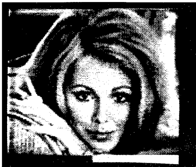
is one means of smoothing out the effects of contouring, as shown here. At the left is a 128 by 128 picture-element slow-scan picture with 16 brightness levels. At the right is the same picture except for the addition of pseudo-random noise.
