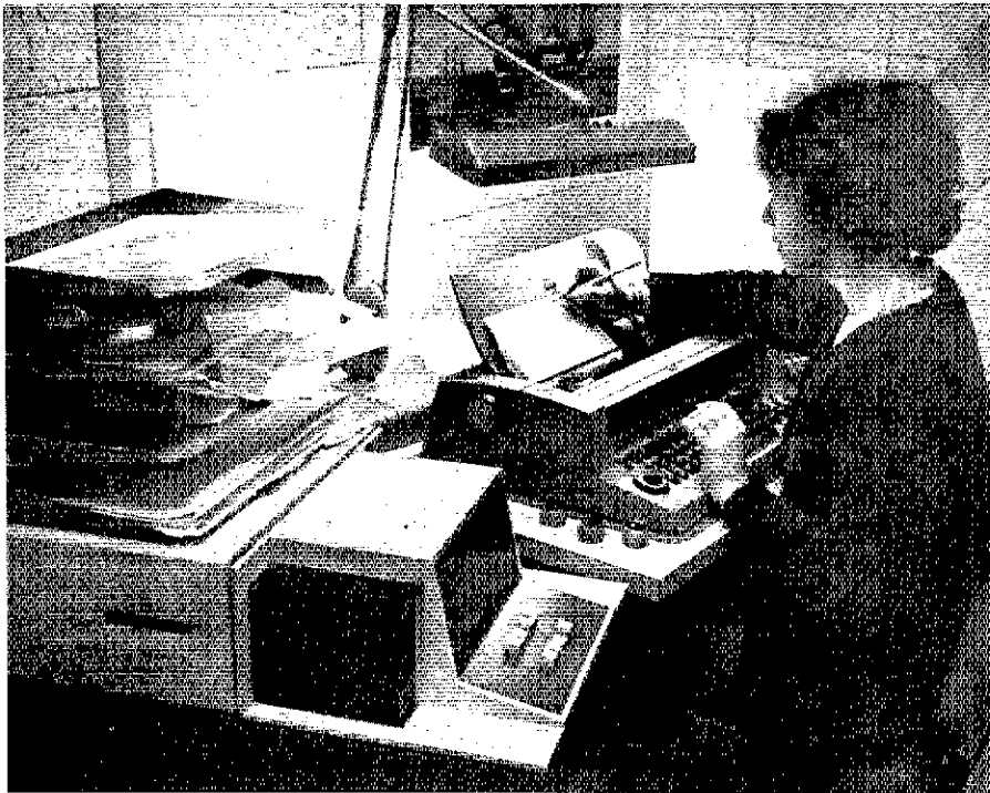
xjm189.i5.t was not long ago, that some mysterious signals . . . that's the first line of Lee's edited manuscript as a typist recorded it in coded form on magnetic tape in the IBM composing system. Here the coded instructions are being used to print out the information in QST type at a speed of 150 wpm!
