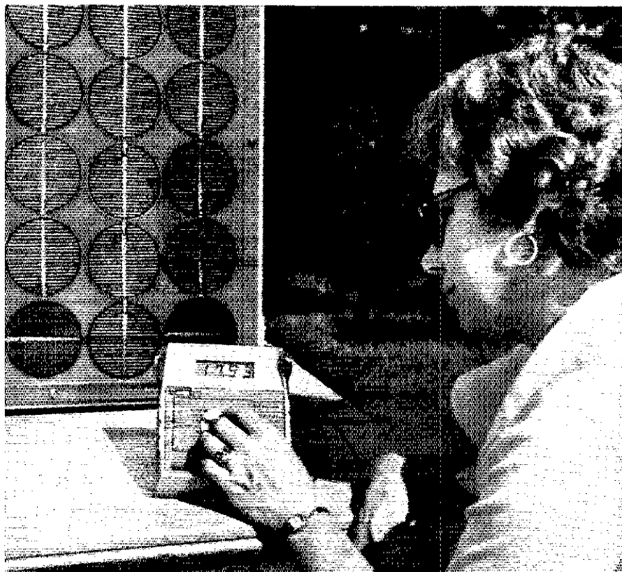
Fig. 7 — W1CCKK of the ARRL hq. staff checks the no-load output voltage of the commercial solar panel during a period of bright sunlight. A reading of 17.93 volts was obtained (battery disconnected).
