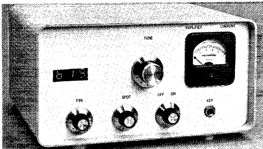
The medium-power solid-state cw/RTTY transmitter puts out about 35 watts into a 50-ohm load. An antenna tuner should be used for best results if the SWR is different from 1:1, since the output tuning is fixed. The indicated frequency is 3.619 MHz. The control labeled "FSK" is for adjustment of the RTTY shift.
