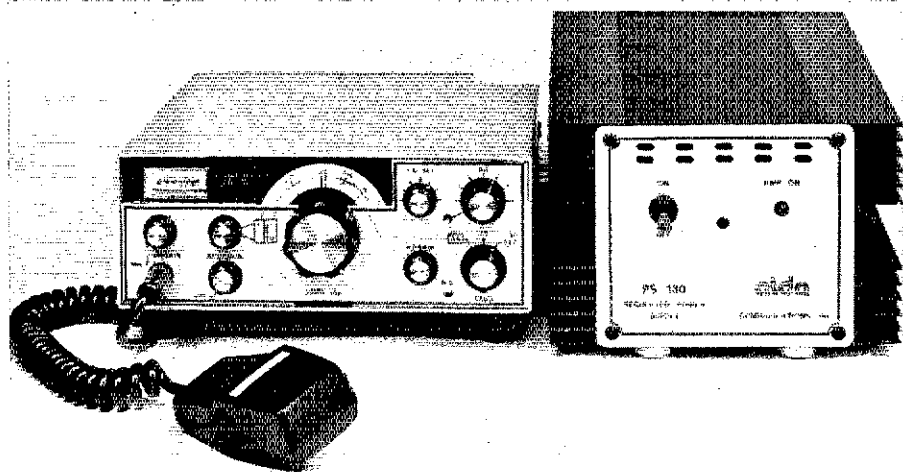
The Alda 103 and its optional 30-A supply, the PS-130. The dial on the '103 is available in Braille for the blind ham.
