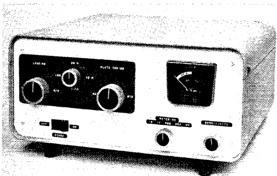
Front view of the modified SB-200 linear amplifier. A small false panel covers the original panel holes and adds a contrasting green color to the white front panel. Green Dymo tape labels identify the control functions.
