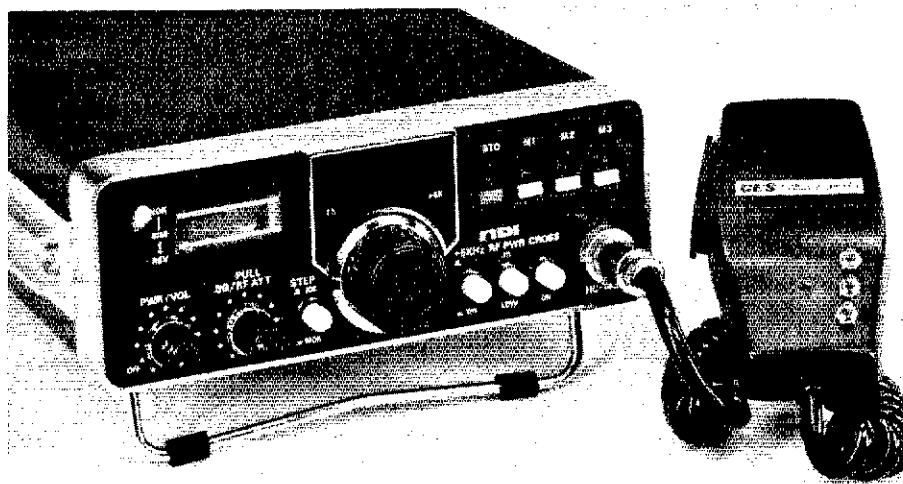
The NDI '1400 is shown here with the optional RM1400TT microphone. The frequency-changing buttons can be seen at the right-hand side of the microphone. The tactile Touch-Tone pad is on the rear of the microphone and not visible in this photograph.
