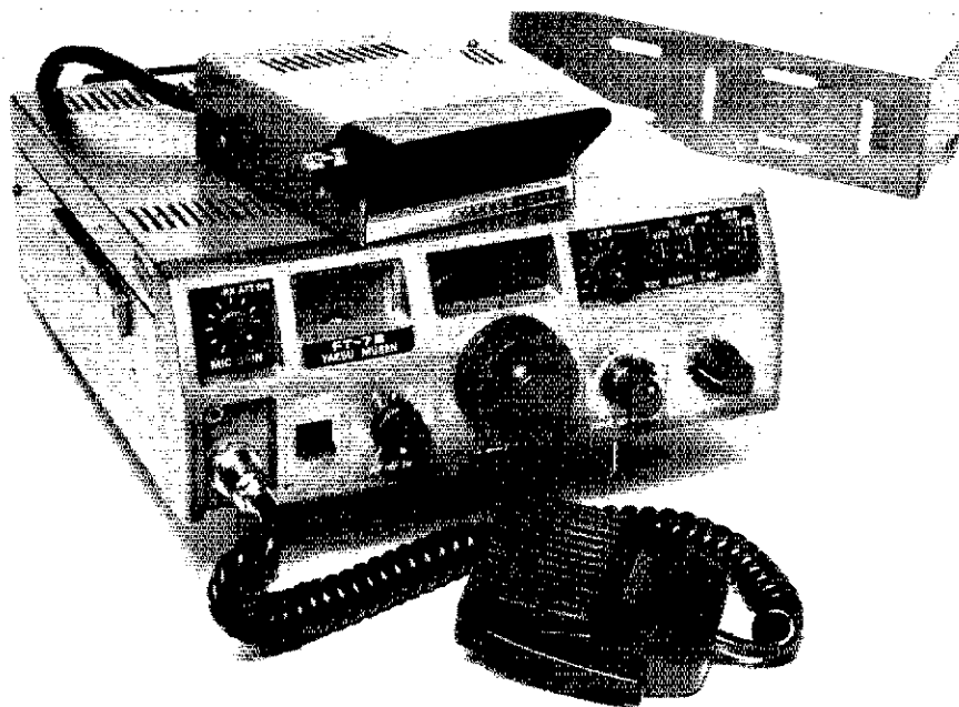
The FT-7B transceiver with optional YC-7 remote frequency display. The microphone and mobile mounting bracket are supplied with the transceiver.
