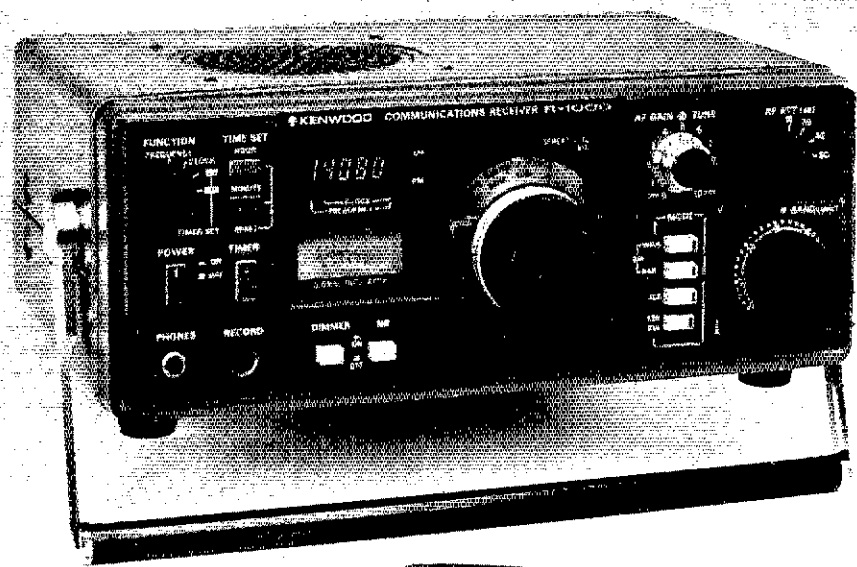
Fig. 1 — Kenwood's R-1000 is a compact performer: The carrying handle also serves as a support if additional table clearance is desired.
