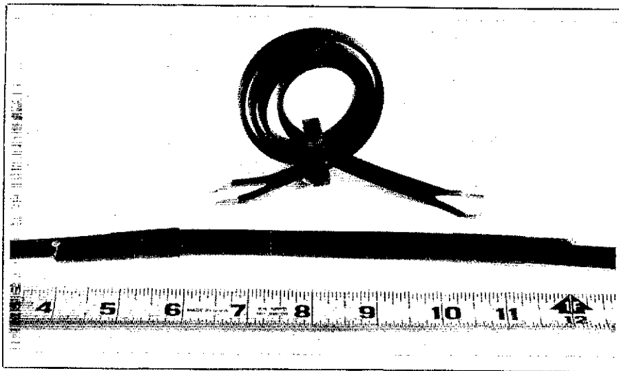
Fig. 4 — Common-mode chokes. At the top, several turns of twin-lead are taken through an FT-114-43 ferrite toroid; best results will be obtained if the twin-lead has an oval cross section. At the bottom, the twin-lead has been cut near the TV set. The conductors have been shorted at the resulting ends and the ends have been overlapped approximately 9 inches. Shrinkable tubing or tape is used to hold the two pieces together.
