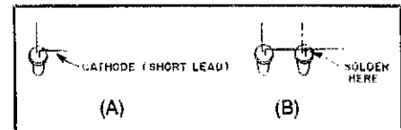
Fig. 10 — (A) The minutes and seconds LED cathodes are bent in this shape prior to mounting. (B) Each cathode of a 10-LED group is soldered as illustrated.
