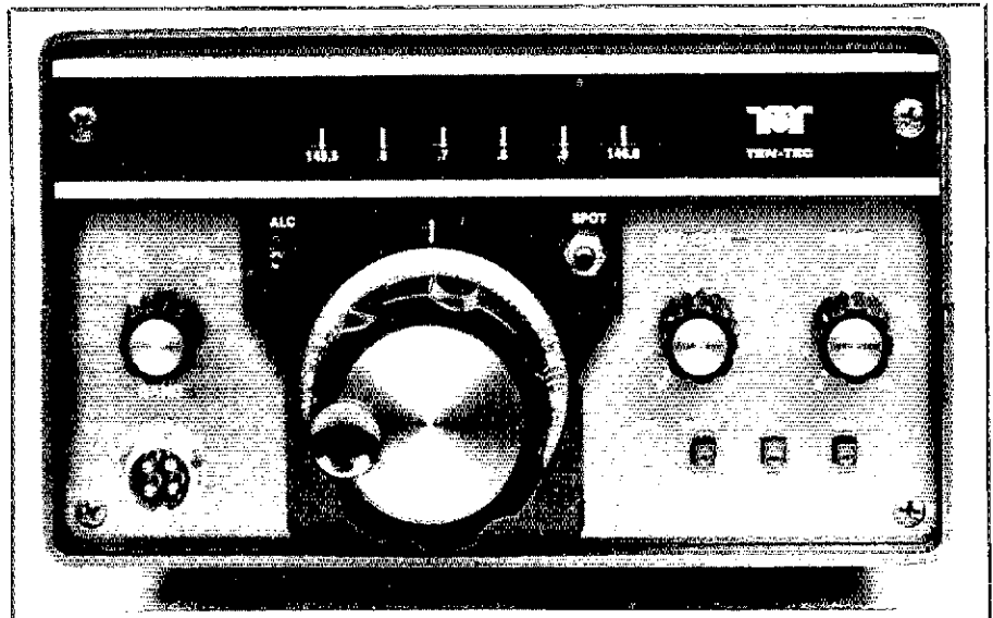
The Ten-Tec 2510 Mode-B satellite station is designed specifically for Mode-B operation. The box contains a 435-MHz SSB and CW transmitter, as well as a 145- to 28-MHz receiving converter with a low-noise front end.
