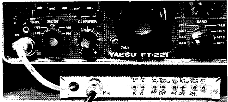
Fig 14—The station control unit at WD4FAB fits underneath a transceiver. It houses the TR sequencer and provides instant control of many station functions.
