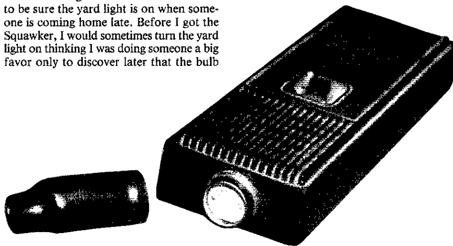
Fig 1—The Squawker. A salvaged cassette recorder microphone case is used as the enclosure. The photocell is the cylindrical light-colored object in the foreground. To the left of the Squawker is a piece of heat-shrink tubing used as a light shield when examining LEDs (see text).
