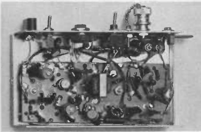
Interior of the ultra-portable transceiver. Double-sided board is used in this equipment.
