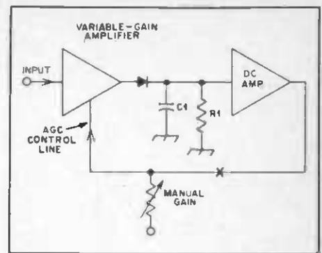
Fig. 50 — Circuit representation of a total agc loop.
