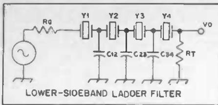
Fig. 37 — Details of a 4-pole lower-sideband ladder filter.
