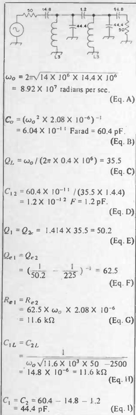
Fig. 6 — Design of a filter using the method of Fig. 5. The filter is terminated in 50 ohms at each end and has a bandpass of 14 to 14.4 MHz.
