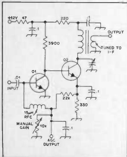
Fig. 42 — A dual-gate MOSFET i-f amplifier.
