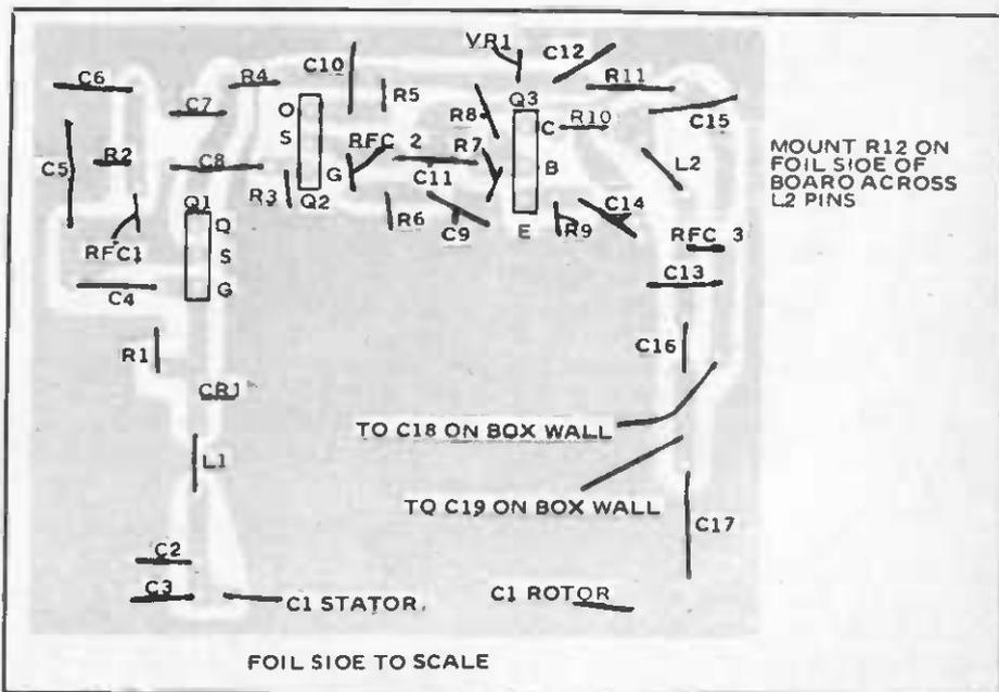
Fig. 9 — Scale layout of the VFO circuit board.
