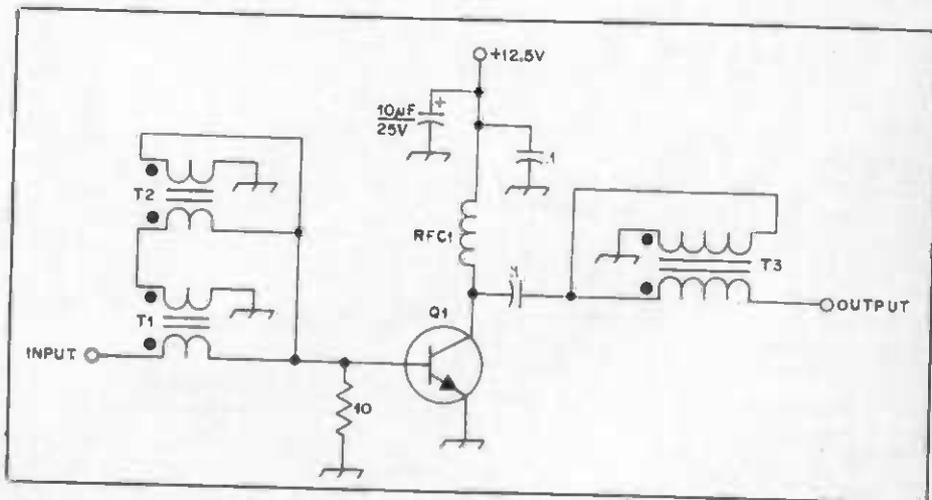
Fig. 33 — Single-ended 4- to 6-W amplifier. RFC1 is a 25- $\mu$ H choke capable of passing 1 ampere. See text for discussion of Q1. T1, T2 and T3 contain 7 bifilar turns of two twisted pairs of No. 26 enamel wire on Amidon FT-37-61 toroid cores.
