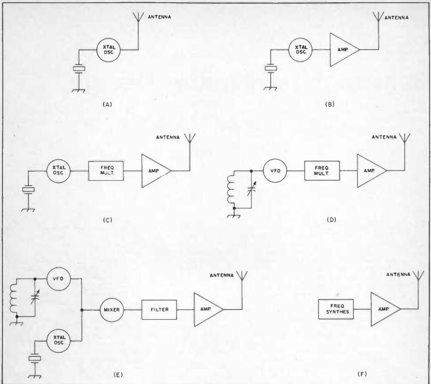
Fig. 1 — Block diagrams of various cw-transmitter formats.
