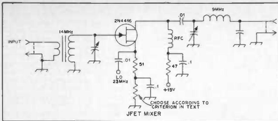
Fig. 14 - Circuit of a JFET mixer.
