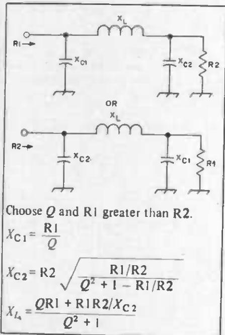
Fig. 4 — Pi-network configuration with design equations.
