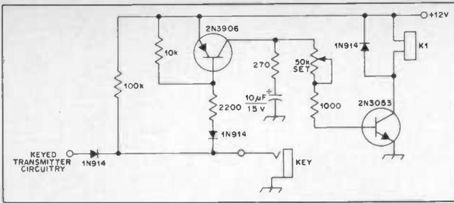
Fig. 80 - A relay-driver circuit for T-R applications.
