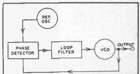
Fig. 32 — Illustration of a basic PLL circuit.
