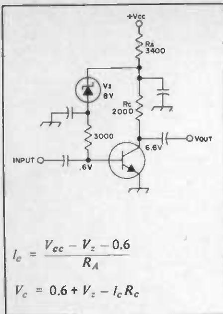
Fig. 12 — Amplifier bias using the Zener diode.
