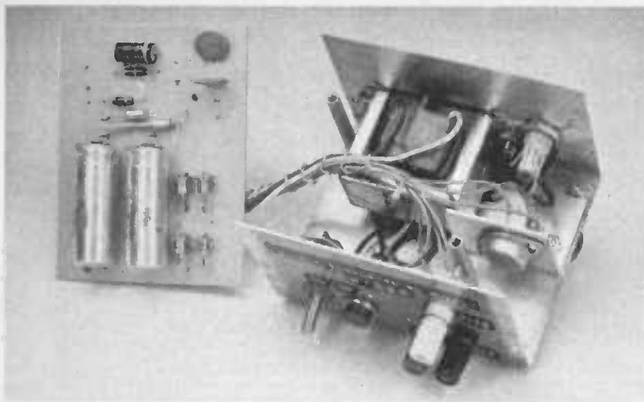
Inside layout of the 500-mA supply. The pass transistor is seen on an L-shaped homemade heat sink.
