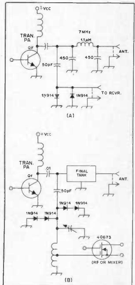
Fig. 90 — Circuit of a simple T-R switch.
