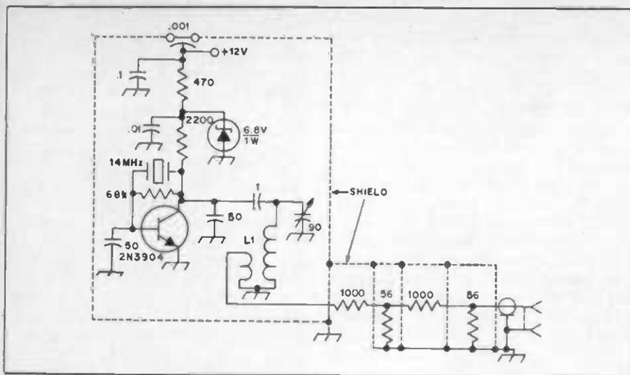
Fig. 65 — Circuit of the weak-signal 14-MHz generator. L1 has 24 turns of No. 26 enam. wire on an Amidon T50-6 toroid core. The link consists of a single turn of wire.
