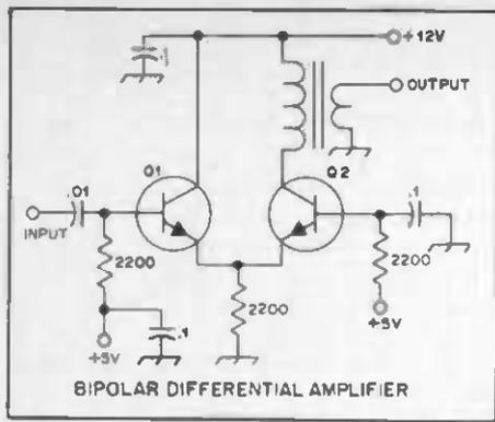
Fig. 43 — A differential pair i-f amplifier.
