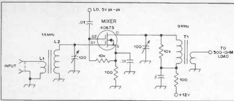
Fig. 58 — Circuit for a dual-gate MOSFET mixer.
