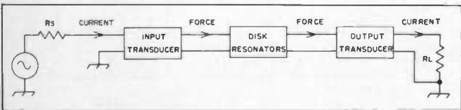
Fig. 29 — Illustration of how a mechanical filter operates.
