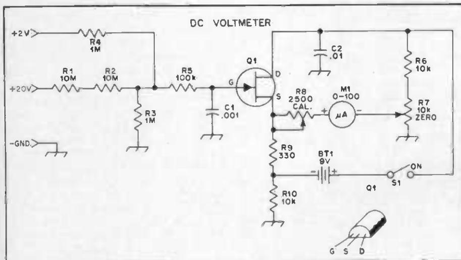
Fig. 1 — Circuit for the FET voltmeter. Fixed-value resistors are 1/4- or 1/2-W composition. C1 and C2 are disk ceramic. M1 is a 100- $\mu$ A dc meter. Q1 is a Motorola MPF102 or HEP802. R7 and R8 are pc-board-mount composition controls.
