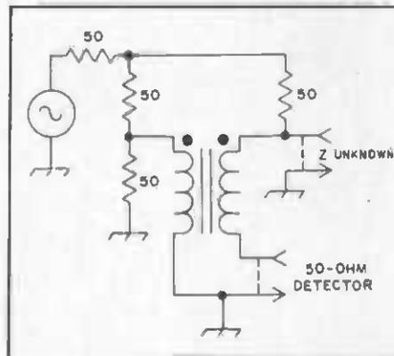
Fig. 36 — A return-loss bridge for impedance measurements. See text.
