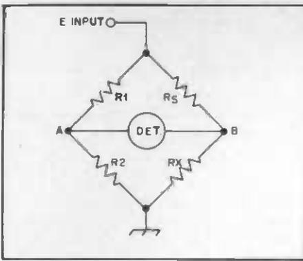
Fig. 24 - A Wheatstone bridge for measuring dc resistance.
