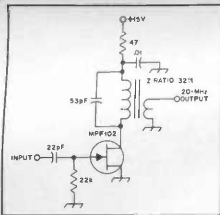
Fig. 18 — Circuit of an FET frequency multiplier.
