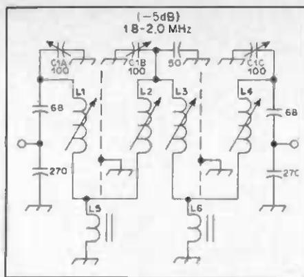
Fig. 8 — Tunable Cohn type of filter for 1.8 MHz. L5 and L6 are 1.45- $\mu$ H bottom-coupling toroidal inductors.
