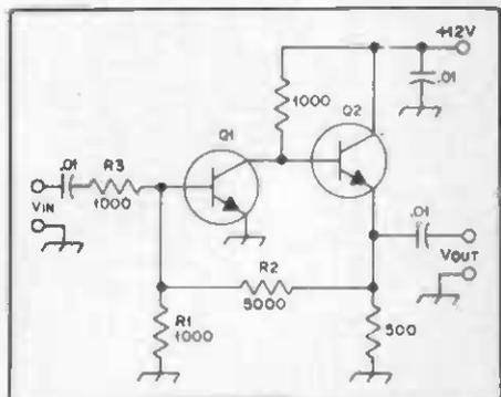
Fig. 10 — Rf buffer using shunt feedback.
