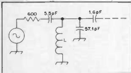
Fig. 4 — Input portion of a filter from Table 3.
