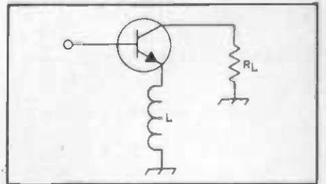
Fig. 6 — Amplifier with an inductive-emitter termination. This method is often used with microwave amplifiers to achieve a proper input impedance match while preserving amplifier-noise figure and stability.
