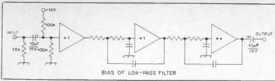
Fig. 20 — Biasing of cascaded filter sections is simple, as shown here.
