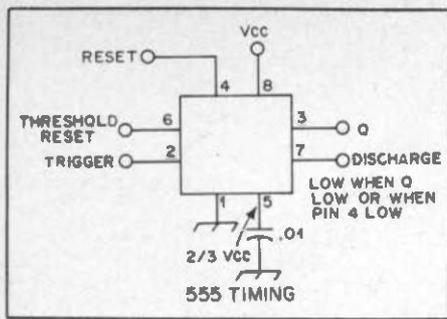
Fig. 86 — Block presentation of an NE555 timer IC.
