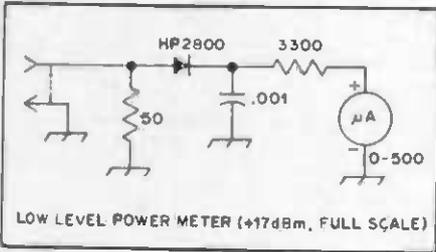
this kind are easily calibrated by noting that the circuit is still a peak-reading detector. This allows a dc calibration to be done.
