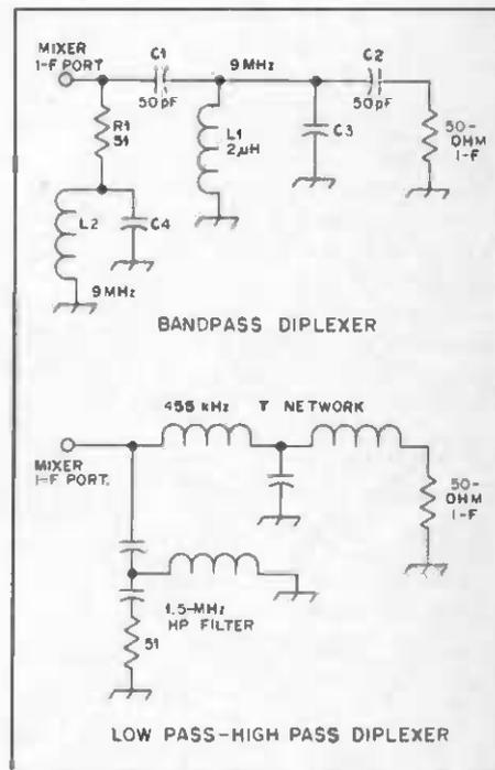
Fig. 11 — Diplexer circuits for use after a mixer.
