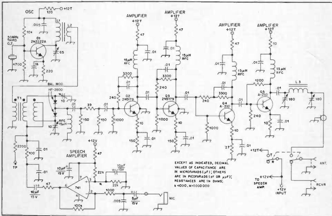
Fig. 29 — Circuit for a 6-Meter dsb QRP transmitter (see text). T-R switching is realized with a double-pole, double-throw slide switch.
