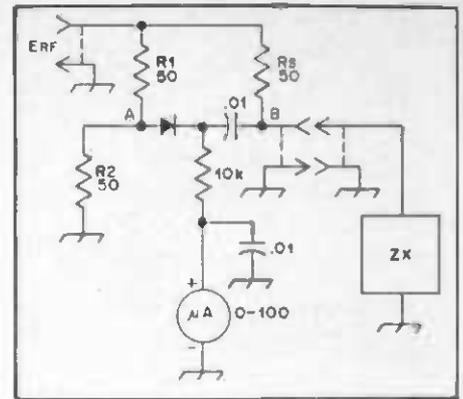
Fig. 26 - A bridge circuit for rf sine waves.
