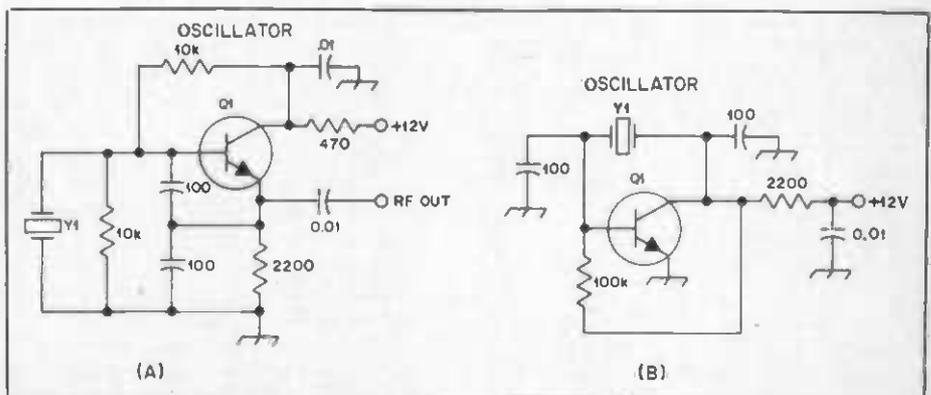
Fig. 6 - Crystal oscillators which use no tuned circuits.
