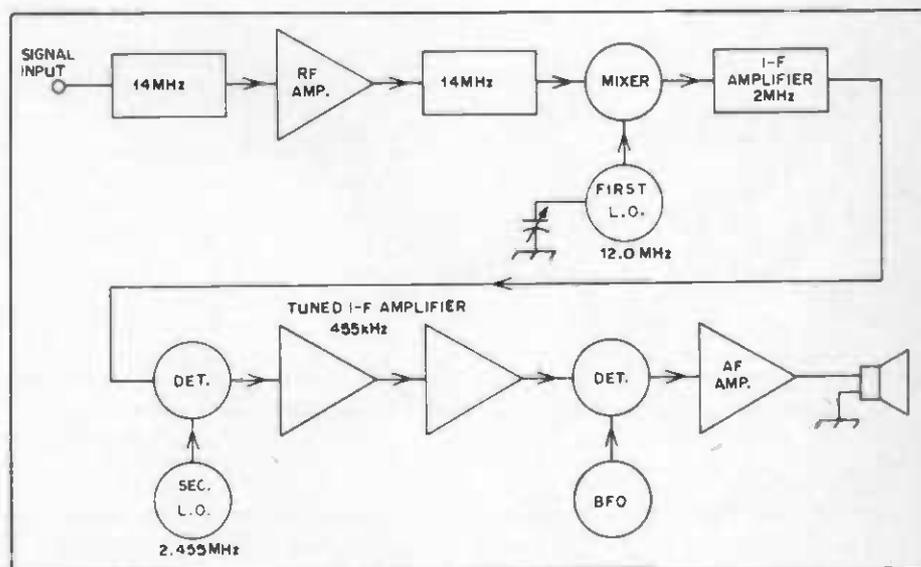
Fig. 26 — Representation of a dual-conversion superheterodyne receiver.
