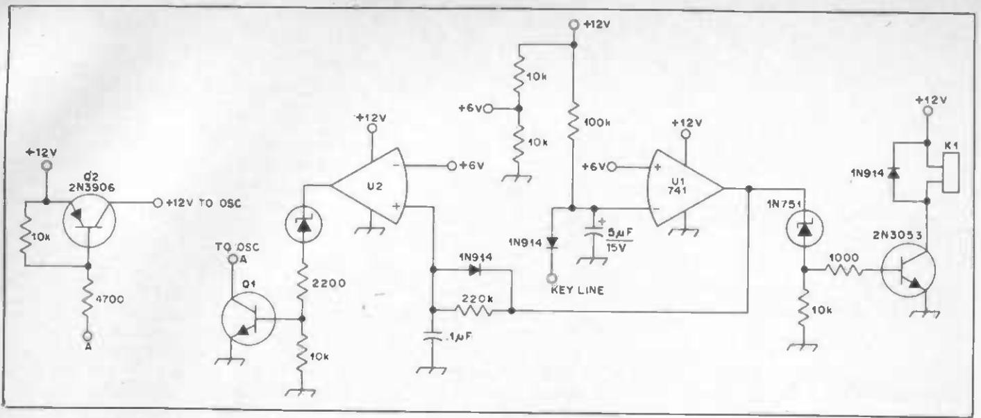
Fig. 83 — Recommended T/R circuit (see text explanation).
