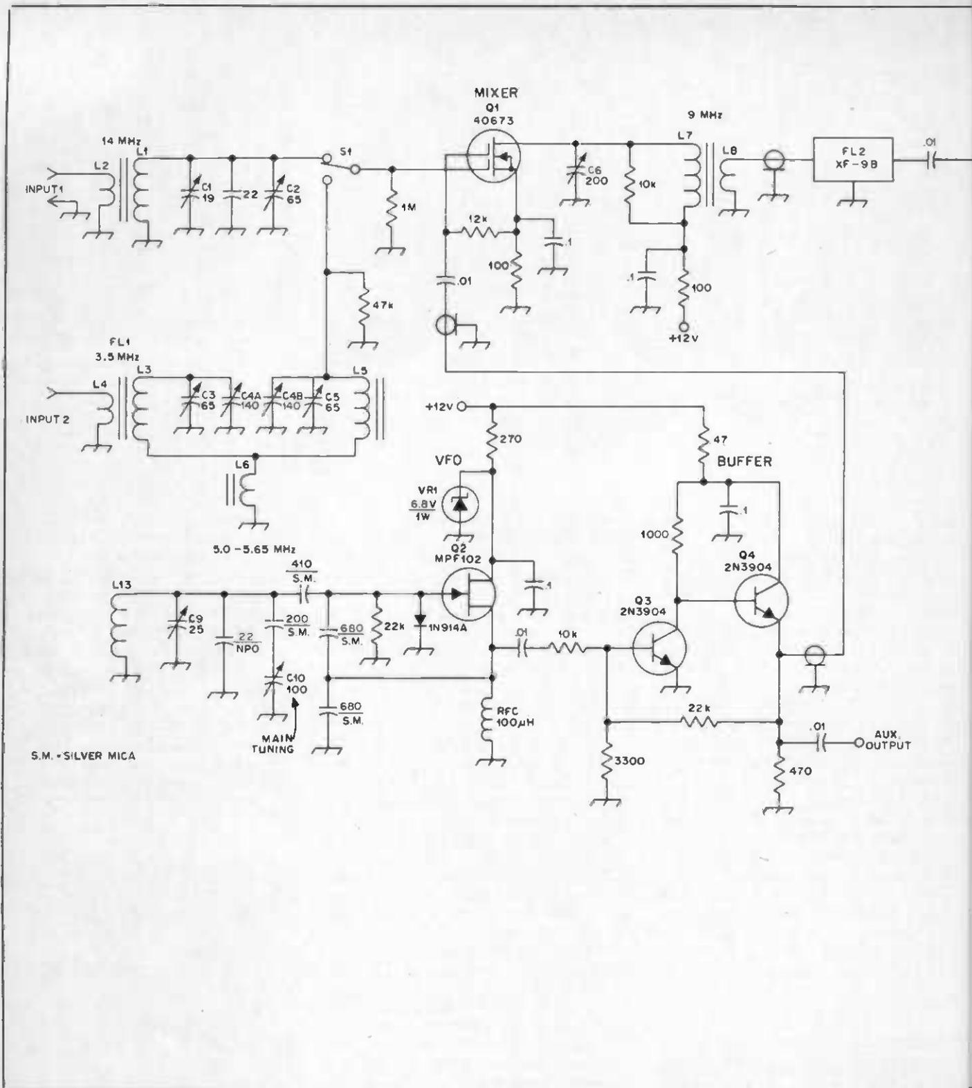
Fig. 74 — Schematic diagram of the 20- and 80-meter superheterodyne receiver. Fixed-value capacitors are disk ceramic unless noted. Fixed-value resistors are 1/2-Watt composition. Polarized capacitors are electrolytic. Numbered capacitors not listed below are trimmers.
