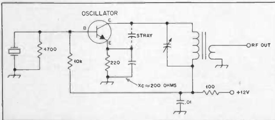
Fig. 3 — Circuit for a bipolar-transistor crystal oscillator.
