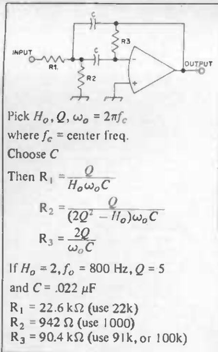
Fig. 23 — Band-pass filter with suitable design equations.
