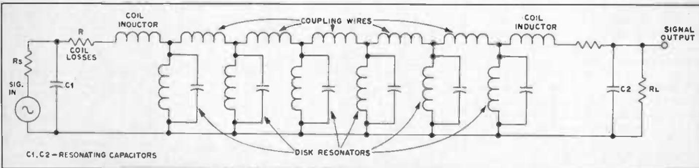
Fig. 30 — Analogous representation of a mechanical filter.
