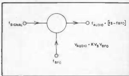
Fig. 3 — Representation of a product detector.
