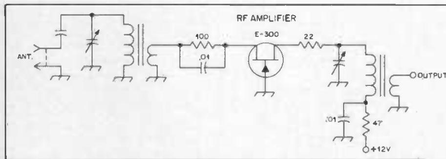
Fig. 65 — Circuit of a common-gate JFET rf amplifier.
