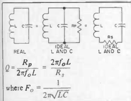
Fig. 4 - Modelling of an ideal resonator with series or parallel resistance.
