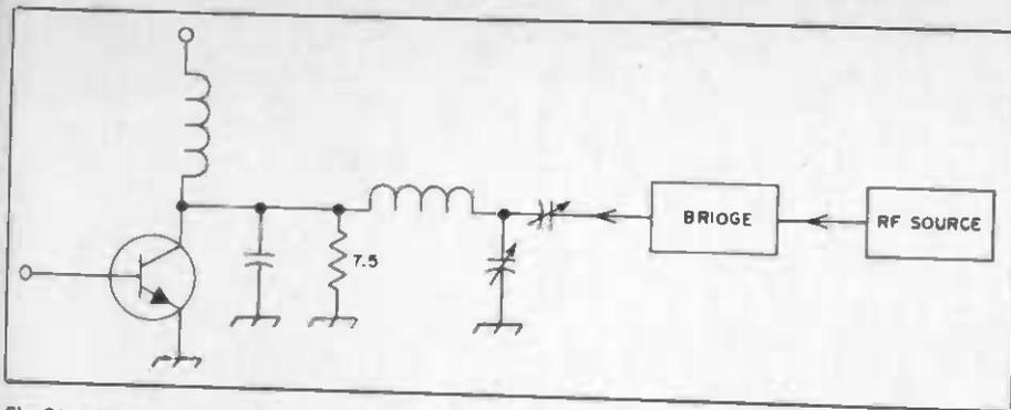
Fig. 31 — Method for prealigning an output network.
