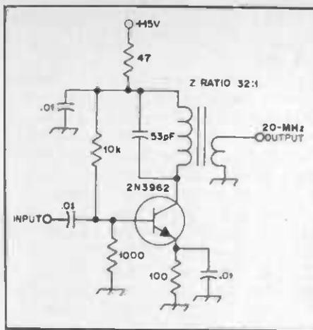
Fig. 15 — Diagram of a bipolar-transistor frequency multiplier.
