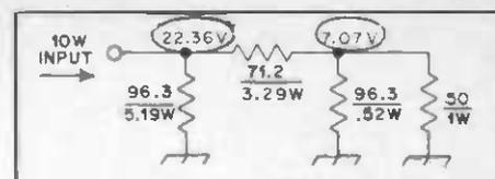
Fig. 22 — A 10-dB pi type of attenuator.
