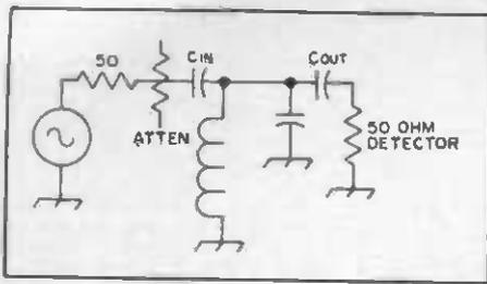
Fig. 10 — Method for determining resonator unloaded  $Q$ .
