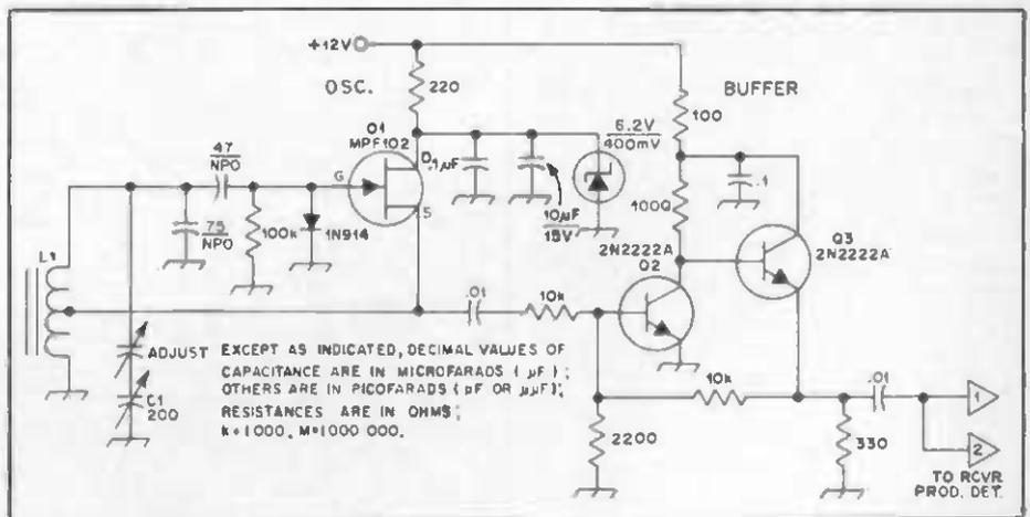
Fig. 31 — 3.5- to 4-MHz VFO for the WA7MLH 75-meter dsb transceiver.
