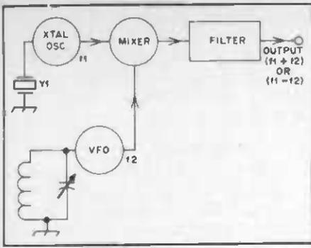
Fig. 25 — Block diagram of a heterodyne frequency generator.
