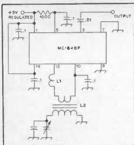
Fig. 28 — An oscillator which employs an MC1648P IC. L1 is a ferrite bead with two turns of wire. L2 is a high  $Q_M$  toroid tuned circuit. The link should contain only the number of turns necessary to sustain oscillation. A typical turns ratio is 4:1.
