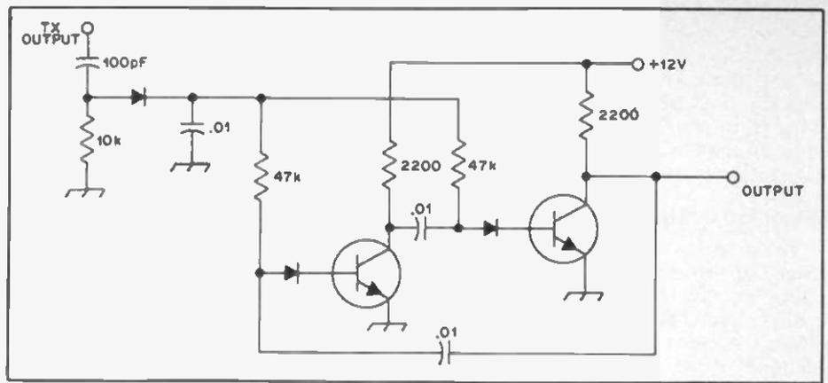
Fig. 76 — Another type of sidetone oscillator (see text).
