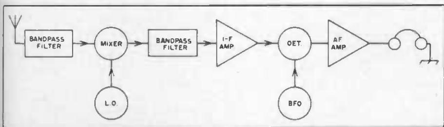
Fig. 2 — Configuration for a basic superheterodyne receiver.
