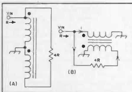
Fig. 12 — Circuit of a 4:1 step-up transformer.
