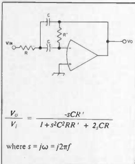
Fig. 21 — Representation of a single-section active band-pass filter.
