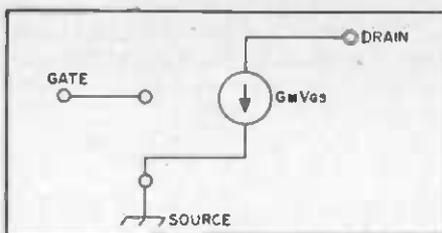
Fig. 7 — Simplified model of a field-effect transistor.
