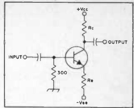
Fig. 10 - Dual supply biasing.
