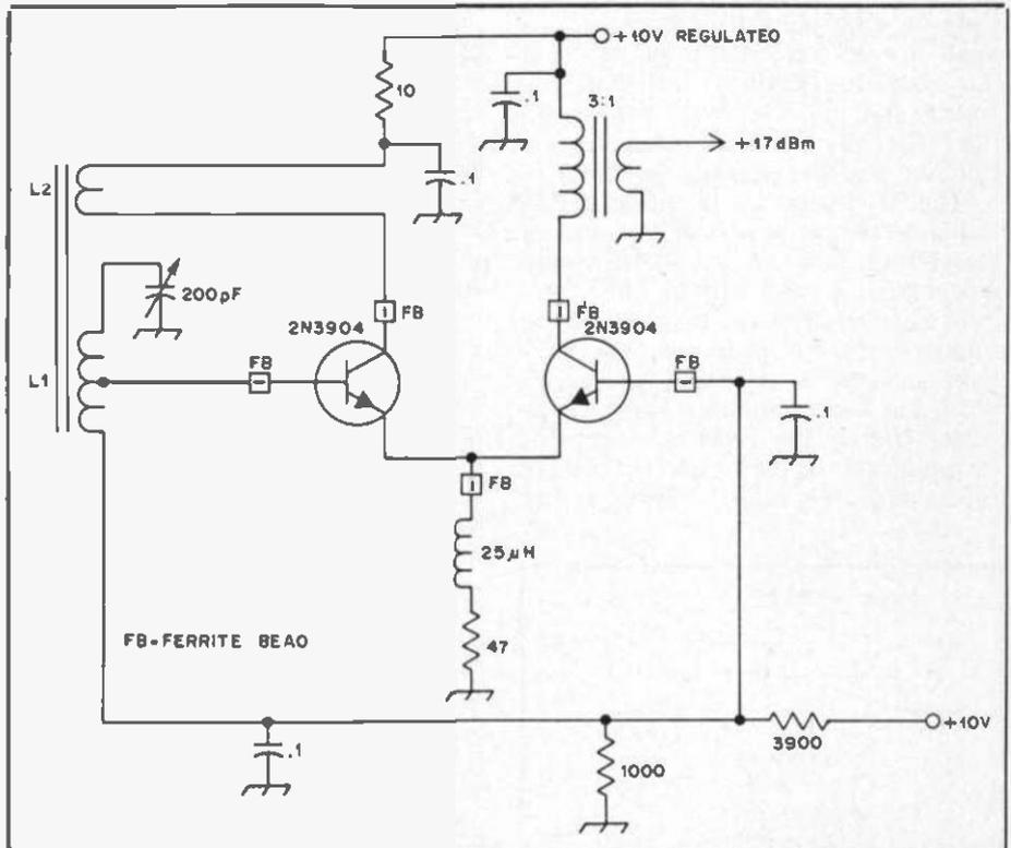
Fig. 26 — Circuit of the K7HFD low-noise oscillator. L1 is 1.2  $\mu$ H and uses 17 turns of wire on a T68-6 toroid core. The tap is at 1 turn. Q at 10 MHz is 250. L2 is a 2-turn link over L1.
