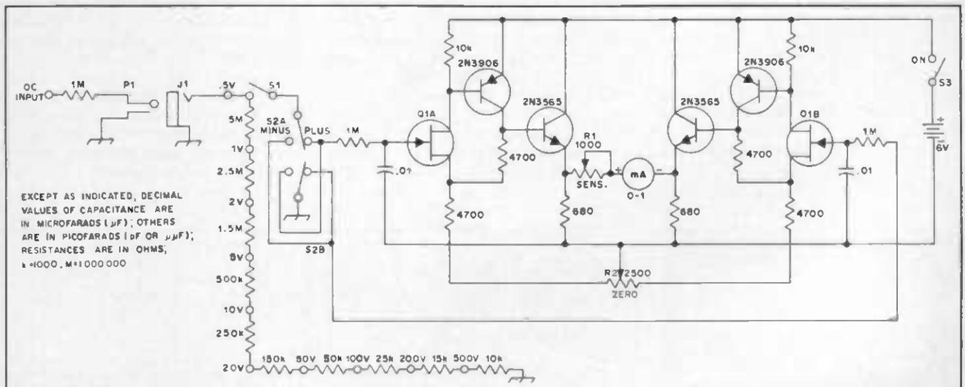
Fig. 5 — A semiconductor equivalent of some of the popular VTVMs used by amateurs. The circuit exhibits low-drift characteristics respective to temperature changes. Q1 = Dual N-channel JFET,  $V_p \approx 1.5V$ .
