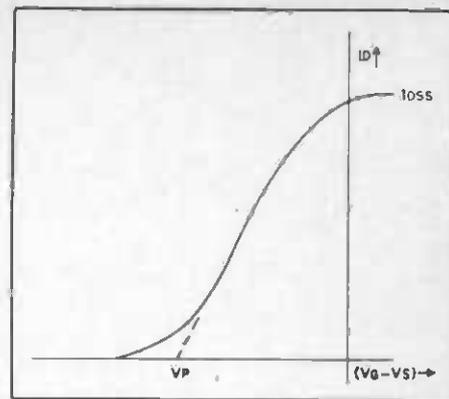
Fig. 17 — Basic dc characteristics of the junction FET.
