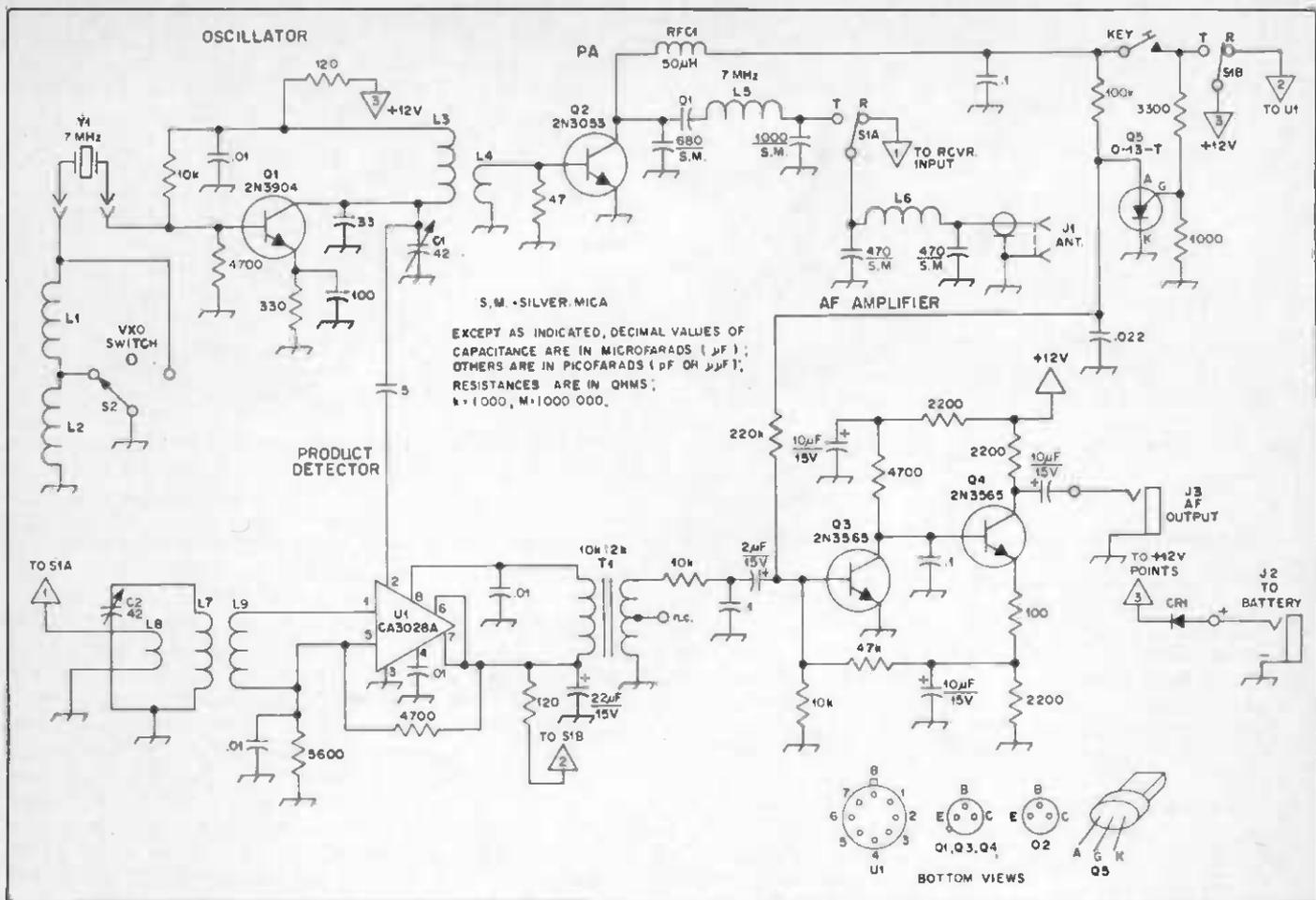
Fig. 6 - Schematic diagram of the ultra-portable transceiver. Fixed-value capacitors are discussed in the text. Resistors are 1/4-watt composition.
