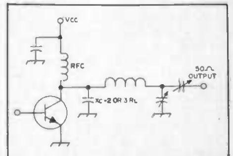
Fig. 30 — Circuit of the modified L-C-C network.
