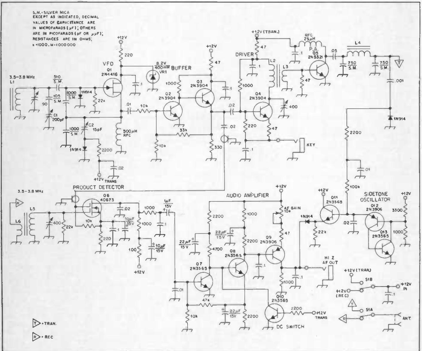
Fig. 7 - Schematic diagram of the KL71AK 80-meter transceiver. Fixed-value capacitors are disk ceramic unless otherwise noted. Polarized capacitors are electrolytic. Unlabeled variable capacitors are mica compression trimmers. Fixed-value resistors are 1/4- or 1/2-W composition.
