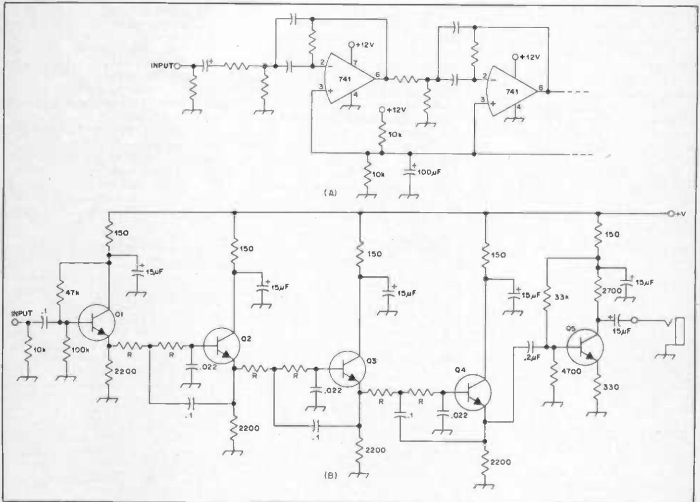
Fig. 24 — Multisection active filters with single power-supply voltage. Q1 to Q5 are 2N3565 (or equiv.). R is 3300  $\Omega$  for 1-kHz cutoff or 1500  $\Omega$  for 2.3-kHz cutoff.
