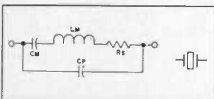
Fig. 32 — Electrical equivalent of a quartz crystal.
