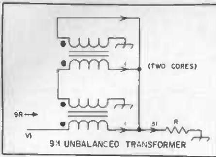
Fig. 15 — Illustration of a 9:1 unbalanced transformer.
