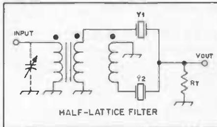
Fig. 35 — Circuit for a half-lattice crystal filter.
