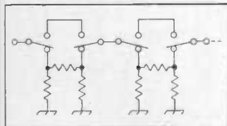
Fig. 21 — Circuit for a step attenuator which is useful into the vhf spectrum.
