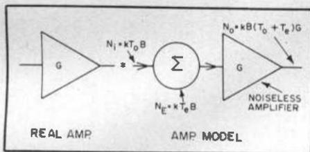
Fig. 1 - The principle of noise temperature.
