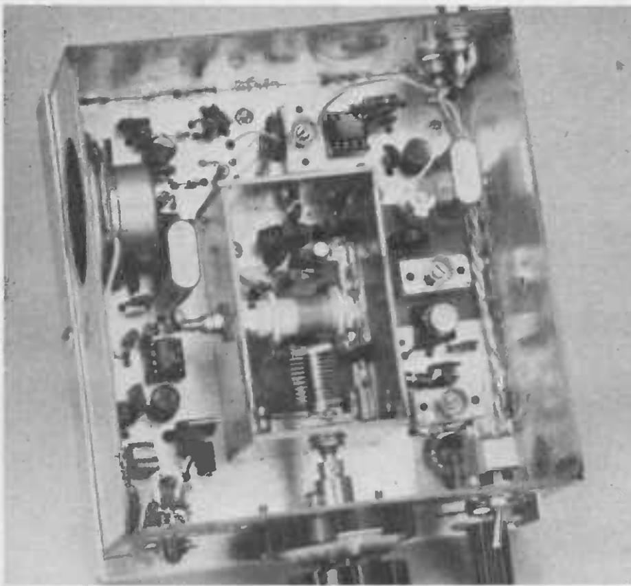
Interior of the unutilized receiver. The local oscillator is seen in its compartment at the center. A press-fit U-shaped cover is placed over the VFO box when the receiver is operating. The receiver front end is at the lower right. At the upper left is a miniature speaker, the rim of which is tack soldered to the box wall at four points. The 20-meter converter board mounts on the rear wall of the box (upper left).
