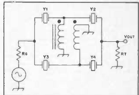
Fig. 36 — Example of a cascaded half-lattice crystal filter.
