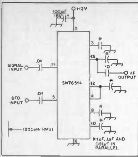
Fig. 7—A product detector can be built from an SN76514 IC. The SN-76514 mixer IC has been reidentified as TL-442-CM by Texas Instruments. It may be procured under either part number.
