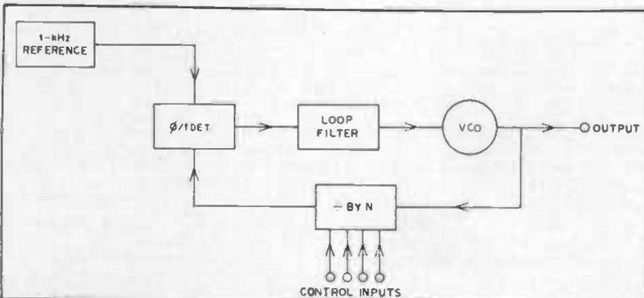
Fig. 35 — Block diagram of a divide-by-N synthesizer.
