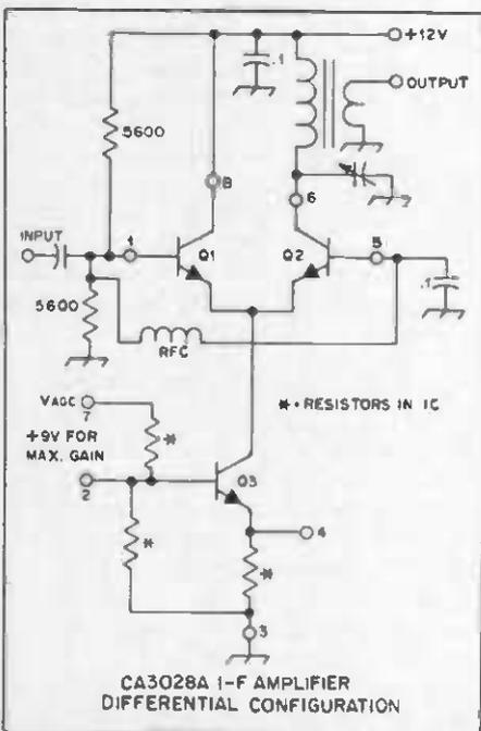
Fig. 44 — Illustration of a CA3028A differential i-f amplifier.
