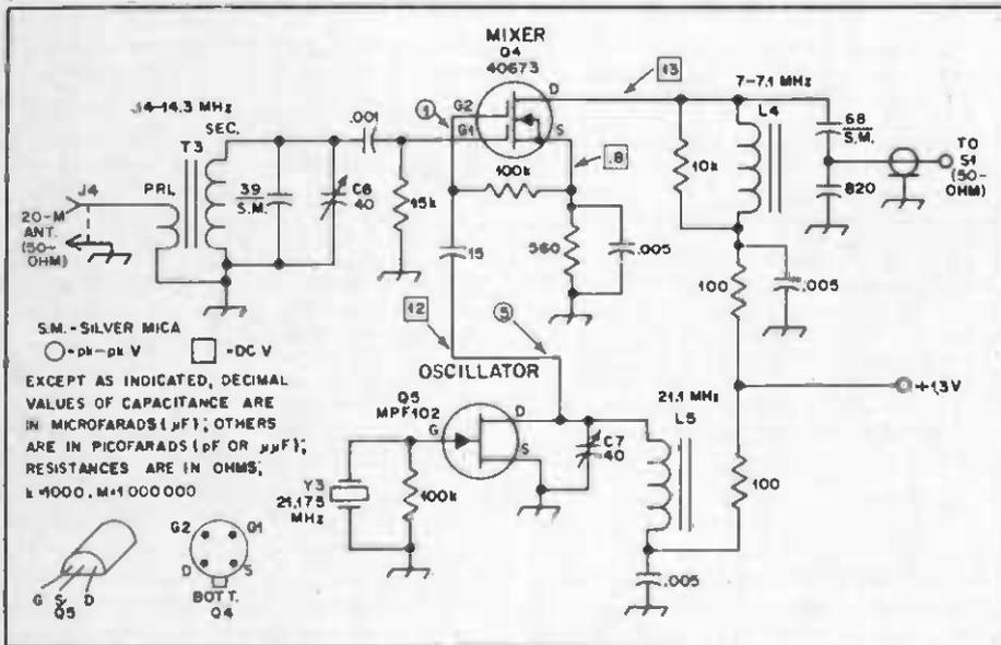
Fig. 76 — Schematic diagram of the 20-meter converter. Fixed-value capacitors are disk ceramic unless noted otherwise. Resistors are 1/4- or 1/2-W composition.
