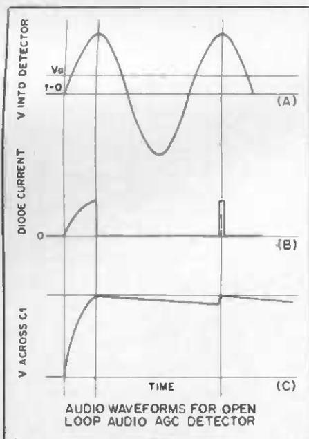
Fig. 51 — Waveforms for open-loop audio agc detector.
