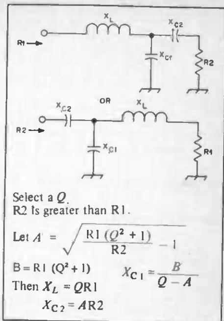
Fig. 5 — The L-C-C matching network with related equations.
