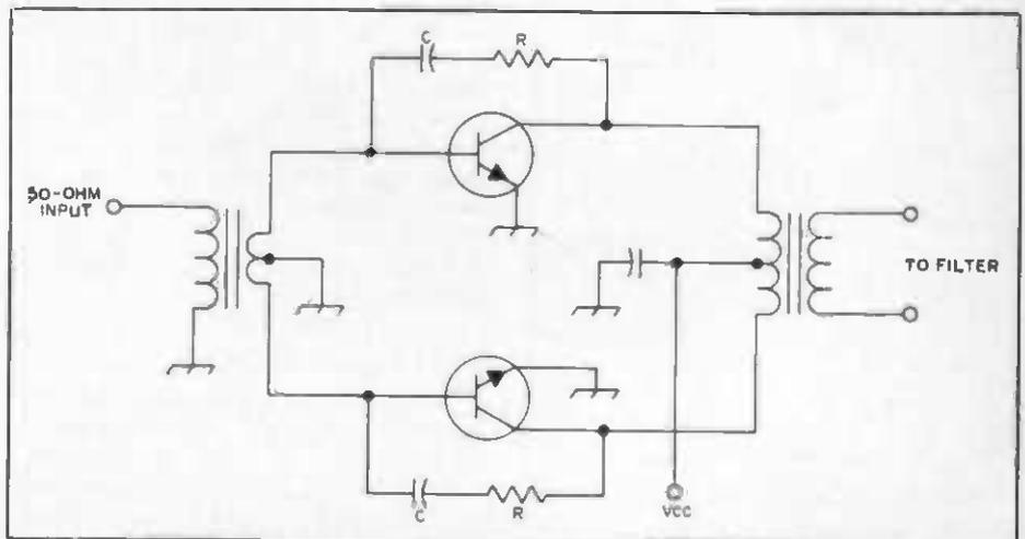
Fig. 26 — Gain compensation networks for negative feedback.
