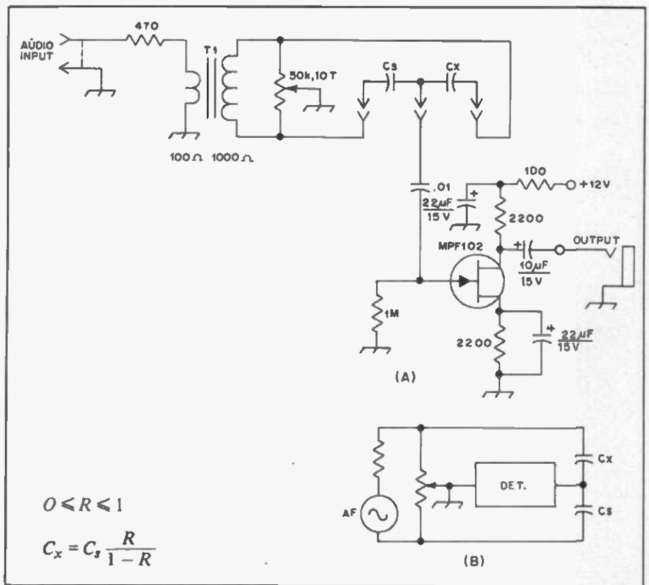
Fig. 64 — Schematic diagram of the capacitance bridge.
