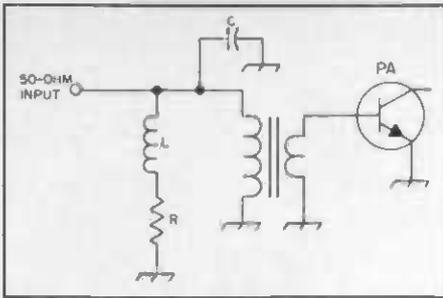
Fig. 24 — Gain-compensating network, labeled L and R.
