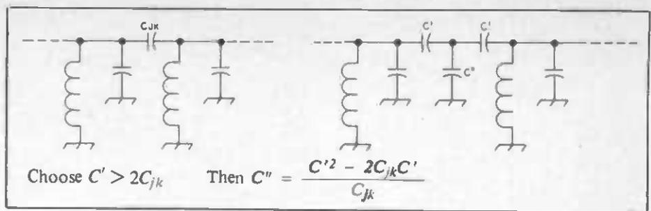
Fig. 8 — Method for dealing with small values of coupling capacitors.
