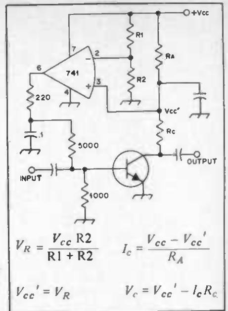
Fig. 14 — An operational amplifier supplying the bias voltage.
