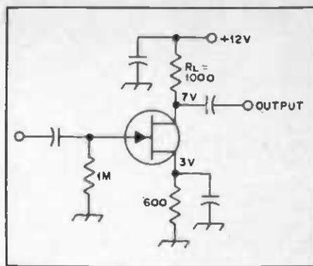
Fig. 21 — Audio amplifier using a JFET.
