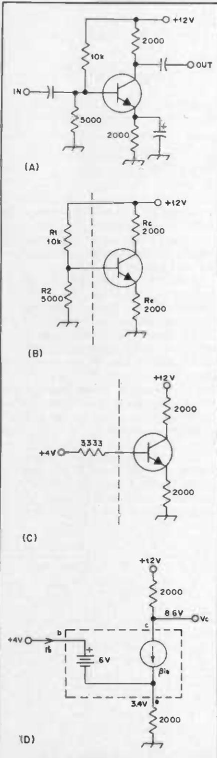
Fig. 9 - Typical bias arrangement for a well-designed amplifier.
