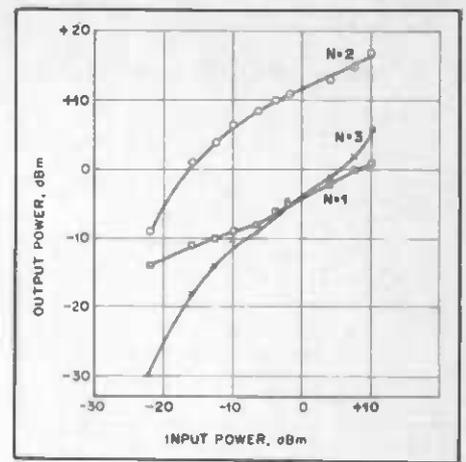
Fig. 16 — Input power versus output power in dBm for a bipolar-transistor frequency doubler. See text for explanation of the curves.
