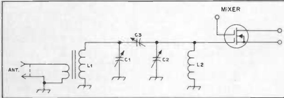
Fig. 63 — A singly terminated double-tuned input circuit.
