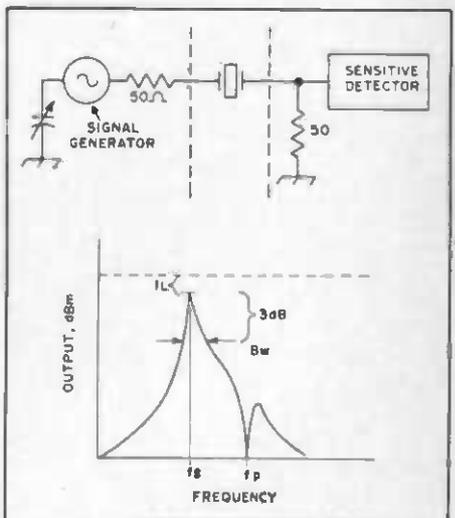
Fig. 33 — Test setup for evaluating a quartz crystal.
