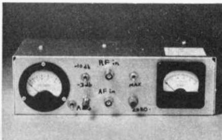
A general-purpose test instrument. The meter at the left is for readout of an audio voltmeter. The instrument is not calibrated, but there are calibrated attenuations of 3 and 10 dB. The meter at the right is an indicator for a broadband rf detector. A broadband amplifier is contained in the case. It allows sensitivities of -65 dBm up through 50 MHz. The rf detector is used in conjunction with a step attenuator to produce 1-dB accurate measurements of gain, return loss and related parameters.
