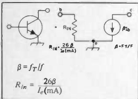
Fig. 1 — Simplified model for a bipolar transistor.
