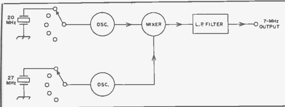
Fig. 31 — Representation of a simple 7-MHz synthesizer.
