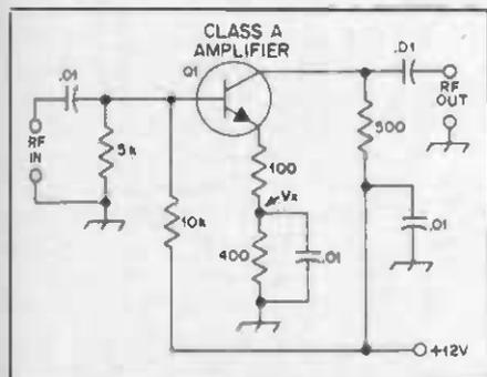
Fig. 8 — Class A amplifier using emitter degeneration.
