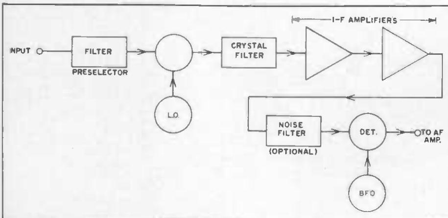
Fig. 38 — Block diagram of a modern superheterodyne receiver.
