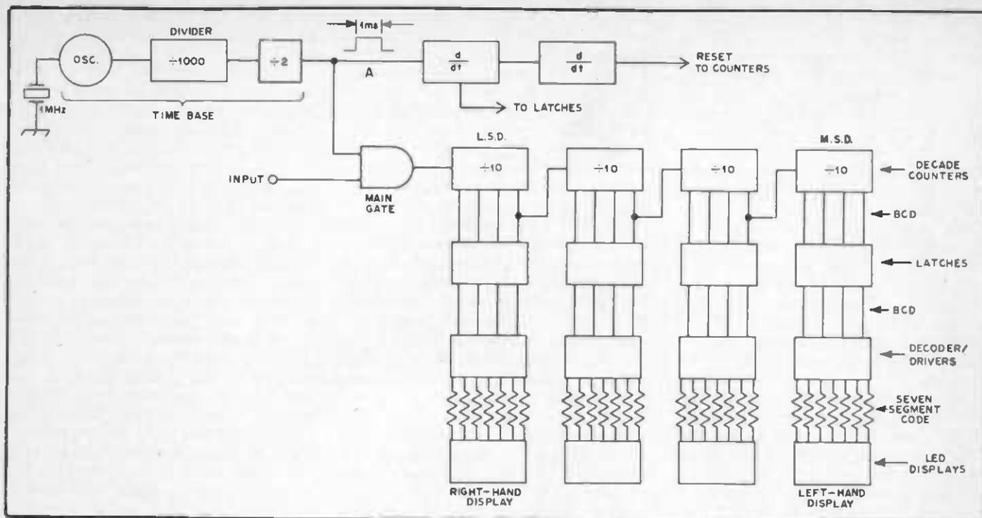
Fig. 33 — Block diagram of a fundamental frequency counter.
