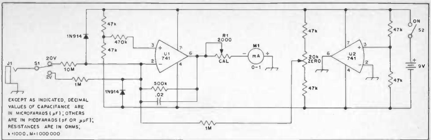
Fig. 4 — Circuit of the op-amp voltmeter.
