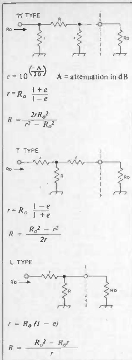
Fig. 20 — Three circuits for forming resistive attenuators.
