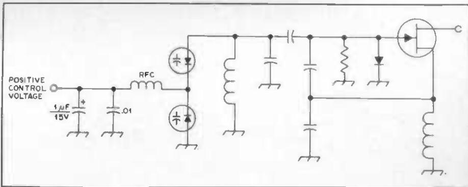
Fig. 3 — VFO circuit showing varactor-diode tuning.
