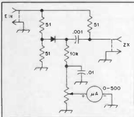
Fig. 27 - A bridge circuit which has a sensitivity control.
