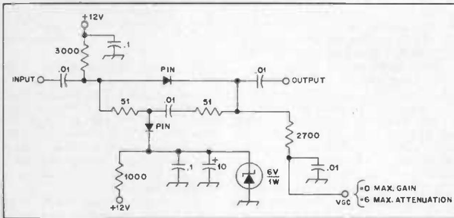
Fig. 48 — Bridge-Tee attenuator using PIN diodes.
