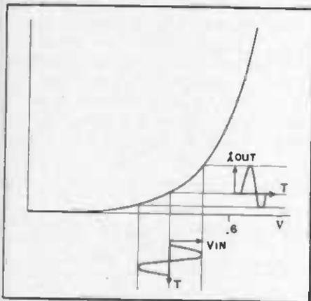
Fig. 10 - Small-signal waveform applied to a diode detector and the resultant output.
