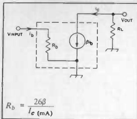
Fig. 16 — Small-signal model of the audio amplifier.
