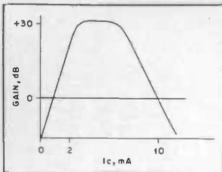
Fig. 40 — Gain as a function of current.
