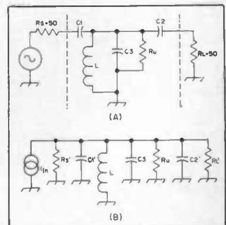
Fig. 5 - Example of a filter which has loss.
