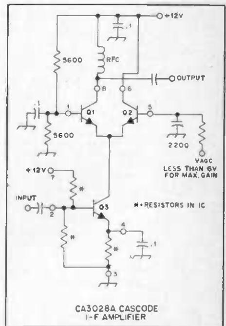
Fig. 45 — Cascode i-f amplifier using a CA3028A IC.
