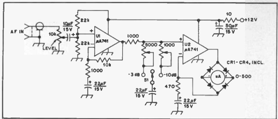
Fig. 63 — Details of the audio voltmeter. CR1 through CR4 are 1N914s. M1 is a 500-μA meter, and S1 is a center-off spst toggle switch.
