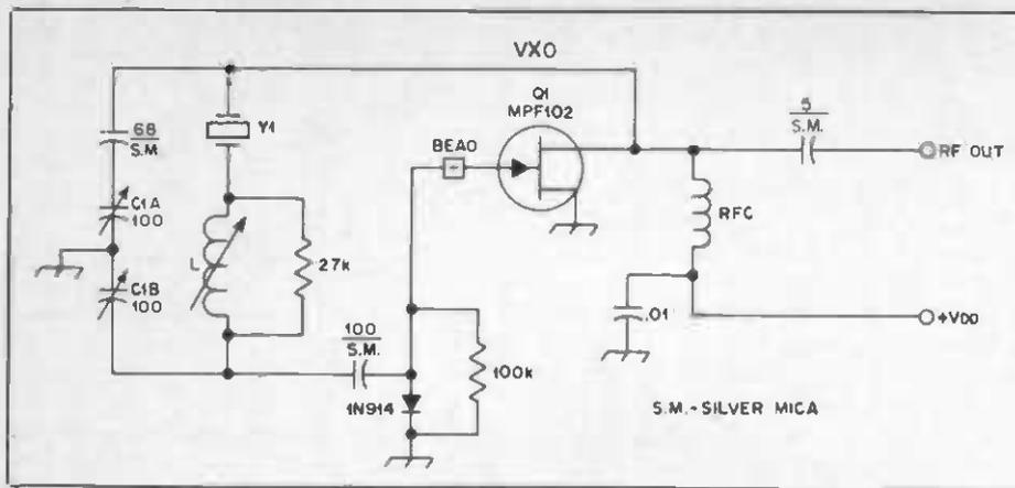
Fig. 5 - Vxo circuit for pulling the crystal frequency.
