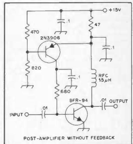
Fig. 17 — A post mixer amplifier without feedback.
