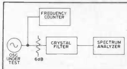
Fig. 27 — System for evaluating the oscillator of Fig. 26.
