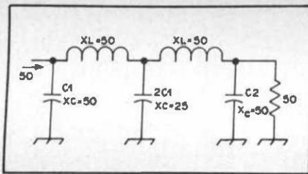
Fig. 7 — Half-wave filter network circuit.
