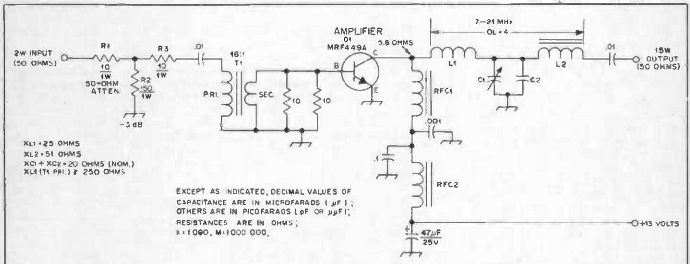
Fig. 36 — Schematic diagram of the 15-watt amplifier. Fixed-value capacitors are disk ceramic unless otherwise noted. Resistors are 1/2-watt composition unless specified differently. The  $47\text{-}\mu\text{F}$  capacitor can be electrolytic or tantalum.
