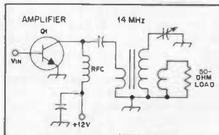
Fig. 16 — Example of a link-coupled output network.
