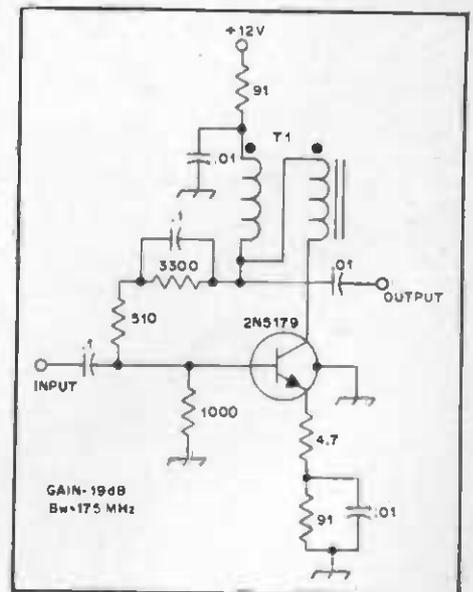
Fig. 12 - Diagram of a broadband amplifier which can be used to extend power-meter sensitivity to lower power levels. T1 contains 7 bifilar turns of enameled wire on an Amidon FT-23-43 toroid core. Circuit gain is 19 dB and the bandwidth is 175 MHz.
