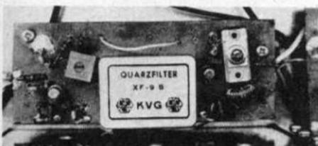
The 9-MHz i-f amplifier used in the universal ssb/cw transmitter.
