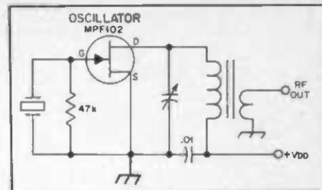
Fig. 4 — Crystal oscillator which employs a JFET.
