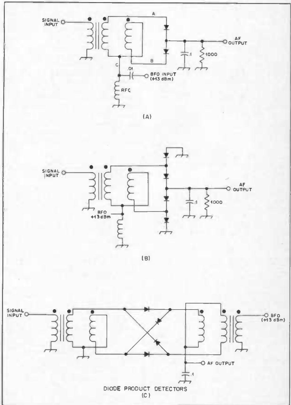
Fig. 9 — Examples of three diode detectors.
