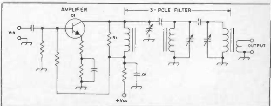
Fig. 14 — Buffer amplifier with a three-pole output filter.
