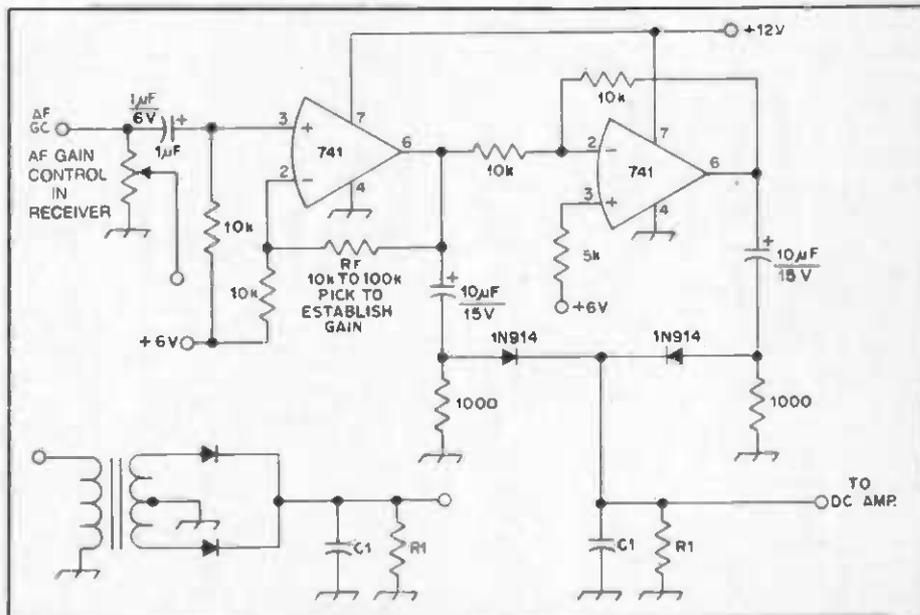
Fig. 53 — Examples of full-wave audio agc detectors.
