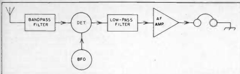
Fig. 1 — Block diagram of a direct-conversion receiver.
