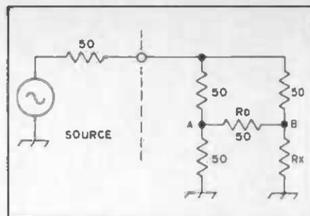
Fig. 35 — Another version of a simple resistive bridge.
