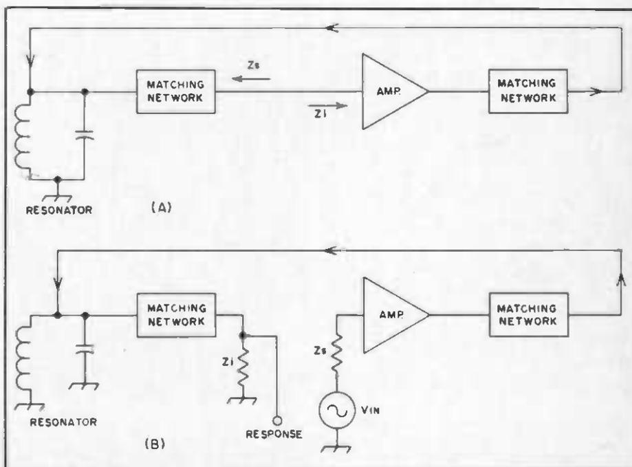
Fig. 1. — Block diagram of an LC oscillator.
