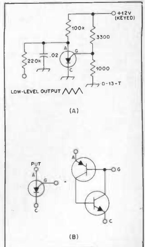
Fig. 74 — Circuit of a PUT audio oscillator.
