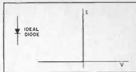
Fig. 2 — Current flow in the "ideal" diode.
