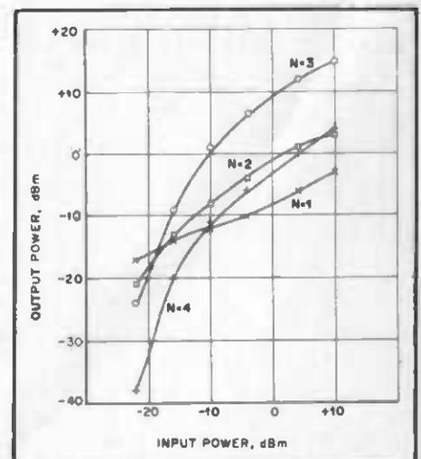
Fig. 17 — Input power versus output power for a bipolar-transistor frequency tripler. See text for data concerning the curves.
