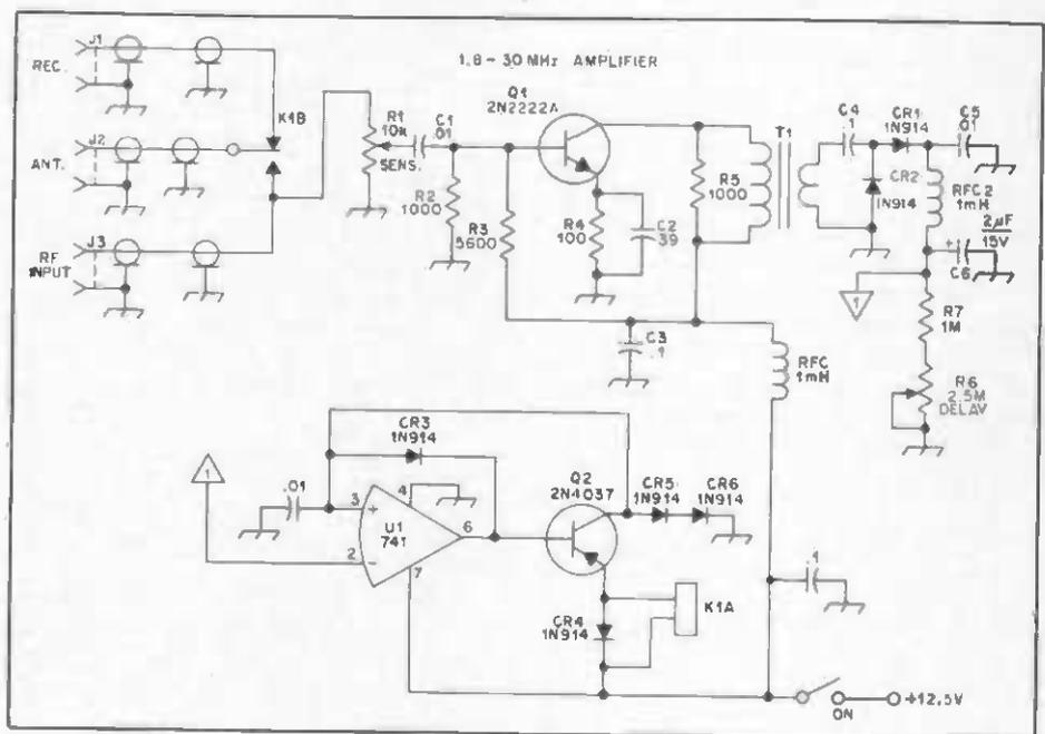
Fig. 85 — Circuit of an rf-actuated relay driver. This unit was first described in *QST* for Aug., 1976, p. 21, inclusive of a pc-board layout. K1 is a 12-V relay with a field coil dc resistance between 500 to 1,000 ohms. T1 primary has 25 turns of No. 28 enam. wire on an Amidon FT-50-43 toroid core. The secondary consists of 5 turns of No. 28 wire wound over the primary. RFC1 and RFC2 contain 42 turns of No. 28 enam. wire on FT-50-43 toroid cores.
