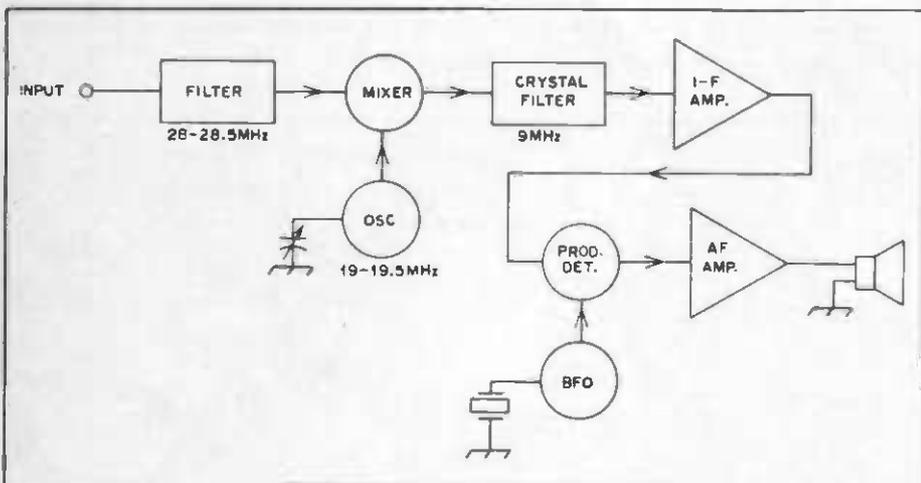
Fig. 28 — Representation of modern-day single-conversion superheterodyne receiver.
