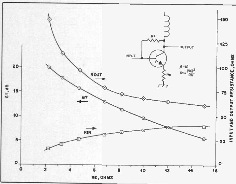
Fig. 18 —  $G_t$ ,  $R_{in}$  and  $R_{out}$  as a function of feedback components. A simple model was assumed for this calculation with a beta of 10. No account was taken for phase shifts in beta. Nonetheless, the calculations agree well with measured results. A profound advantage of feedback is predictability in design.
