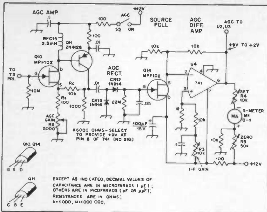
Fig. 39 — Schematic diagram of the agc system. Capacitors are disk ceramic except when polarity is indicated, which signifies electrolytic. Fixed-value resistors are 1/2-W composition. This module is not enclosed in a shield compartment.
