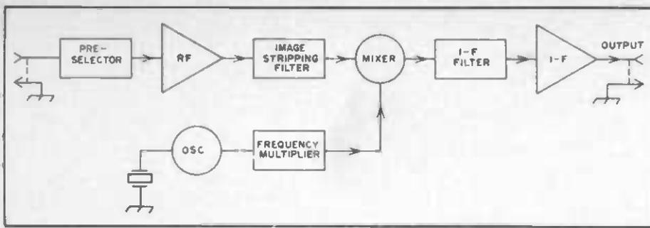
Fig. 30 — Block diagram of a typical crystal-controlled converter.
