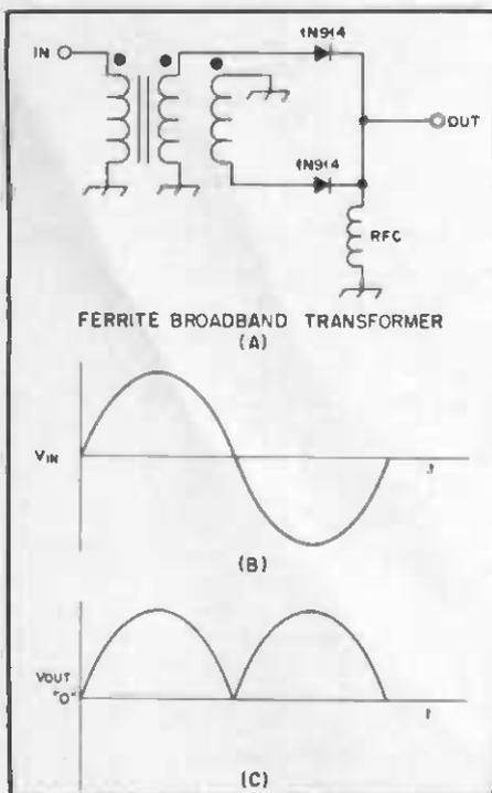
Fig. 19 — Illustration of a diode frequency doubler.
