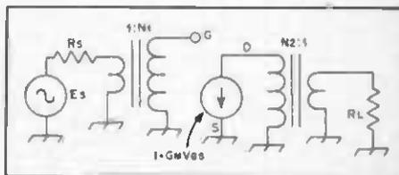
Fig. 8 — Common-source FET amplifier with transformer coupling at the input and output.
