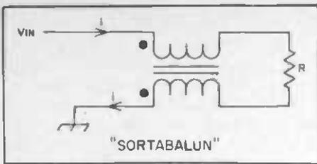
Fig. 11 — Circuit for an isolation transformer.
