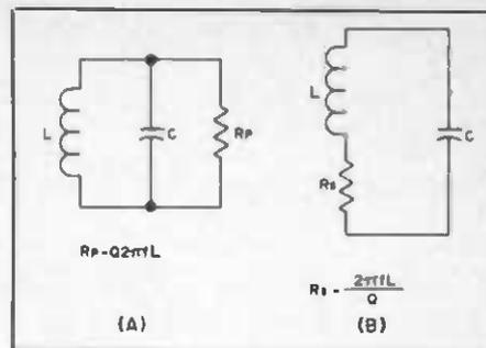
Fig. 12 - Schematic representation of circuit losses.
