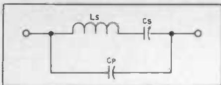
Fig. 2 — Equivalent circuit for a quartz crystal.
