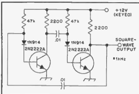
Fig. 75 — Sidetone oscillator using a multivibrator.
