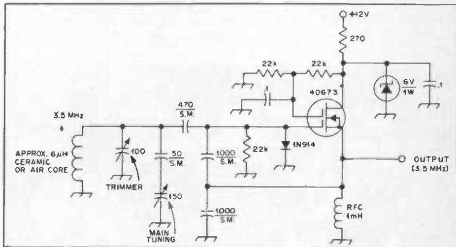
Fig. 4 — Circuit of a dual-gate MOSFET VFO.
