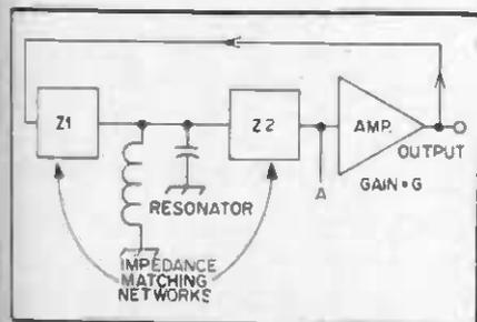
Fig. 22 — Generalized diagram of an oscillator.
