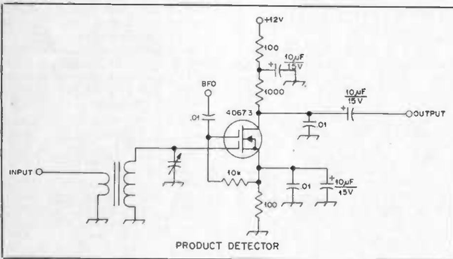
Fig. 5 — Example of a dual-gate MOSFET product detector.
