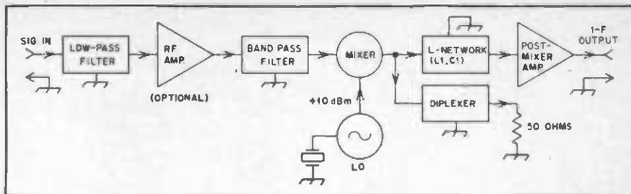
Fig. 41 — Block diagram of the CER-verters.
