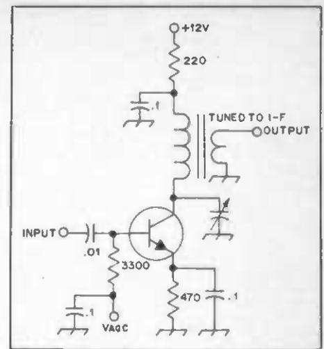
Fig. 39 — A single stage of i-f amplification, utilizing a bipolar transistor.
