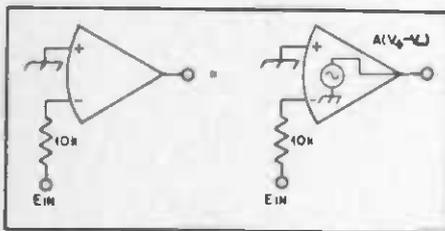
Fig. 24 — Operational amplifier connected in the inverting configuration.
