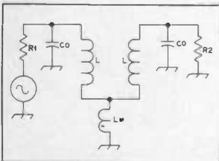
Fig. 7 — Mutual-inductor coupling method.
