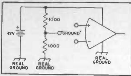
Fig. 23 — Synthetic ground for an operational amplifier.
