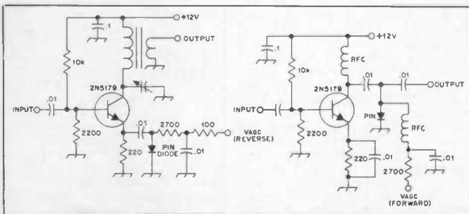
Fig. 47 - Gain control by means of PIN diodes.
