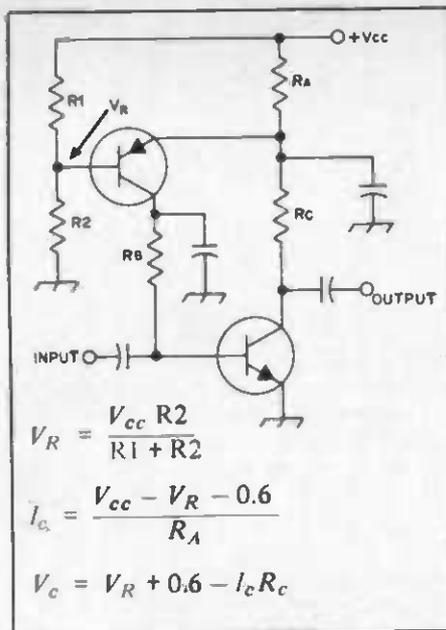
Fig. 13 — Separate transistor acting as a bias source.
