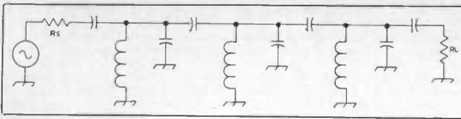
Fig. 6 — Example of a multi-resonator filter.
