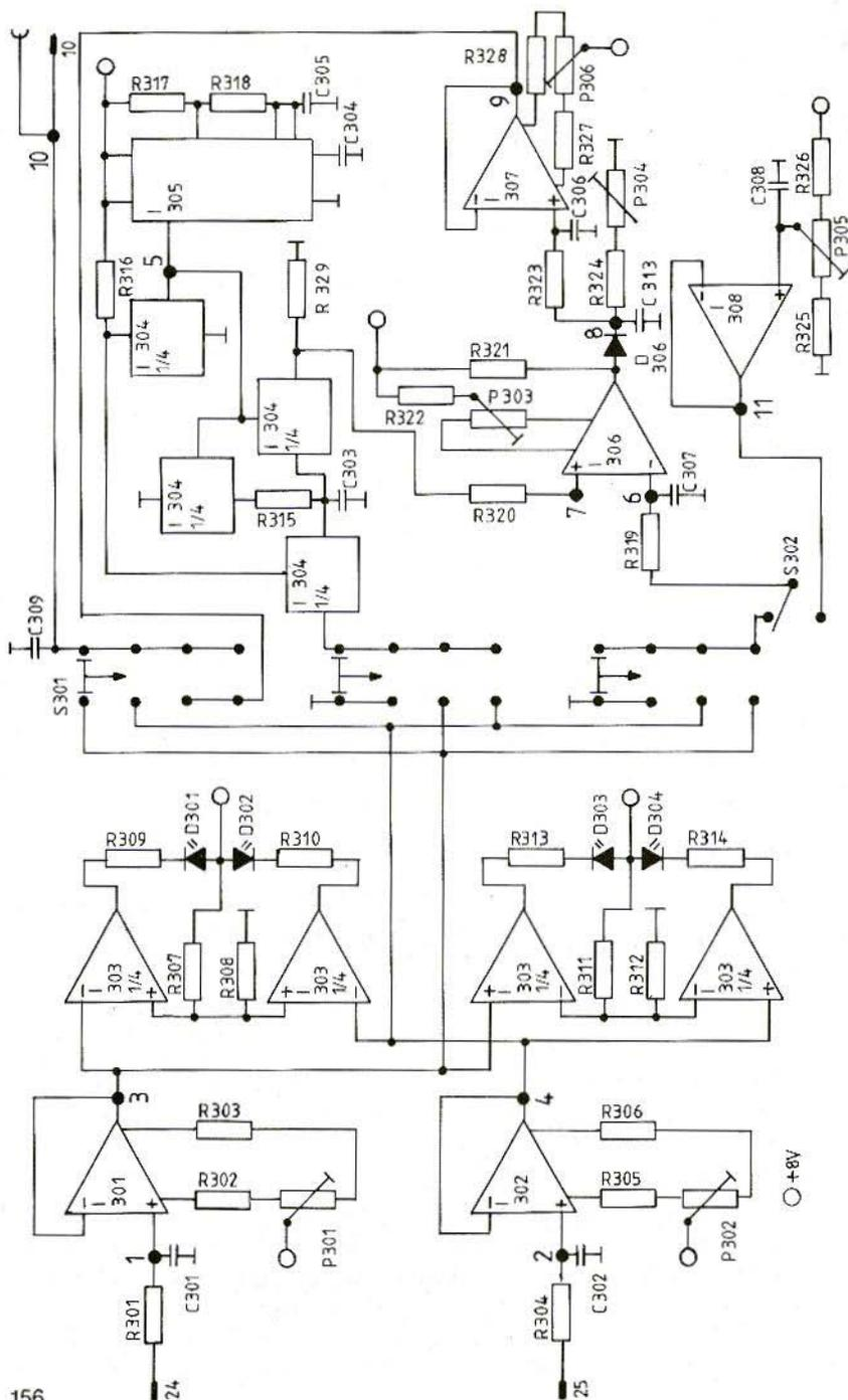
Fig. 32: The logarithmic circuit
