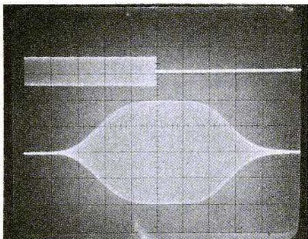
Fig. 5a: Pulse behaviour of the CCW-filter module with input and output pulse displayed linearly. Pulse duration: 12.5 ms; time scale: 2.5 ms/division
