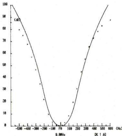
**Fig. 3:** Theoretical passband curve of the CCW-filter; the values marked with "x" are the measured values of the home-made filter
