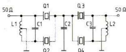
**Fig. 2:** A four-pole crystal filter as described by DK 1 AG (1)
