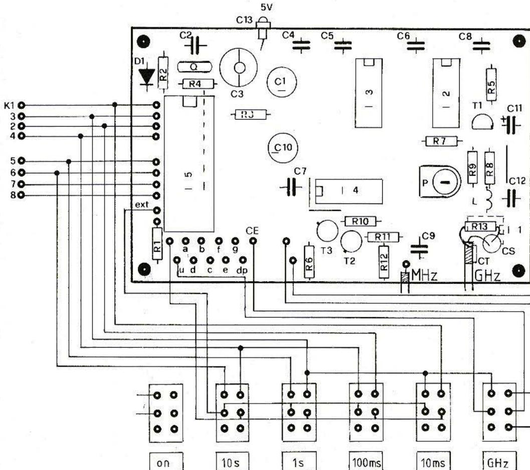
Fig. 3: Component and wiring plan for the counter board DCØRZ 002
