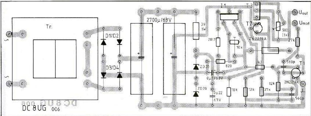
Fig. 10: Component locations on the power supply/switching amplifier board DC 8UG 006
