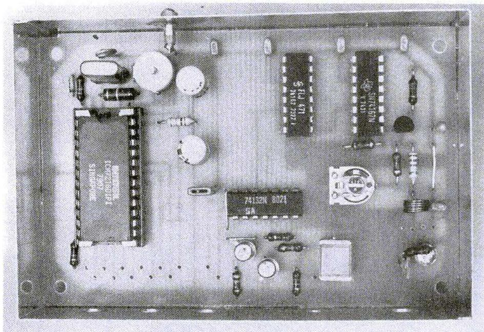
Fig. 5: One will see the input circuit of the U 664 B of the counter module
