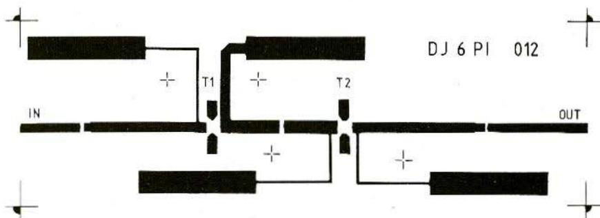
Fig. 2: PC-board DJ6PI 012 for the 2-stage preamplifier using a 0.79 mm thick epoxy PC-board
