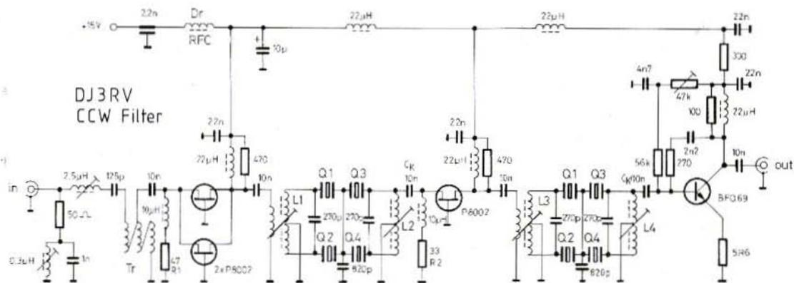
Fig. 4: Circuit diagram of the whole CCW-filter module
