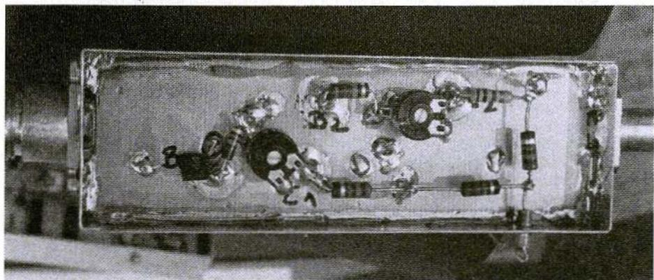
Fig. 7: The DC-voltage network can be accommodated on the ground side of the board between the feedthrough capacitors and the ground surface
