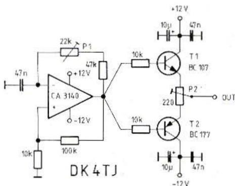
Fig. 5: 1000 Hz drive circuit
