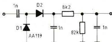
Fig. 2: The demodulator probe should be built up using good UHF-practice
