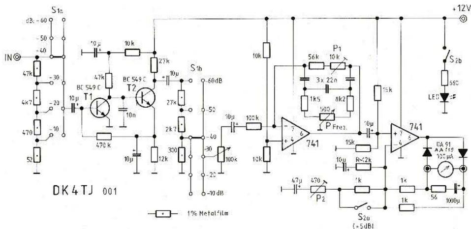
Fig. 1: The VSWR-indicator comprises AF-amplifier, 1000 Hz-filter and linear rectifier
