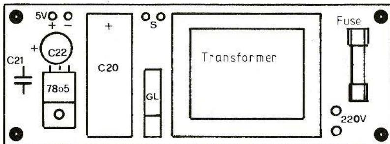
Fig. 7: Power supply board DC 0RZ 004 is able to provide 300 mA at +5 V
