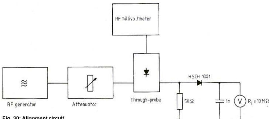
**Fig. 30: Alignment circuit**
