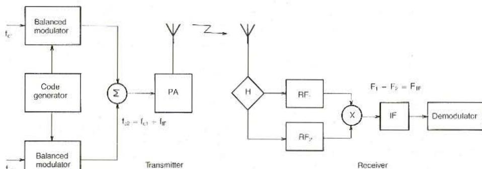
Fig. 11: Synchronization method using a transmitted reference signal
