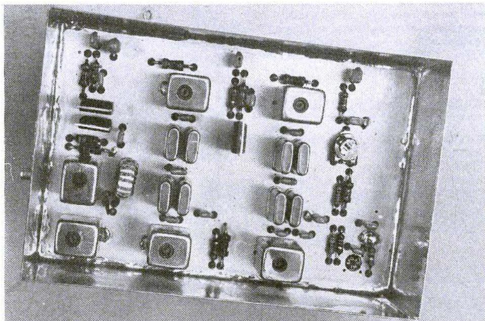
Fig. 1: Photograph of the author's prototype CCW-crystal filter for use as a module in the IF-circuit designed by DJ3RV (VHF COMMUNICATIONS 14, Ed. 4/82, Pages 239-252)
