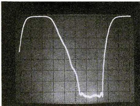
Fig. 5b: Output pulses of the CCW-filter module in a logarithmic display of the amplitude. Pulse duration: 12.5 ms; pulse repetition frequency: 25 Hz; amplitude: 10 dB/division; time scale: 5 ms/division
