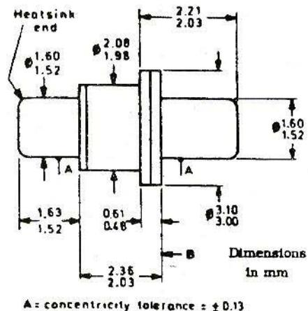
Fig. 1: Case and dimensions of the noise diode BAT 31
