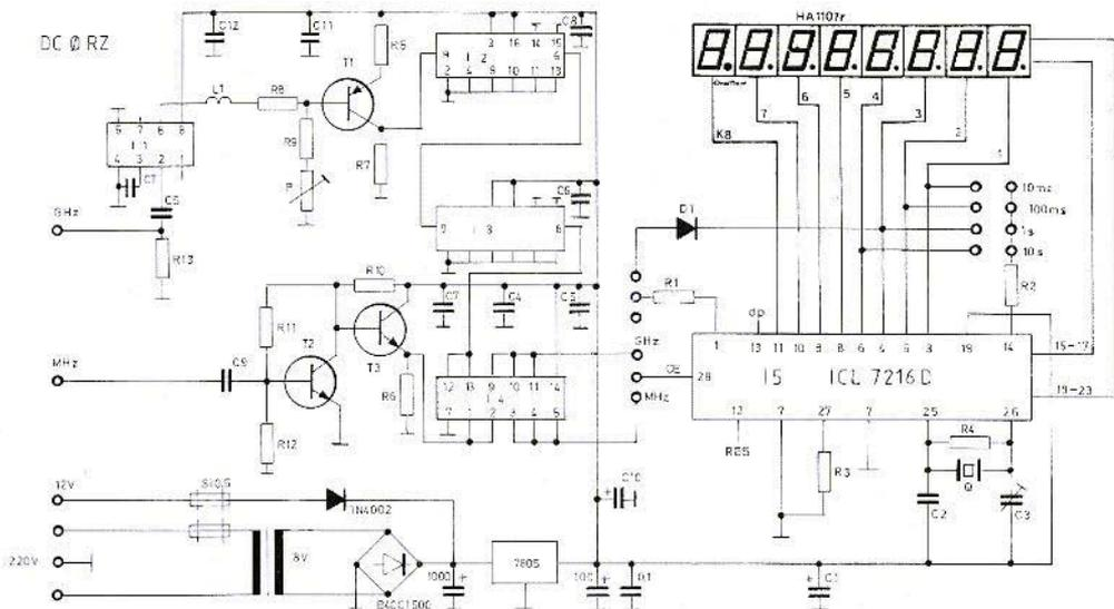
Fig. 2: Circuit diagram of the counter with eight-digit readout and power supply
