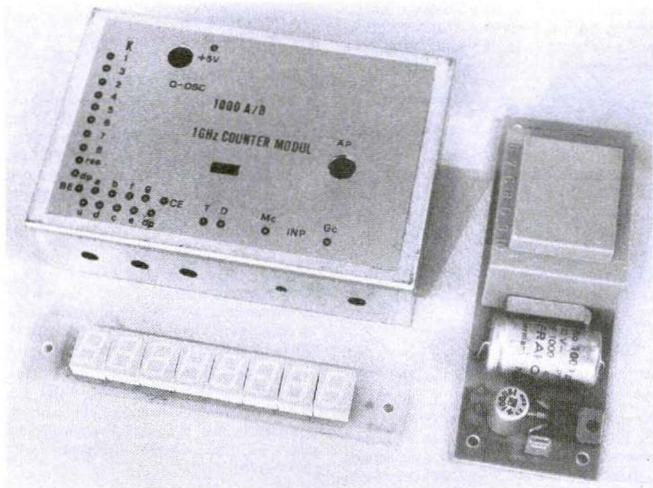
Fig. 1: Counter module, readout, and power supply before the connection
