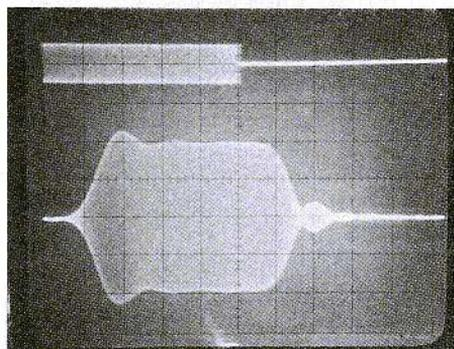
Fig. 6a: Pulse behaviour of a filter with Tschebyscheff characteristic (XF-9NB). Input and output pulse displayed linearly. Scales as in Figure 5a.
