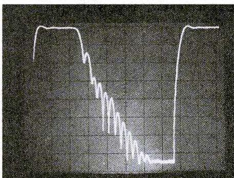
Fig. 6b: Output pulse of a XF-9NB filter with the amplitude displayed logarithmically. Pulse duration: 12.5 ms; pulse repetition frequency: 25 Hz; scales as shown in Fig. 5b.
