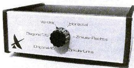
Ready-to-operate as described in VHF COMMUNICATIONS 2/1973. Complete with three BNC connectors (N or SO 239 connectors are also available) in an attractive cabinet. Especially designed for use with crossed yagi antennas mounted as an "X", and fed with equal-length feeders.
