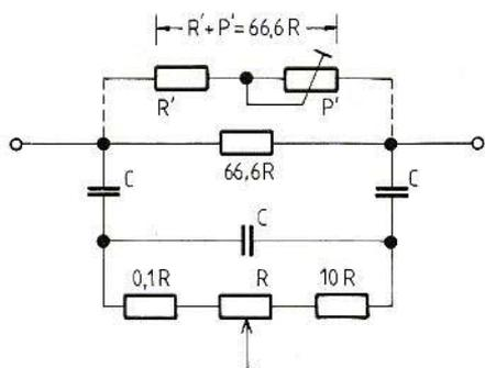
Fig. 10: Design of the filter for a tuning range of 1:3
