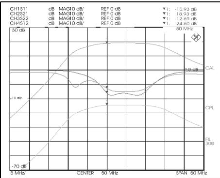
**Fig 15: Frequency response of the completed LNA**
