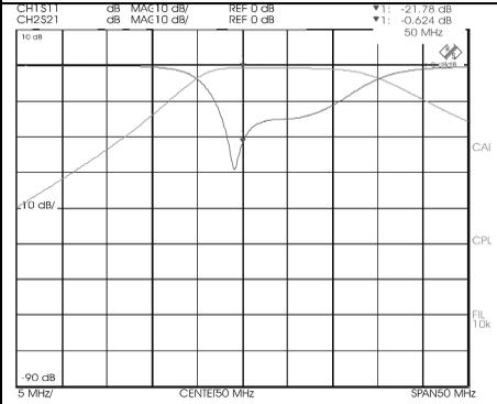
**Fig 10: Measured performance of the 50MHz bandpass filter.**
