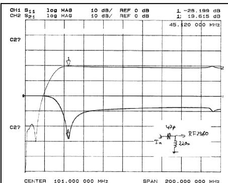
**Fig 14: Frequency response at the input of the LNA.**
