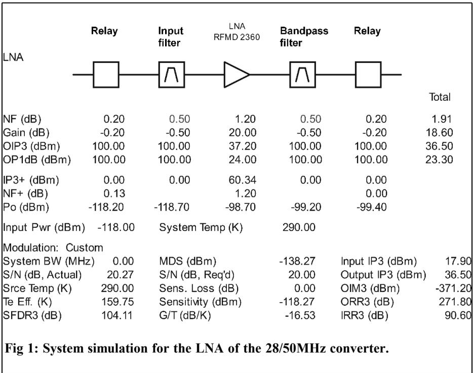
given a value of +100dBm. This value is for real filters, which are assembled using ferrite materials. This is unrealistic, but can be used as an approximation for a starting point at low input levels.
