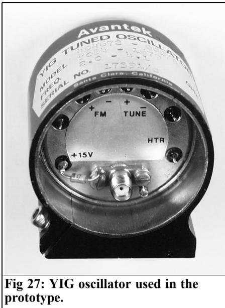
**Fig 27: YIG oscillator used in the prototype.**
