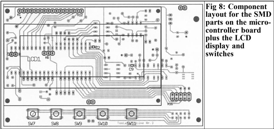
**Fig 8: Component layout for the micro-controller board plus the LCD display and switches**
