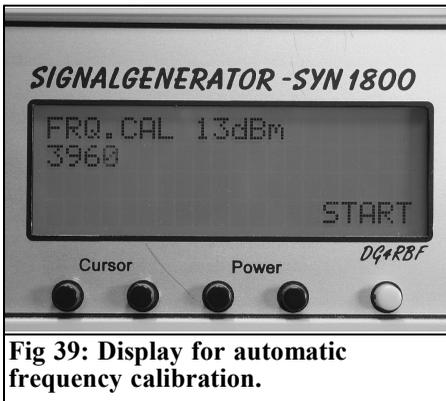
**Fig 39: Display for automatic frequency calibration.**
