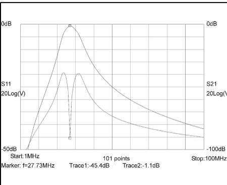
**Fig 23: Simulated performance of the diplexer.**
