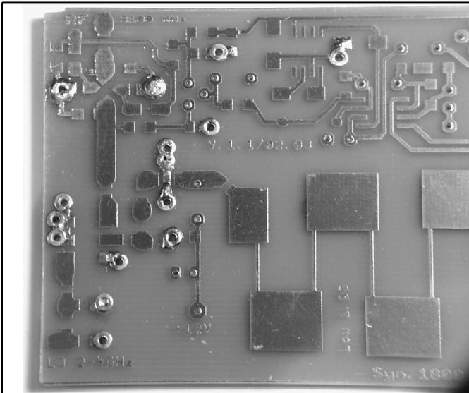
**Fig 34: Example of through hole plating.**
