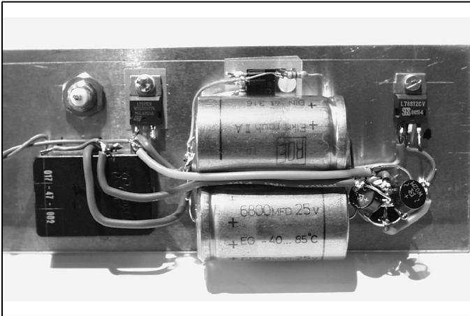
**Fig 35: Power supply components mounted on the rear panel of the unit.**
