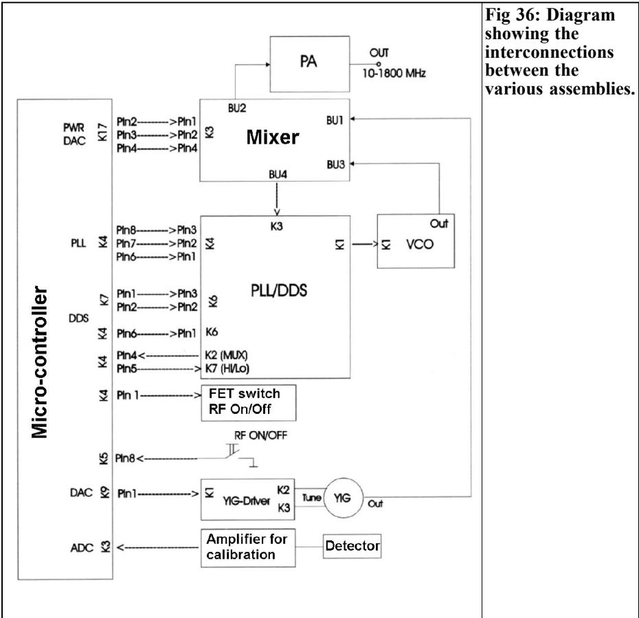
**Fig 36: Diagram showing the interconnections between the various assemblies.**
