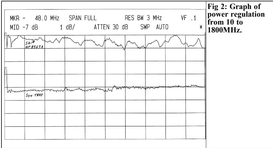
**Fig 2: Graph of power regulation from 10 to 1800MHz.**
