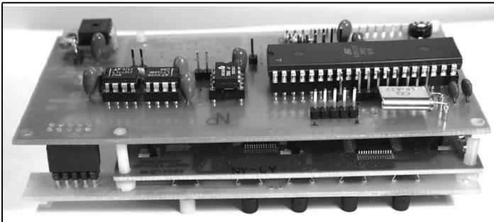
**Fig 5: View of the micro-controller board with the LCD display underneath.**
