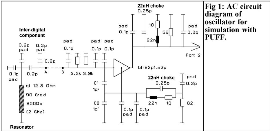
**Fig 1: AC circuit diagram of oscillator for simulation with PUFF.**
