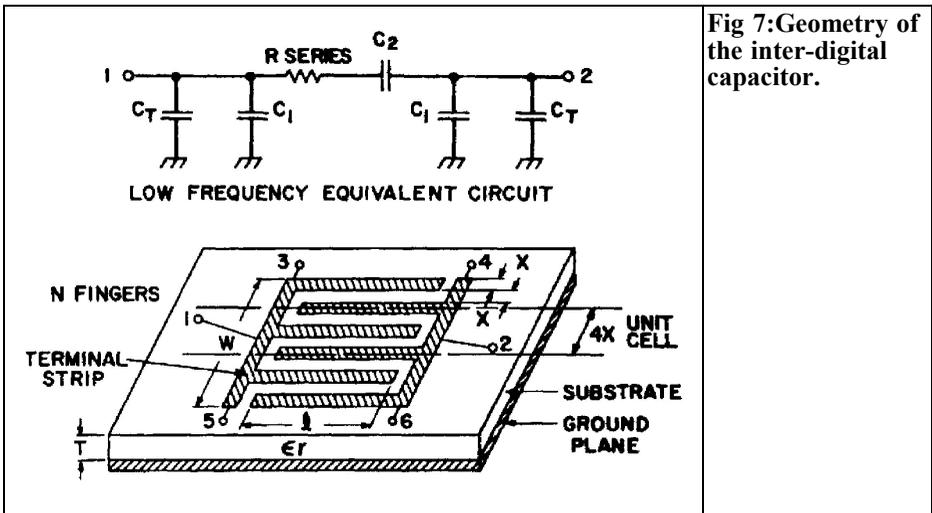
**Fig 7: Geometry of the inter-digital capacitor.**
