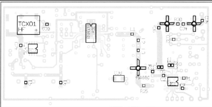
Fig 25: SMD component layout for the PLL/DDS board.
