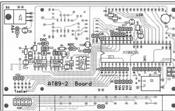
**Fig 7: Component layout for the AT89-2 micro-controller board.**
