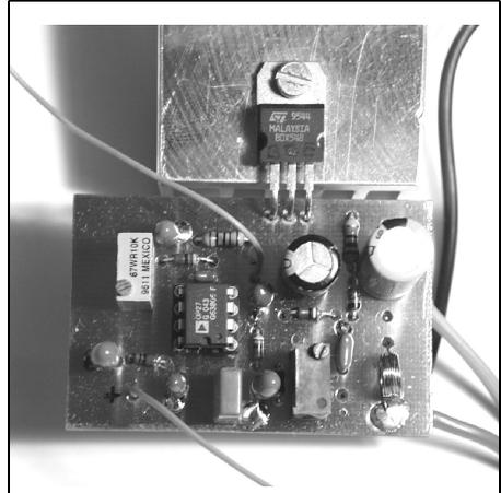
**Fig 31: The completed YIG driver assembly.**
