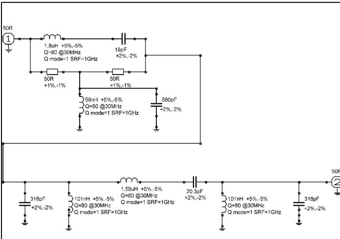
**Fig 26: Circuit diagram of the diplexer for 10MHz bandwidth.**
