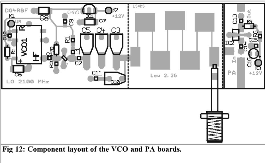
**Fig 12: Component layout of the VCO and PA boards.**
