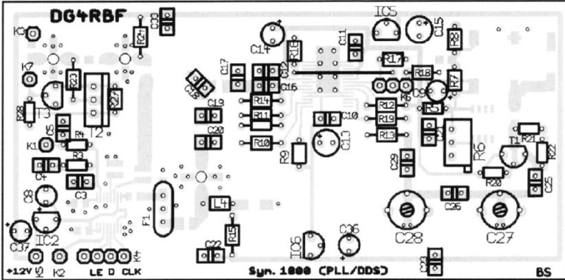
Fig 24: Component layout for the PLL/DDS board.
