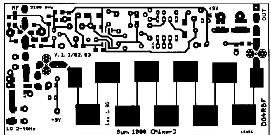
Fig 15: PCB layout for the mixer and filter.
