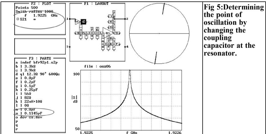
**Fig 5:** Determining the point of oscillation by changing the coupling capacitor at the resonator.
