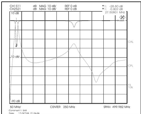
**Fig 21: Measured wide band performance of the 28MHz filter.**
