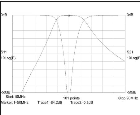
**Fig 9: Simulated performance of the 50MHz bandpass filter.**
