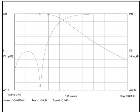
**Fig 13: Simulated performance of the 60MHz low pass filter.**
