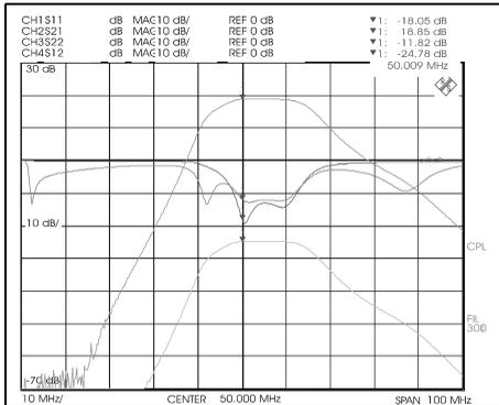
**Fig 16: Frequency response of the completed LNA**
