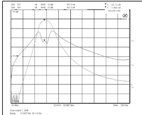
**Fig 28: Measured performance of the diplexer.**
