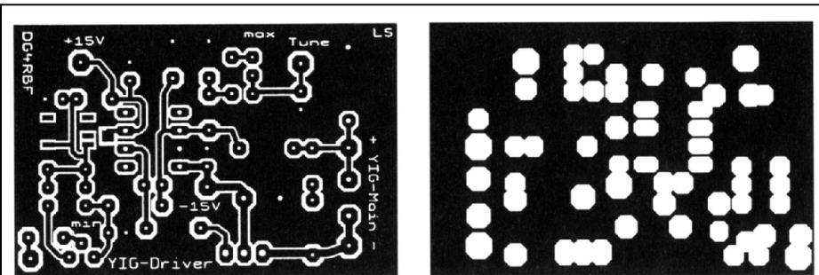
Fig 29: PCB layout for the YIG driver.
