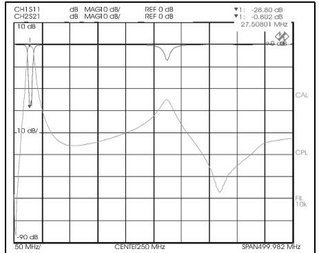
**Fig 11: Measured wide band performance of the 50MHz filter.**
