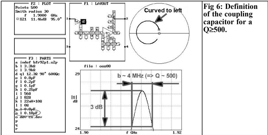
**Fig 6: Definition of the coupling capacitor for a  $Q > 500$ .**
