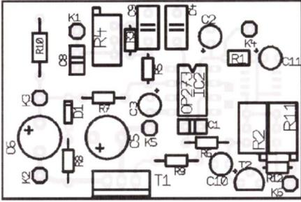
**Fig 30: Component layout fro the YIG driver**
