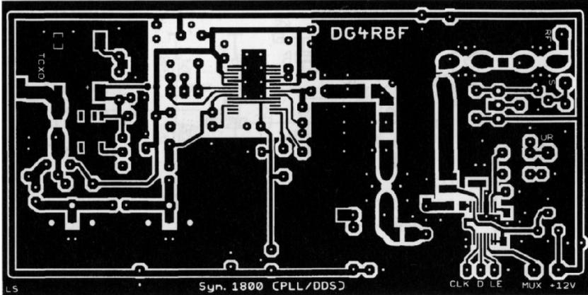
**Fig 22: Track side PCB layout for the PLL/DDS board.**
