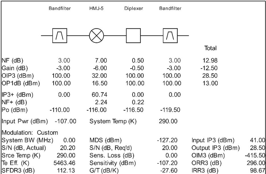
**Fig 2: System simulation for the converter of the 28/50MHz converter.**
