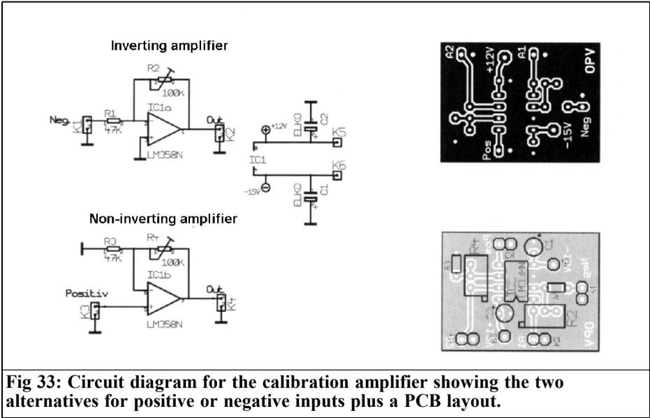
**Fig 33: Circuit diagram for the calibration amplifier showing the two alternatives for positive or negative inputs plus a PCB layout.**
