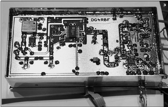
**Fig 26: Completed PLL/DDS unit.**
