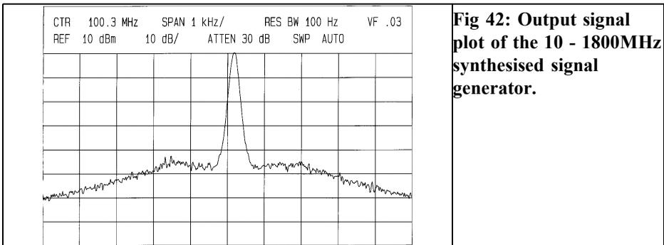
**Fig 42: Output signal plot of the 10 - 1800MHz synthesised signal generator.**
