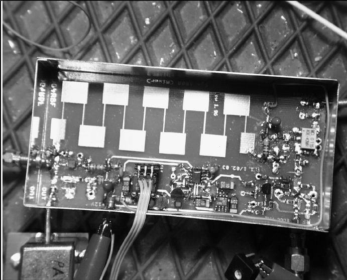
**Fig 17: Picture of the completed mixer assembly.**
