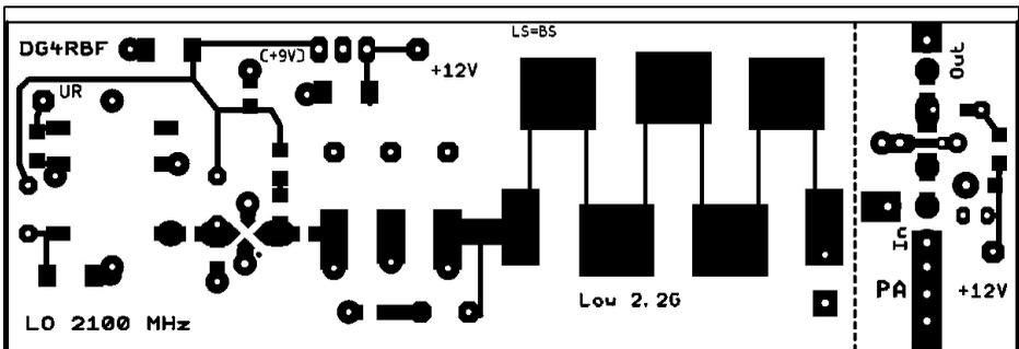
**Fig 11: PCB layout of the VCO and PA boards.**
