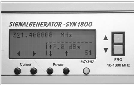
**Fig 37: Display showing the five operating buttons.**
