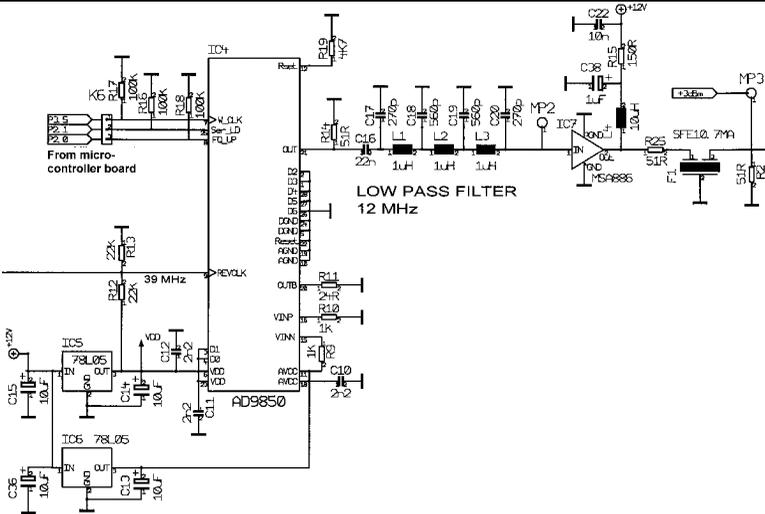
Fig 20: Circuit diagram of the DDS section of the PLL/DDS assembly.
