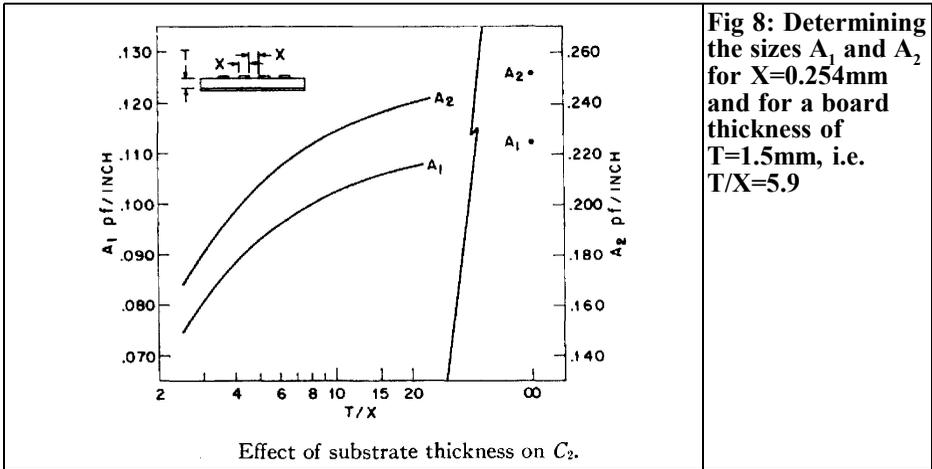
**Fig 8: Determining the sizes  $A_1$  and  $A_2$  for  $X=0.254mm$  and for a board thickness of  $T=1.5mm$ , i.e.  $T/X=5.9$**
