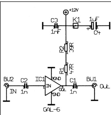
**Fig 18: Circuit diagram of the GAL-6 output amplifier.**
