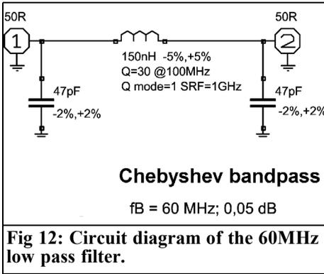
**Fig 12: Circuit diagram of the 60MHz low pass filter.**
