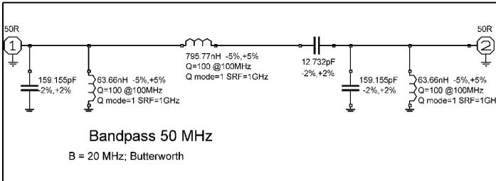
**Fig 8: Circuit diagram of the 50MHz bandpass filter.**
