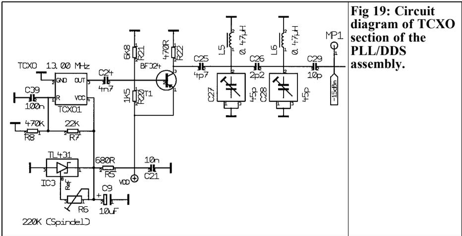
**Fig 19: Circuit diagram of TCXO section of the PLL/DDS assembly.**
