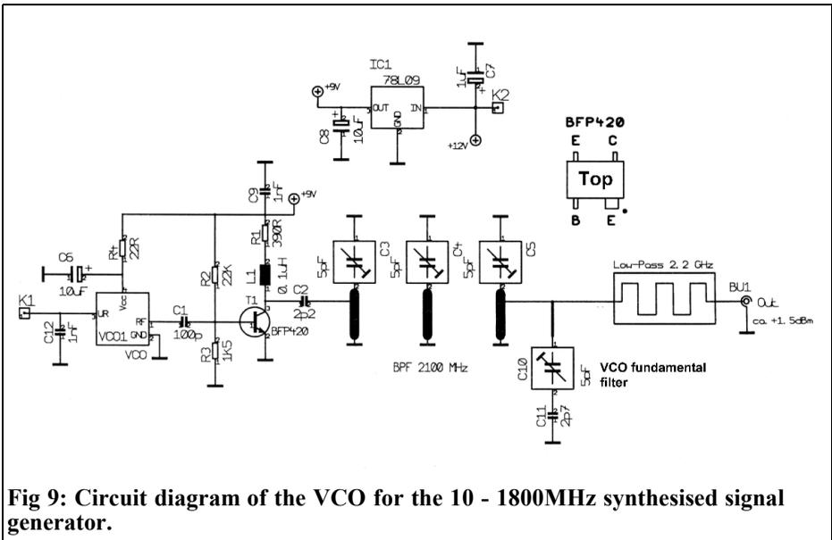
**Fig 9: Circuit diagram of the VCO for the 10 - 1800MHz synthesised signal generator.**
