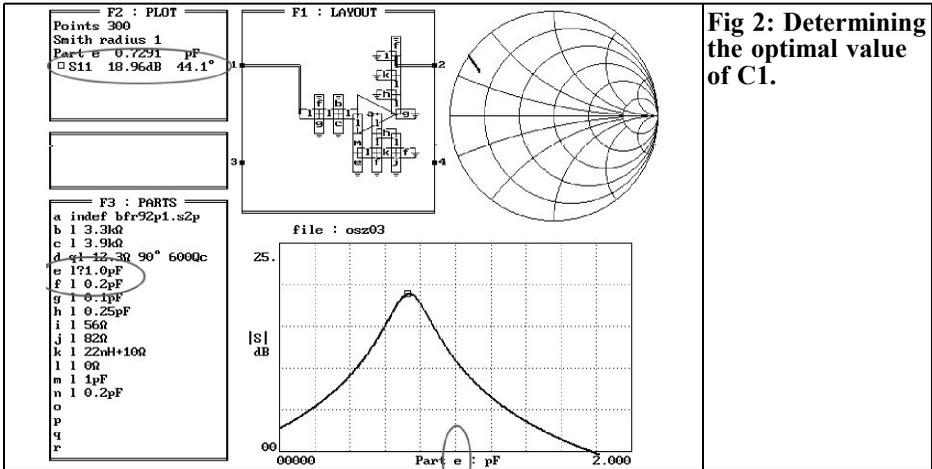
**Fig 2: Determining the optimal value of C1.**
