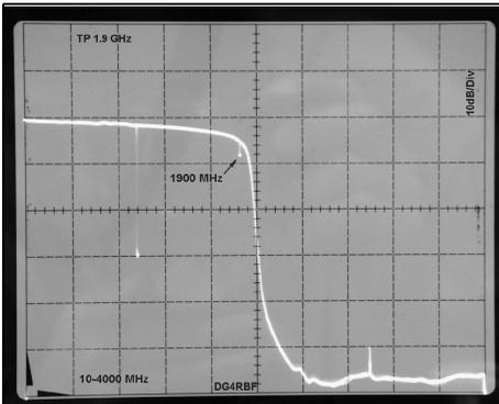
**Fig 14: Frequency response of the 21 pole filter at the output of the mixer.**
