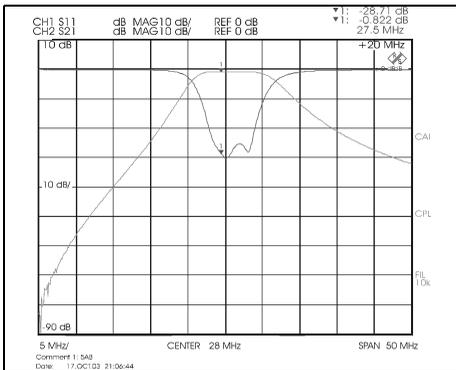
**Fig 20: Measured response of the 28MHz bandpass filter.**
