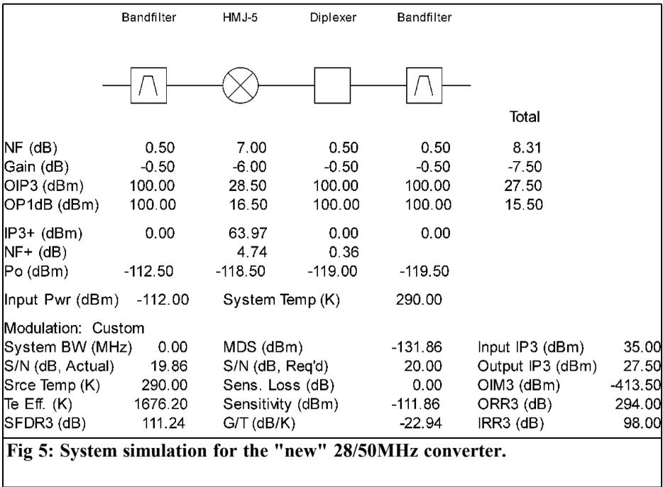
replaced by a cable attenuation of 2dB (e.g. approximately 30m RG 213) and an insertion attenuation of 0.5dB for each band filter and for the diplexer, we then obtain the following results for the system calculation for the new converter; see Fig. 5 and Table 4, column 2.
