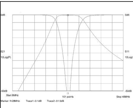
**Fig 19: Simulated response of the 28MHz bandpass filter.**
