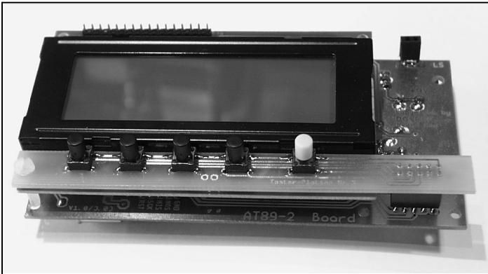
**Fig 4: View of the LCD display mounted on top of the micro-controller board.**
