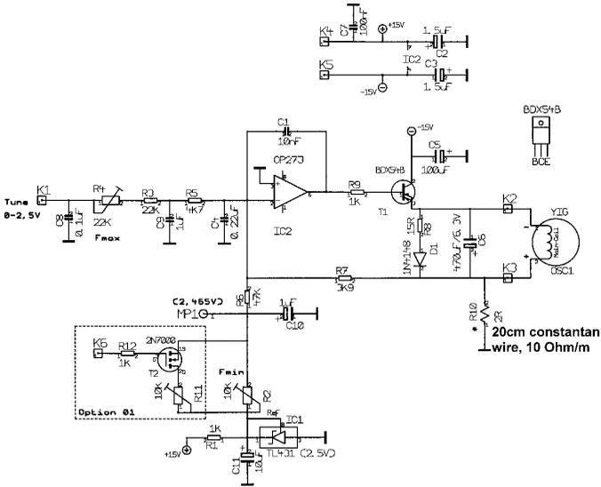
Fig 28: Circuit diagram of the YIG driver.
