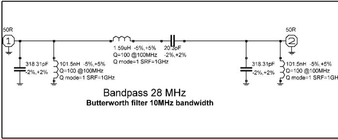
**Fig 18: Circuit diagram of the 28MHz bandpass filter.**
