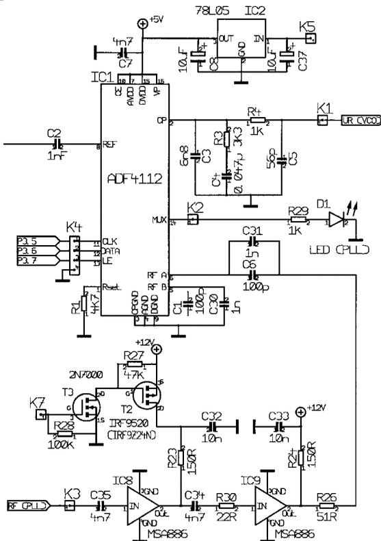
Fig 21: Circuit diagram of the PLL section of the PLL/DDS assembly.
