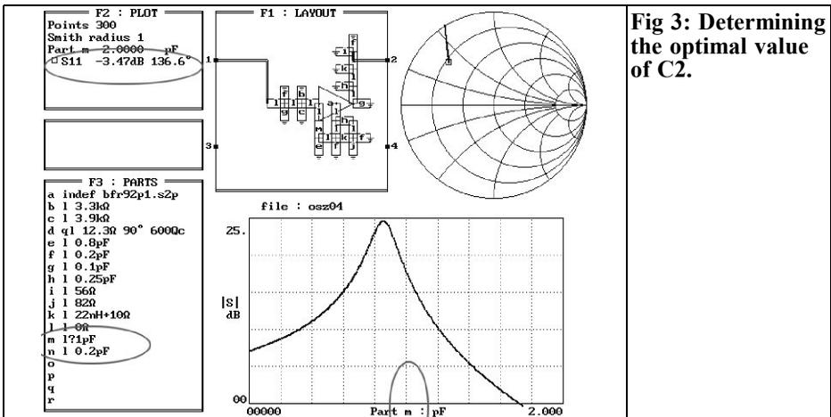
**Fig 3: Determining the optimal value of C2.**
