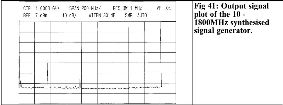
**Fig 41: Output signal plot of the 10 - 1800MHz synthesised signal generator.**
