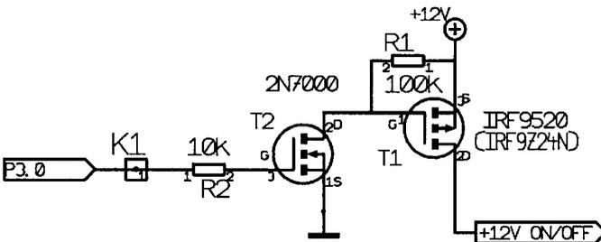
**Fig 32: Circuit diagram for the RF On/Off control.**
