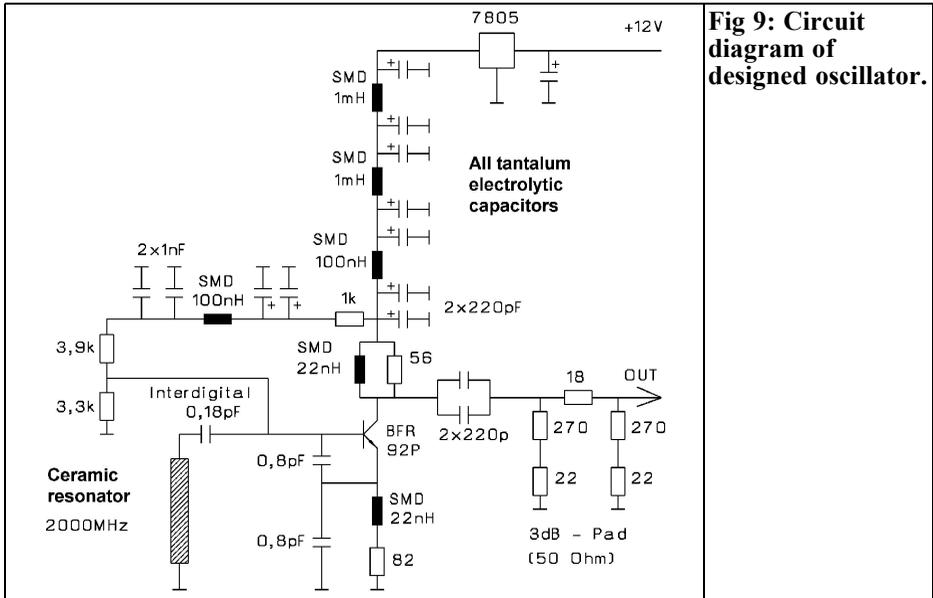
**Fig 9: Circuit diagram of designed oscillator.**
