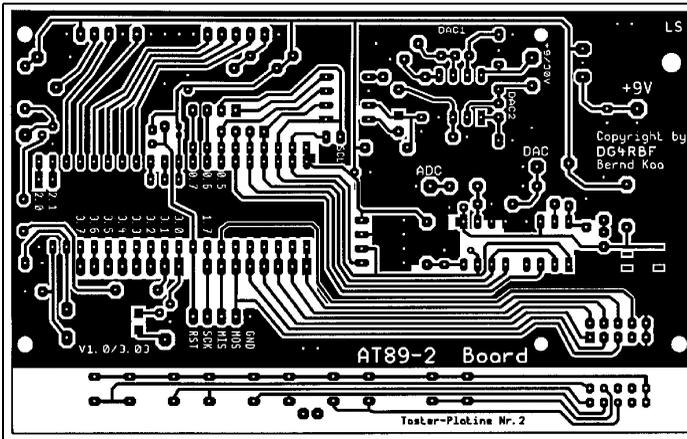
**Fig 6: PCB layout for the AT89-2 micro-controller board.**
