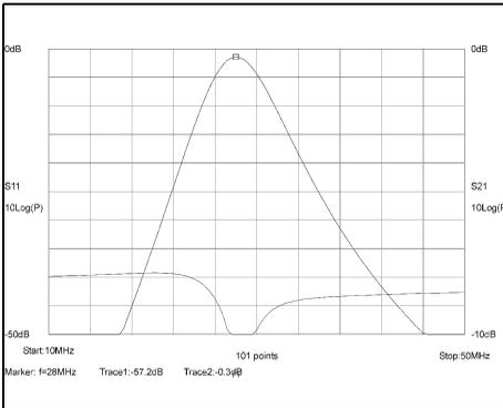
**Fig 27: Simulated performance of the diplexer.**
