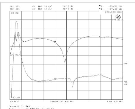
**Fig 29: Measured performance of the diplexer.**
