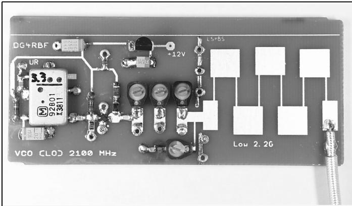
**Fig 10: The completed VCO board.**
