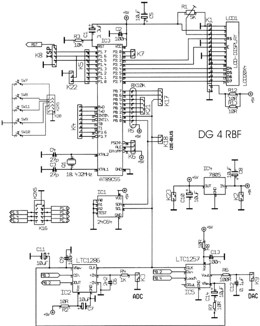
Fig 3 Circuit diagram of the new micro-controller for the 10 - 1800MHz synthesised signal generator.
