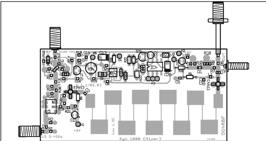
Fig 16: Component layout of the mixer.
