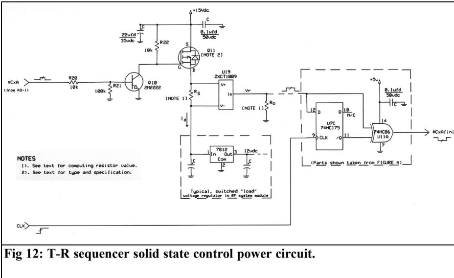
**Fig 12: T-R sequencer solid state control power circuit.**
