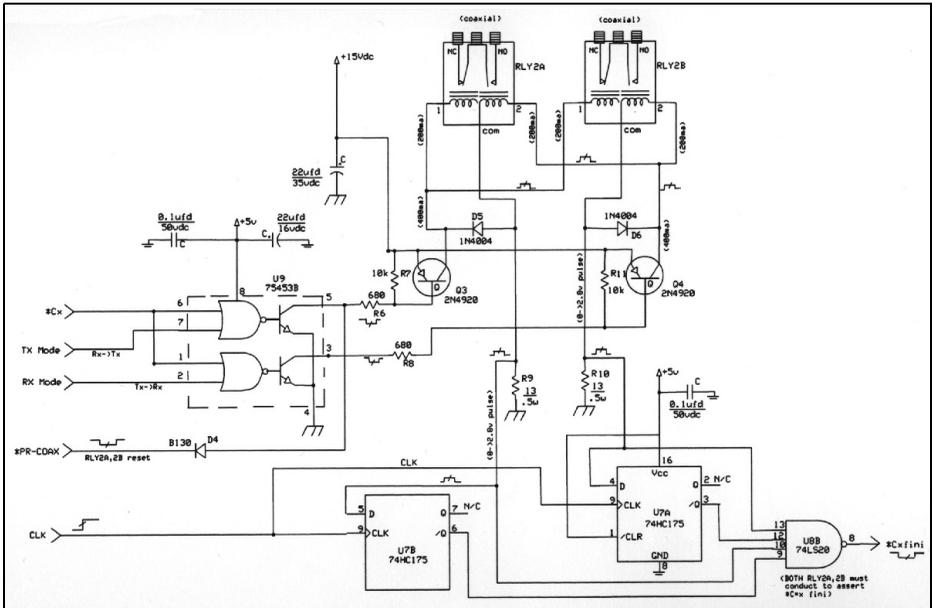
**Fig 5: T-R sequencer dual pulse latching coaxial relay.**
