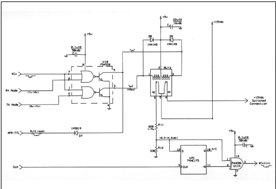
**Fig 6: T-R sequencer sequence control circuit.**
