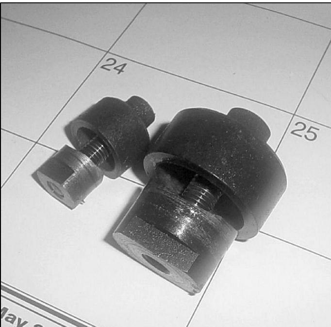
**Fig 4: Chassis punches.**
