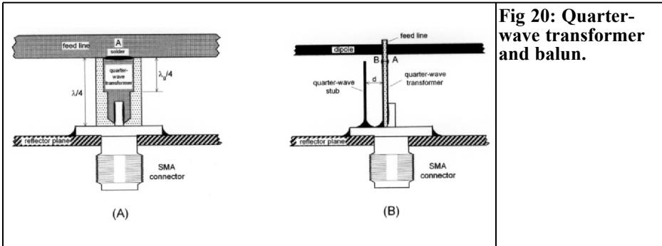
**Fig 20: Quarter-wave transformer and balun.**
