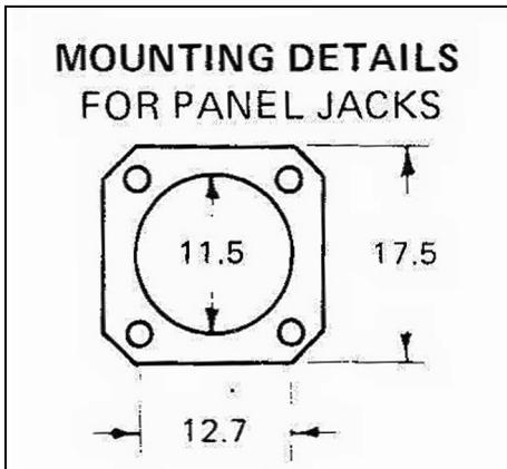
**Fig 2: BNC 4-hole connector details.**
