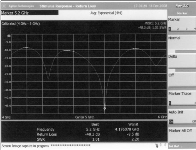
**Fig 22: Return loss measured.**
