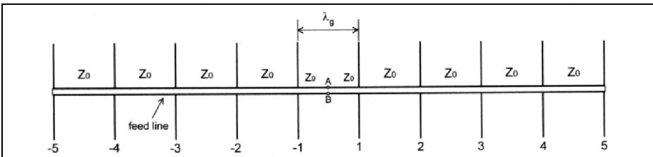
**Fig 15: Feed line with uniform impedance.**
