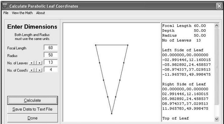
Fig 6: Parabola Leaf calculator results screen.
