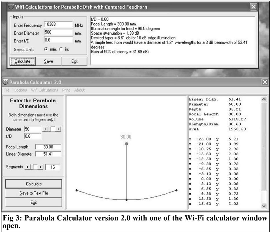
**Fig 3: Parabola Calculator version 2.0 with one of the Wi-Fi calculator window open.**
