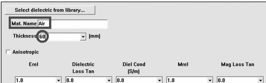
**Fig 10: The area above the PCB in the box is filled with a thick air layer. See text**
