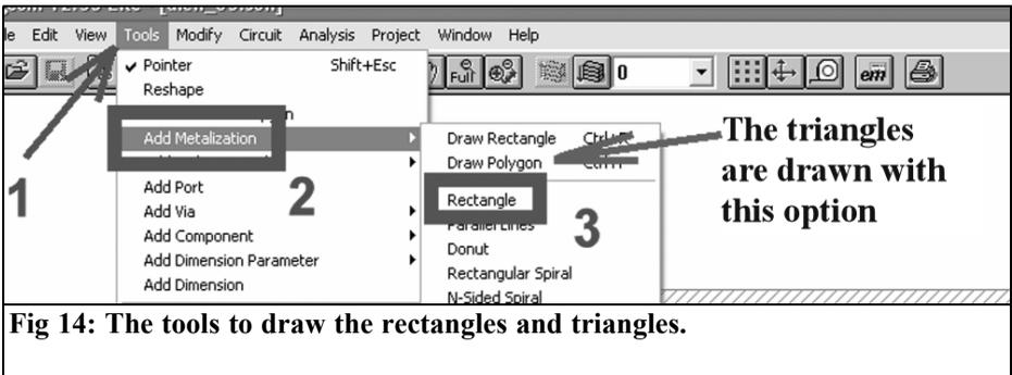
**Fig 14: The tools to draw the rectangles and triangles.**
