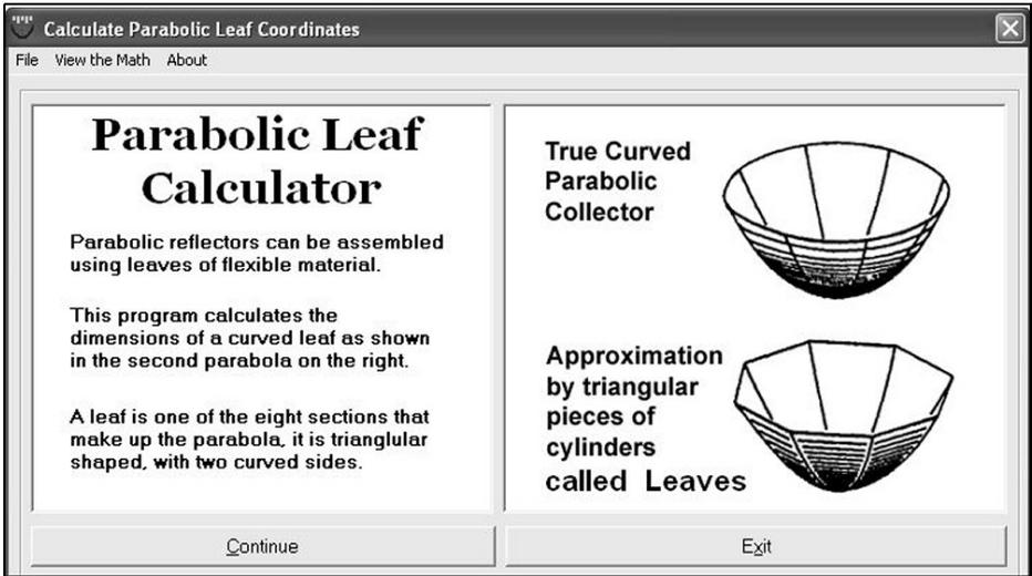
Fig 5: The opening screen of Parabola Leaf Calculator.
