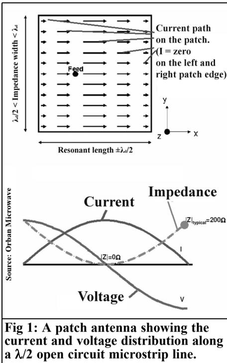
**Fig 1: A patch antenna showing the current and voltage distribution along a  $\lambda/2$  open circuit microstrip line.**
