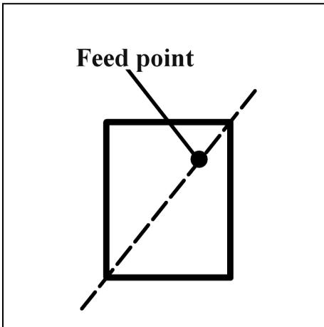
**Fig 4: First possibility: Length and width of the patch are different, the feed point lies on the diagonal. See text**
