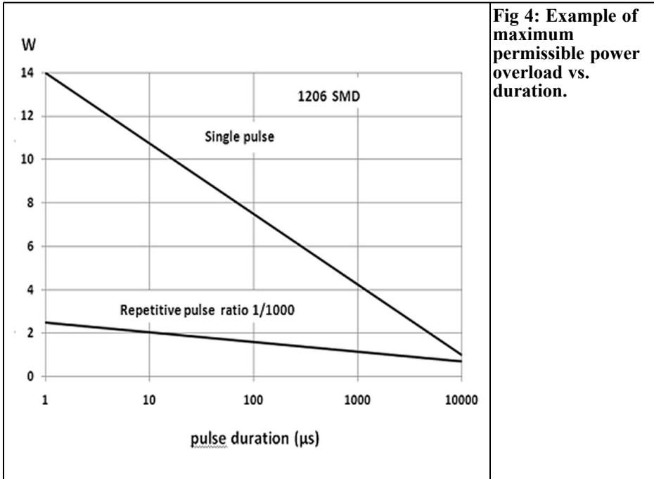
**Fig 4: Example of maximum permissible power overload vs. duration.**
