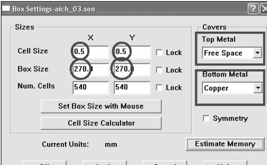
**Fig 12: Very important: the entries for the cell size and the box dimensions as well as “free space” for the cover. See text.**
