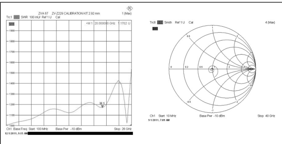
**Fig 15: Professional 50Ω SMA load.**
