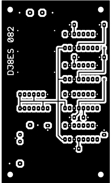
Fig 5: Bottom side PCB layout for the driver module.
