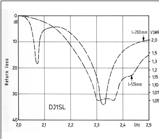
**Fig 4: Matching of a tubular radiator in a frequency range from 2.0 to 2.5GHz.**
