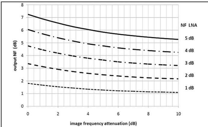
**Fig 8:  $NF_{out}$  vs  $NF_{LNA}$  for various image frequency attenuations.**
