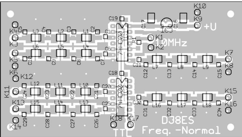
Fig 11: The component layout for the six 10MHz output PCB.
