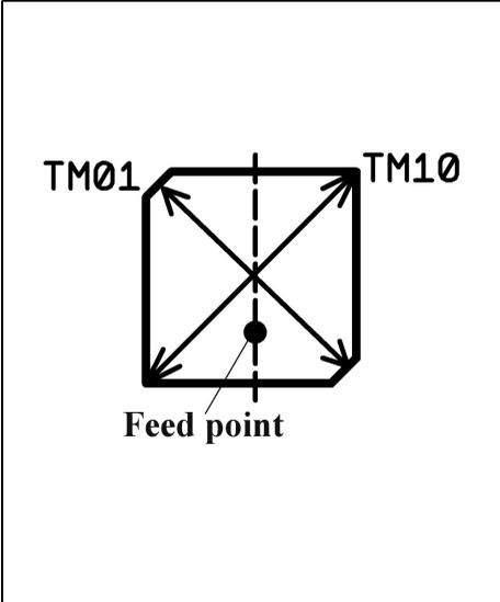
**Fig 6: Third and most popular possibility: the corners are cut at 45 degrees, otherwise the same as Fig 5.**
