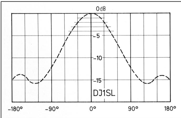
**Fig 5: Radiation diagram (E plane) of the tubular radiator.**
