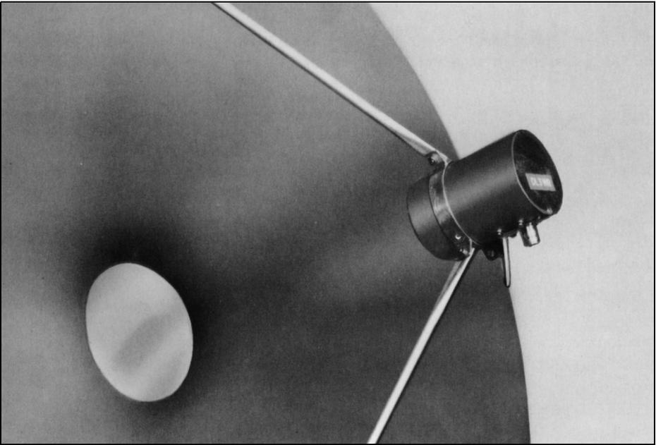
**Fig 6: 1.2 meter parabolic with tubular radiator for the 13cm band ( $G_{\text{dipol}}$  approx. 24 - 25dB).**
