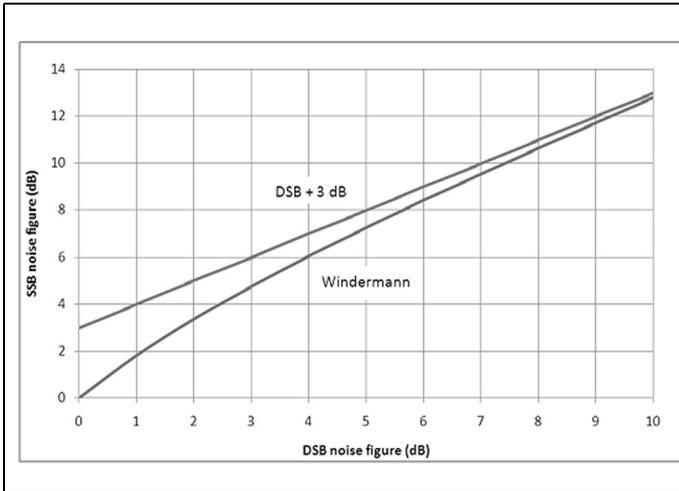
**Fig 6: True SSB figure and DSB +3dB versus DSB figure.**
