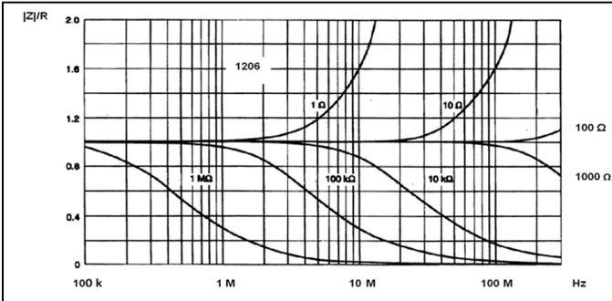
**Fig 9: Example of SMD thick layer 1206 behaviour vs. frequency.**
