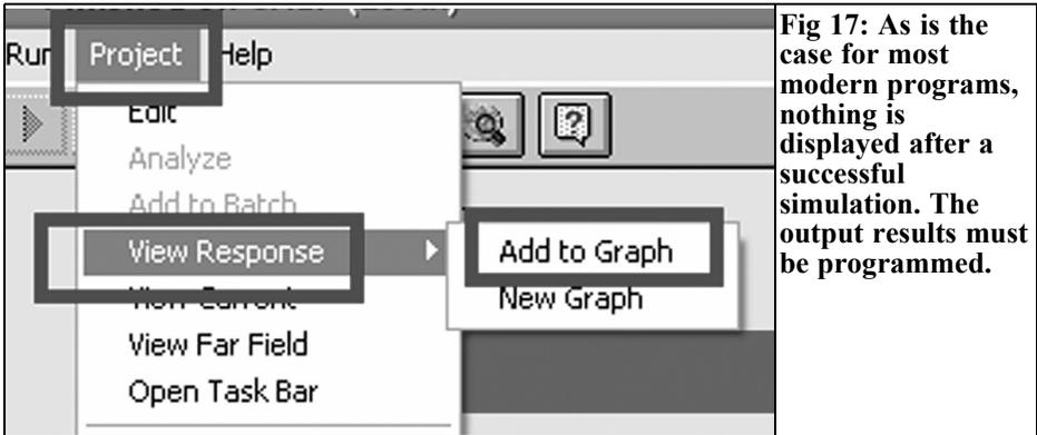
**Fig 17: As is the case for most modern programs, nothing is displayed after a successful simulation. The output results must be programmed.**
