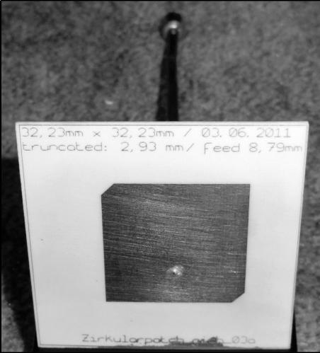
**Fig 23: The final result, the prototype antenna, measured and given to the model flier.**
