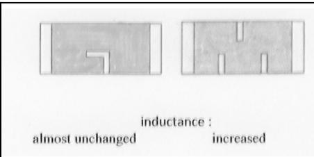
**Fig 10: Chip resistor trimming.**
