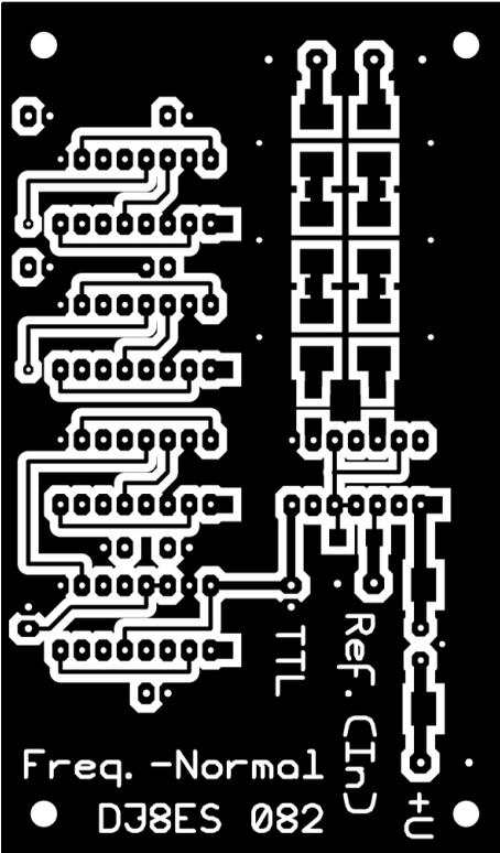
Fig 4: Top side PCB layout for the driver module.
