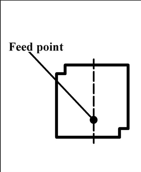
**Fig 5: Second possibility: the patch is square with the corners punched out, the feed point is on the centre line.**
