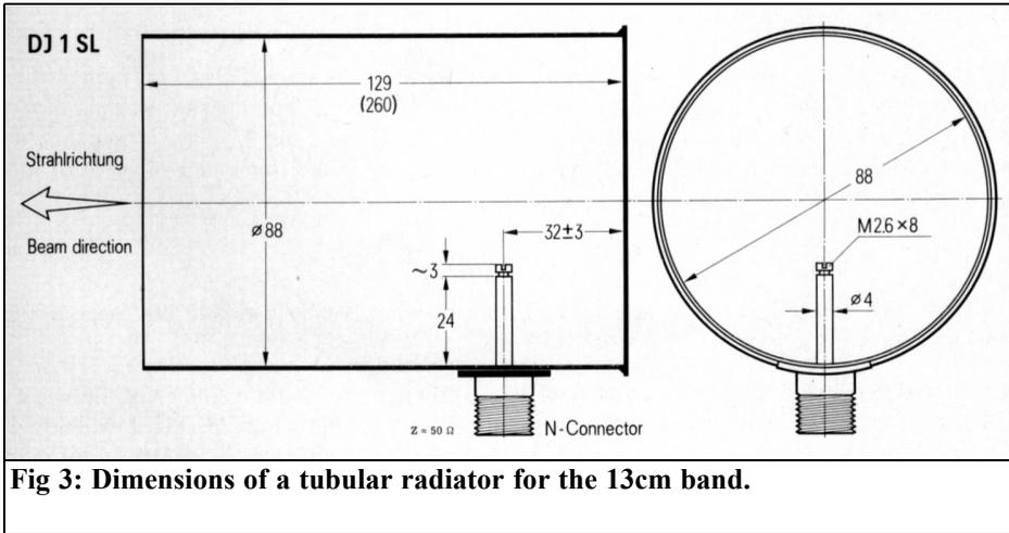
**Fig 3: Dimensions of a tubular radiator for the 13cm band.**
