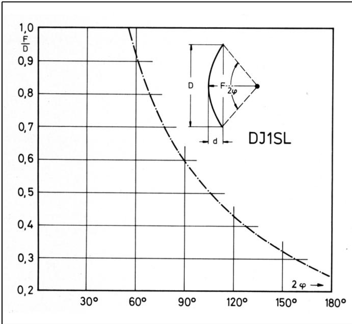
Fig 1: Focal angle of parabolic antennas as a function of F/D.
