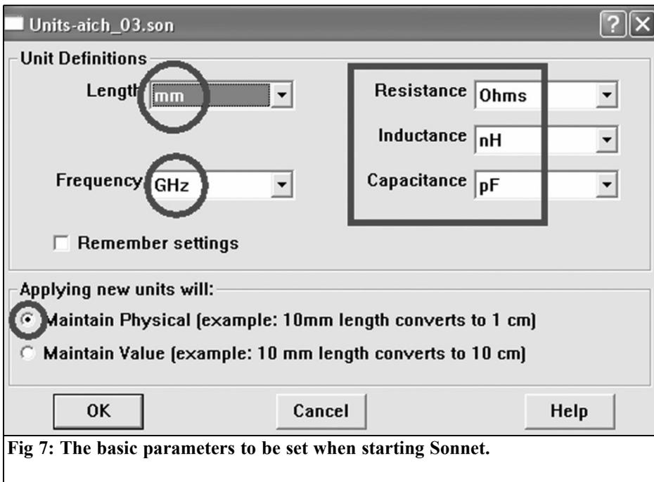
Fig 7: The basic parameters to be set when starting Sonnet.
