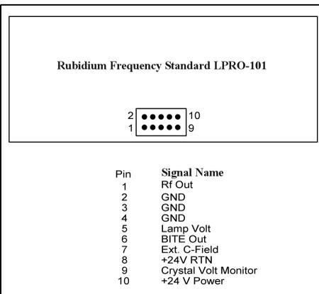
**Fig 2: Pin connections for the 10 way connector on the LPRO-101.**
