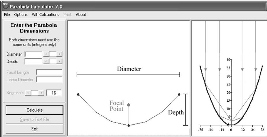
Fig 1: The opening screen of Parabola Calculator version 2.0.
