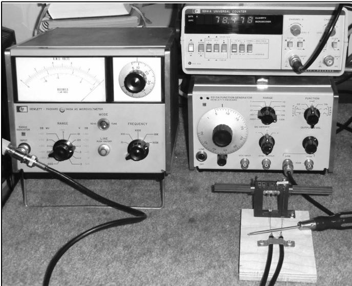
**Fig 5: The equipment used to measure the coil losses and Q.**
