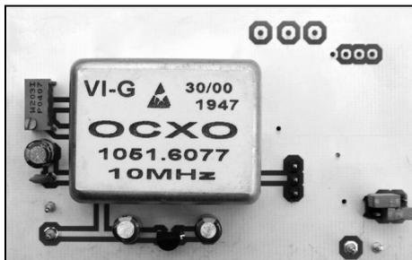
Fig 1: Example of a 10MHz OCXO,
