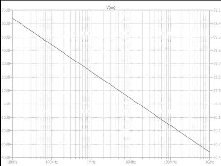
**Fig 15: The frequency response of the Integrator shown in Fig 14.**
