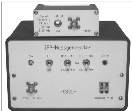
**Fig 13: IP3 generator with a maximum output signal of 2 x +13dBm.**
