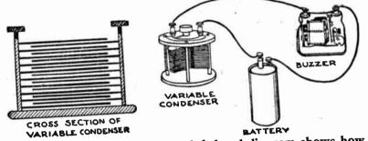
How to test a condenser. The left-hand diagram shows how the plates are arranged. There is no electrical connection between the two sets of plates. To the right is the hook-up for testing as explained in the article.
