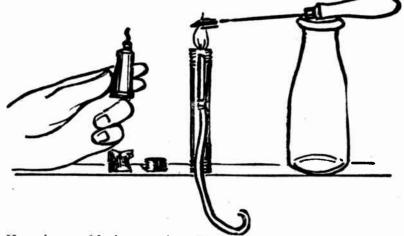
Here is a soldering outfit. The hand is holding a tube of "dope" or "salts"; under it is a piece of solder, next the cap that screws on the alcohol torch, next the torch itself and then the soldering iron resting on a milk bottle.
