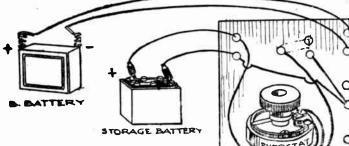
This shows the complete "hook-up" for the audion bulb control panel with the two batteries necessary for its operation. The illustration makes clear the method of wiring and the article explains its operation.
