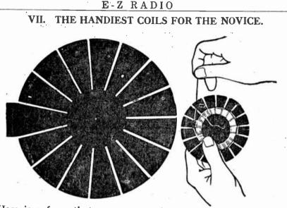
Here is a form that you can use for cutting out the cardboard to make spider-web coils. On the right, the picture shows the method of winding them.
