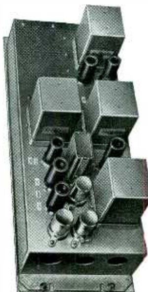
▲ LINE AMPLIFIER with inter-stage plug-in equalization
