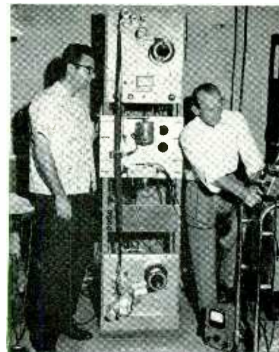
Left: The first closed circuit demonstration of a VR-1000A recorder abroad being given in May 1958, at Associated-Rediffusion Limited in London. Right: Alex Maxey and Kurt Machein are shown with the first one-headed "hoo ha". The tape is four inches wide and is shaped into an overlapping tube. The single scanning head inside the female guide is belt driven by an external motor.
