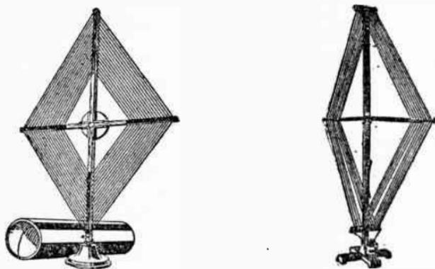
Fig. 7. Two loop aerials. The one on the left is known as the spiral type and the one on the right, the Solenoid type.
