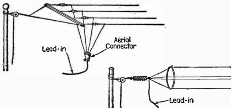
Fig. 3. Insulating multi-wire aerials. Note the location of the insulators and the place where the lead-in is taken off from in each case.
