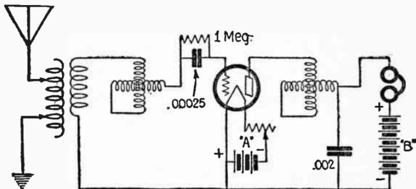
Fig. 22. The three circuit tuner regenerative circuit.
