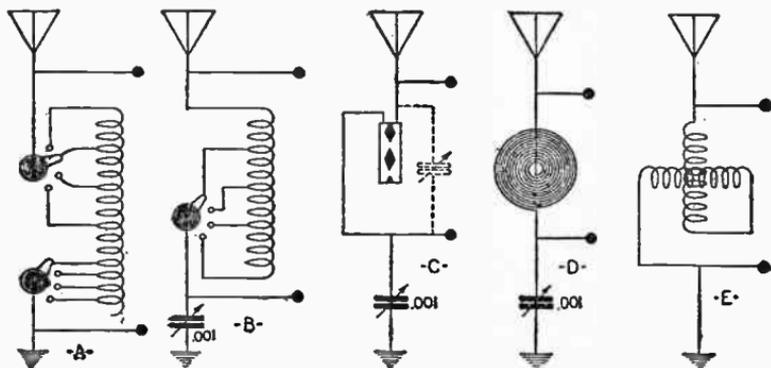
Fig. 9. How inductances and capacities may be used to tune the aerial circuit.
