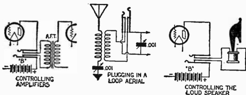
Fig. 34. Several applications of the double circuit jack.
