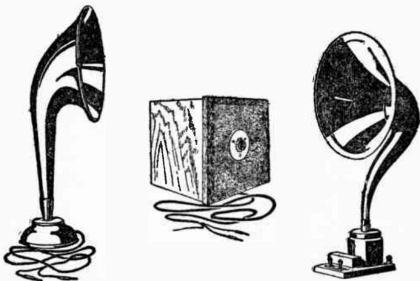
Fig. 36. Popular types of loud speakers. They are, in order, the receiver unit, adjustable, and power talkers.
