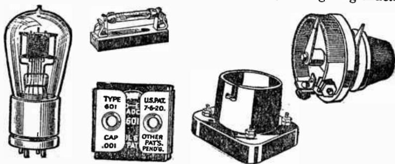
Fig. 16. A vacuum tube and component parts which are used in conjunction with it as a detector. A grid leak, condenser, socket, and a rheostat are shown to the right of the tube.
