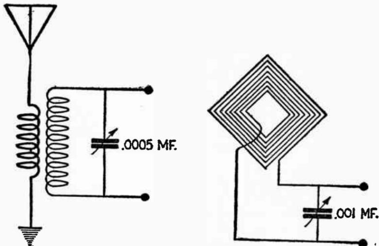
Fig. 12. The untuned primary circuit and method for tuning a loop aerial.
