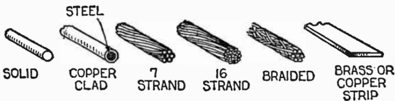
Fig. 1. Cross-sectional view of the various conductors used for aerials.
