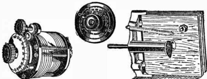
**Fig. 13.** Variable condensers of the three styles as mentioned. Left to right they are, the intersecting plate with vernier device, the mica dielectric, and the book type.
