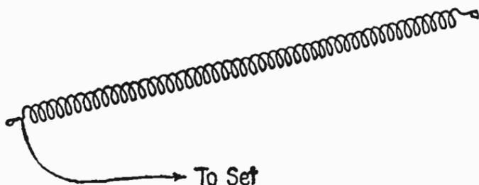
Fig. 6. The spring antenna is installed by simply stretching it between two opposite corners of a room and bringing a lead down to the set.
