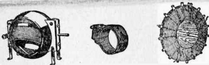
Fig. 8. Three arrangements of inductances. On the left is shown a variometer, in the center a honeycomb coil, and on the right a spiderweb coil.
