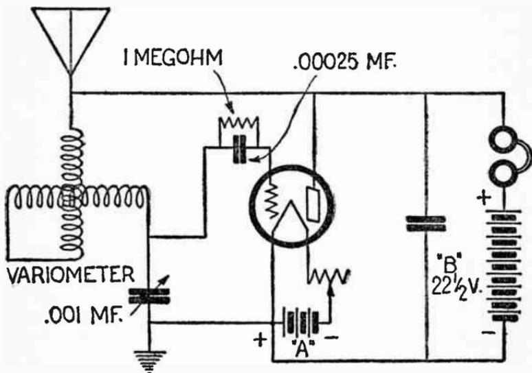
Fig. 21. An ultra audion circuit illustrating capacitive feedback.
