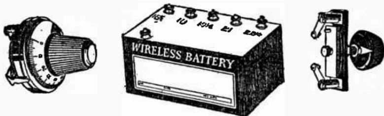
Fig. 18. A vernier rheostat, variable "B" battery and variable grid leak are employed to obtain more accurate adjustment of the vacuum tube.
