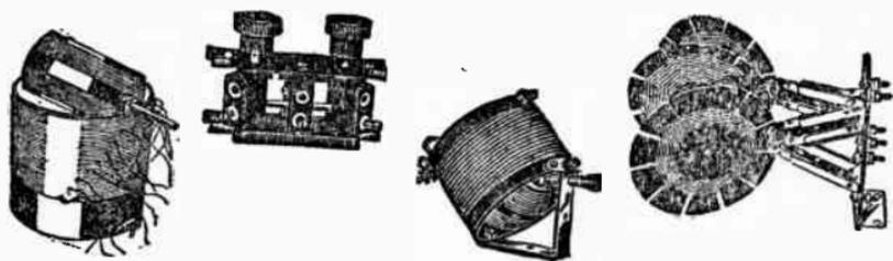
Fig. 10. Coupling devices as used for varying the relation of inductances or coils.
