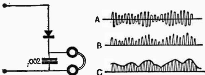
Fig. 15. Connections of a crystal detector and graphs showing rectification of radio frequency currents and the resultant audio frequency current that actuates the phones.
