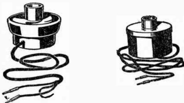
Fig. 35. Loud speaker units adapted to attach to a phonograph.
