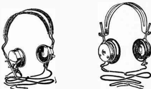
Fig. 32. Telephone headsets especially designed for radio purposes.
