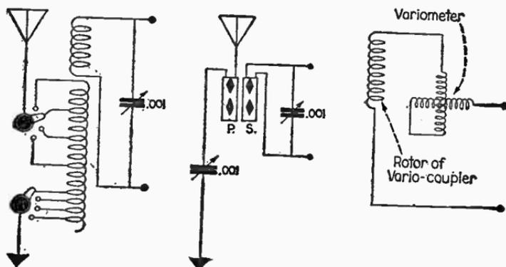
Fig. 11. How coupled circuits are connected and tuned. The first is a tapped vario-coupler, the second honeycomb coils, and a third a variometer.
