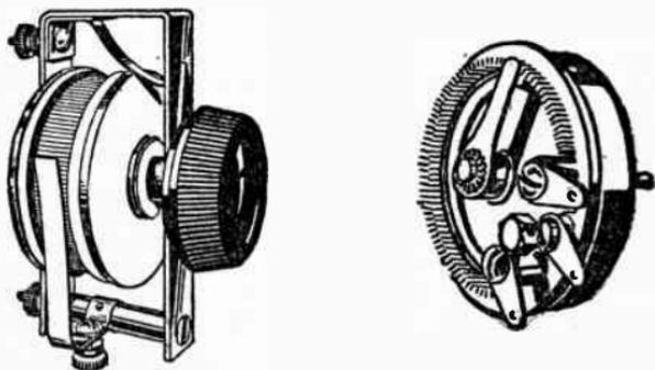
Fig. 25. Potentiometers are used to control the potential or voltage supplied to the radio circuit.
