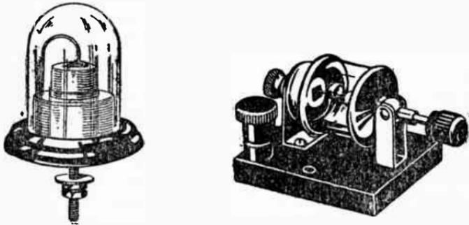
Fig. 14. A fixed and an adjustable crystal detector.
