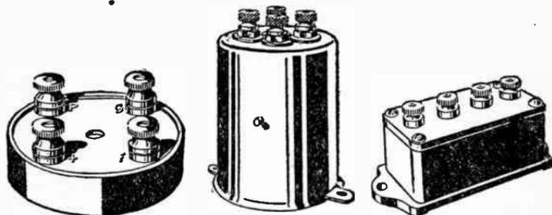
Fig. 23. Types of radio frequency transformers for amplifying the radio currents before being detected.
