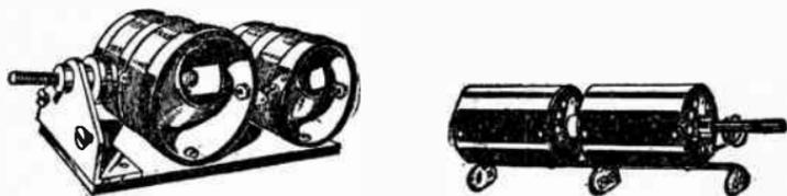
**Fig. 27.** Two forms of adjustable transformers for radio frequency amplification.
