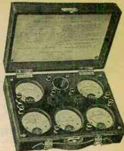
No. 95. A complete testing instrument in connection with a radio receiving set. Particularly adapted for the taking of characteristic curves on vacuum tubes, the only extra equipment being the necessary batteries. The several instruments, any of which may be used independently, include a 0-1.2 filament ammeter, a 0-6 filament voltmeter, a 0-150 plate voltmeter, a 0-10 plate milliammeter and a 25-0-10 grid voltmeter. No. H2110—**\$75.00**
