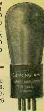
CX310—Cunningham heavy duty power amplifier. Oscillator—Fil. volts 7.5, fil. amps. 1.25, plate volts 350, plate amps. .06, output 7.5 watts. Amplifier—Fil. volts 6.75, fil. amps (max.) 1.25, plate volts (max.) 425. Stock No. H2896—List .....\$9.00
