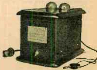
Operates on 60 cycle 110 volt electric current and acts both as "B" eliminator and power amplifier on any set. Takes weak signals from set and amplifies them to tremendous volume, if desired, without distortion. Supplies up to 135 volts "B" current. Employs 216-B or 316-B rectifier tubes and 210 or 310 tubes for amplification.
