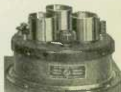
Detector 2-Stage Amplifier
