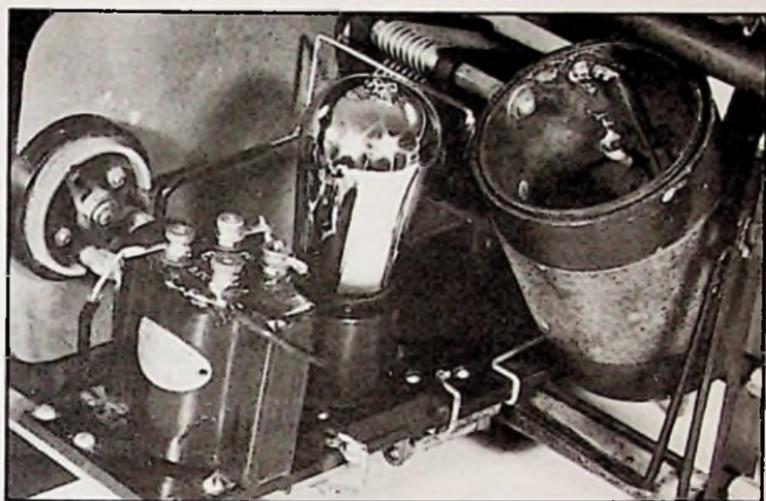
14. Grid Leak Detector (Freed-Eisemann). The AF transformer and filament rheostat are to the left of the tube. To the right is the third RF transformer and tuning capacitor. The grid leak resistor is below the bakelite mounting board and the capacitor is above behind the tube base. Note the RF transformer primary wound on a smaller form inside the secondary.
