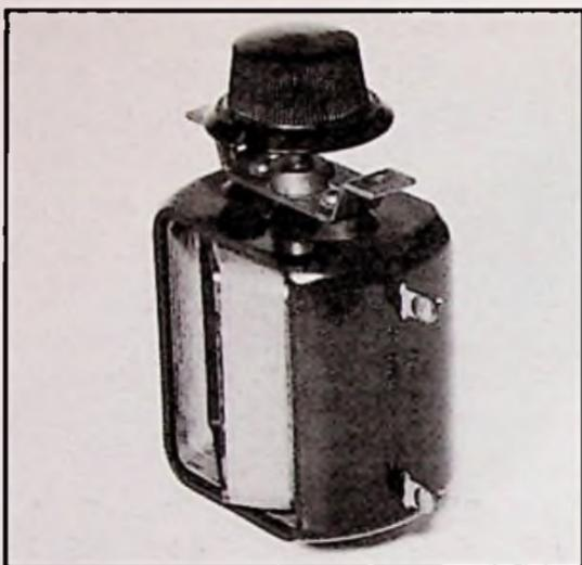
1. *Variometer (General Radio). This compact unit has the stationary coil wound inside the outer bakelite form. Connections to the rotary coil are made through stub shafts at each end of the unit.*
