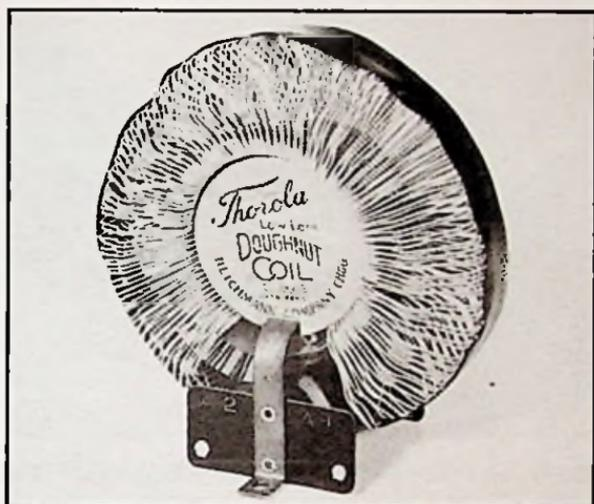
6. Doughnut Coil (Thorola). This coil is self supporting and its toroidal shape minimized coupling. The primary winding is wound between the secondary turns at one end.
