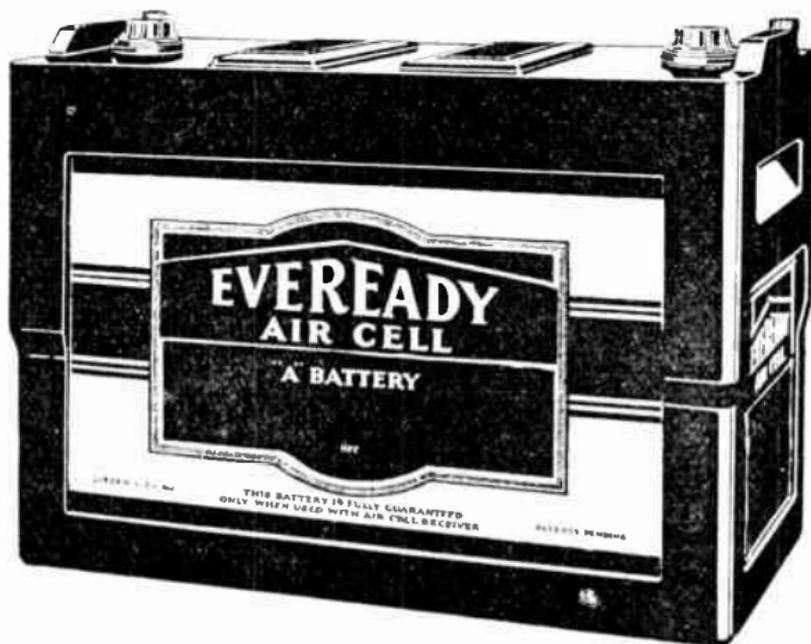
The Eveready Air Cell "A" Battery uses a liquid electrolyte, but is shipped dry. In the dry state, it undergoes no depreciation. It can be activated for service at any time after manufacture and still deliver its full quota of ampere hours. It is activated for service by filling with water.
