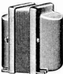
No. 104—110-115 volt primary with four secondaries. No. 1—400-0-400 volts, 100 M.A.; No. 2—2½ volts, 12 amps.; No. 3—2½ volts, 3 amps.; No. 4—5 volts, 2 amps.
