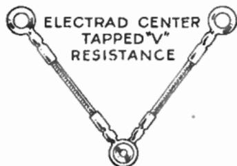
Particularly designed for use across the filaments of A. C. tubes—the center tap providing the electrical center for grid return leads. Made by riveting two matched resistors together—resulting in an unusually accurate center tap. Can be used with any type A. C. tube socket. Total Resistances 10, 20, 30, 40, 50, 80, 100, 150, and 200 ohms. List \$0.50 .....NET \$0.29
