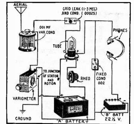
one-half of the total inductance of the variometer tunes the antenna circuit. Therefore, this instrument should be of quite a large size.
