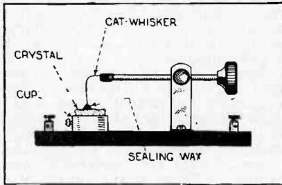
will hold the cat's whisker on it. Jars and jolts will not affect it. You will have, to all purposes, a fixed crystal, but one which easily can be adjusted by removing the wax and reapplying.
