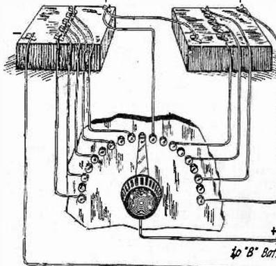
that the purpose of the dead contacts is to prevent short circuiting the cells of the battery in case the switch is left touching two adjacent contacts.
