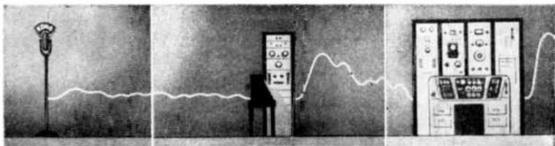
*These pictures show how a KDKA radio program is transmitted and received. Sound waves striking the microphone produce a current of varying intensities. This is sent to the control room, where it is amplified, and then to the master control room, where it is amplified again.*
