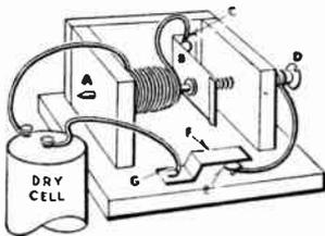
4. With a few simple materials, you can make a Code buzzer. *A* is a nail with about a hundred turns of insulated bell wire around it. *B* is a strip about 3 inches long from a tin can. The free end is about  $\frac{1}{8}$  inch away from the end of nail *A*. The other end is held firm by tack *C*, to which the wire from *A* is connected. *D* is a screw or bolt so adjusted that it presses against the free end of strip *B*.
