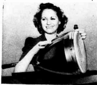
*The kinescope converts electrical impulses into pictures.*
