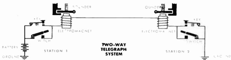
*Here is a two-way telegraph system. When Station 1 wishes to receive, he closes his switch. Station 2 now uses his key to open and close the circuit and send signals. When the key is down, the electromagnets pull down a metal bar in the sounder. When the key is up, the bar springs back. After Station 2 has completed his message, he closes his switch, and is ready to receive. Station 1 opens his switch, and is ready to send.*
