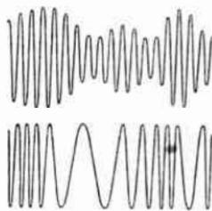
*In AM, amplitude modulation (top), the amplitude, or strength, of the carrier wave is varied by the voice current, but its frequency is constant. In FM, frequency modulation (below), the frequency of the carrier wave is varied, but the strength is constant.*
