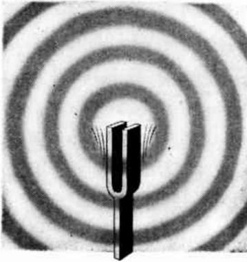
*A vibrating object sends out ripples of dense and rare air. These are sound waves. The pitch of the sound we hear when the waves strike our ear depends on the frequency of the waves—the number that strike our ear in one second. The ear responds to waves with a frequency lower than 10 cycles a second (very low notes) and as high as about 20,000 cycles a second (very high notes.)*
