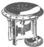
The S-L-F condensers used to tune the various stages of amplification are one of the features of the Synchrophase. Due to their scientifically shaped plates all broadcasting stations are found spaced at equal intervals along the dial scale. By this arrangement the tendency of crowding of stations along the lower end of the dials is materially avoided.
