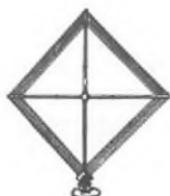
Oftentimes, it is desirable to use a loop aerial because of the advantages of its directional effect which sometimes assists to increase the selectivity of the instrument, particularly when close to broadcasting stations using considerable power. While a loop has these advantages, it should be remembered that they do not receive signals with volume comparable to outside aerial reception.
