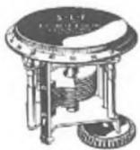
The S-L-F condensers used to tune the various stages of amplification are one of the features of the Synchronphase. Due to their scientifically shaped plates all broadcasting stations are found spaced at equal intervals along the dial scale. By this arrangement the tendency of crowding of stations along the lower end of the dials is materially avoided.
