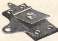
A small neutralizing or balancing condenser, having an exceptionally wide capacity range. Very useful as a compensator for equalizing the units of a multiple-tuning condenser. May be attached directly to socket binding posts or condensers, thus simplifying wiring connections.
