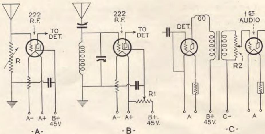
Figure 7—Three suggested volume controls for short wave receivers. Circuit A applies to coupling tubes and circuit B to tubes having a tuned input circuit. Circuit C gives an absolute low signal position and is very satisfactory where the signal does not overload the detector tube. The regeneration control should be used with all three as an added volume control for best results.
