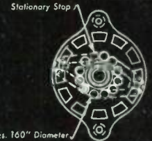
11 Holes, 160" Diameter for Adjustable Stop.
