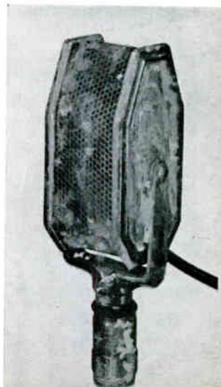
Fig. 3. A velocity microphone under water in the Ohio flood for ten days was found to be in good operating condition when recovered.
