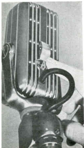
Fig. 1. A sliding panel that gradually closes the back of the microphone changes it from velocity to pressure operated. Closing the back of the velocity makes it higher pitched.
