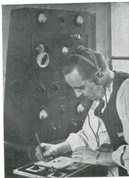
Calibrating a Weston test oscillator dial scale to match the individual oscillator circuit.
