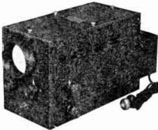
Provides an instantaneous graphic picture of the actual operating conditions in transmitter circuits. Percentage Modulation, Signal Distortion and Peak Voltages are indicated directly, and results are easily interpreted.
