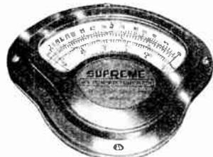
Model 310. A 5" d'Arsonval meter especially designed and built for universal application in radio testing equipment. Provides easy reading over a range 26% longer than the usual meter scale. Fan-shaped bakelite housing moulded for semi-flush mounting. Mounts in circular hole. Dimensional drawing supplied with each meter.
