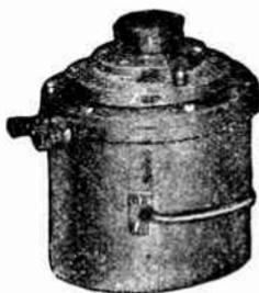
MASTER Racon dynamic horn unit has a continuous rating of 20 watts, peak of 50 watts. 6-8 volt field excitation at 1.1 amp. 15 ohm voice coil. Wt. 13½ lbs. Net.....\$25.88
