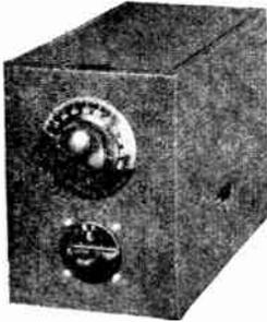
For use with either superheterodyne or TRF Receivers. Designed for use with FB-7, it is equally effective with SW-3 and other receivers. It provides additional selectivity and additional gain and weak signal response. Reduces image frequencies in superheterodynes. Power supply is not critical and may be obtained from the receiver used. The tube may be either a
