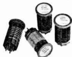
Wound on low loss XP-53 dielectric Hammarlund plug-in forms. Four coils cover the entire range of 17 to 270 meters. One more covers entire broadcast band. Windings of 17 to 41 meter and 33 to 75 meter coils are heavily
