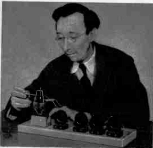
Dr. C. W. Hewlett with his "flea power" motor which is driven by the impulses of sun's rays falling on a photo-electric cell to develop one ten-millionth of a horsepower.
