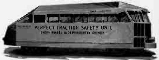
This odd bus eliminates the usual clutches and transmission to reduce maintenance costs. Each wheel is independently driven. The motor is mounted back of the rear axle.
