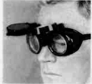
The goggles, fastened to hinge, can be raised to inspect work.
