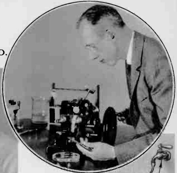
In chipping method of obtaining sections, demonstrated at left, fingernail on left forefinger controls thickness of slice. Use sliding motion when cutting to avoid tearing of delicate tissues. In circle above is rotary microtome, automatic machine used in many laboratories for preparing sections. Knife here remains stationary while object moves rapidly up and down as flywheel is turned. Arrangement of mason jar at right is for washing slices.
