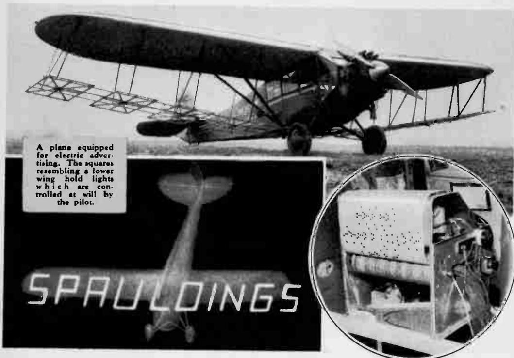
A plane equipped for electric advertising. The squares resembling a lower wing hold lights which are controlled at will by the pilot.
