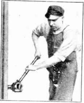
A new ratchet type pipe threader, designed for work where a two-handed threader cannot be used.
