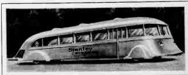
The new streamlined bus is the latest in aerodynamic design with a rear mounted motor to avoid obnoxious engine odors in passenger compartment.
