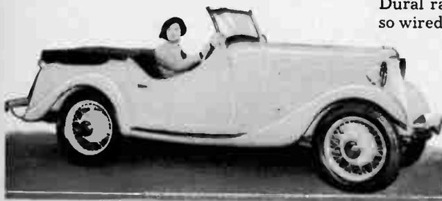
A de-luxe British Ford roadster containing a four cylinder motor which develops ten horsepower—one-eighth the power of the American Ford.
