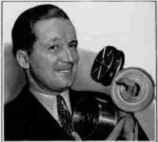
Inventor McKinley Palmer demonstrates simplicity of his new automatic clutch for autos. Device attaches to most modern cars, saves gasoline by preventing racing of engine.
