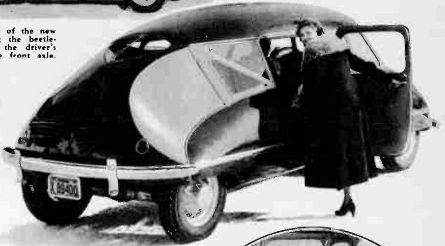
**U**LTRA streamlined, with an engine mounted in the rear, the driving mechanism over the front axle, and an interior designed like a room in a house, the most revolutionary development in the history of automobile construction was presented to the American public for the first time February 1.
