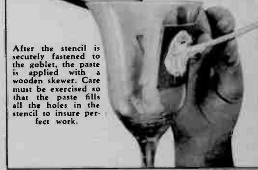
After the stencil is securely fastened to the goblet, the paste is applied with a wooden skewer. Care must be exercised so that the paste fills all the holes in the stencil to insure perfect work.
