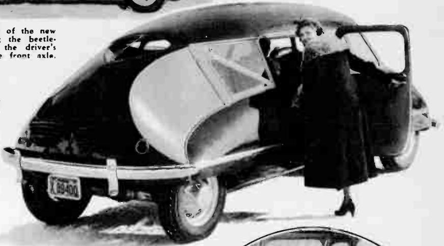
Right—The floor of the new auto is set to the level of the running board, permitting entire elimination of the running board and allowing five inches of extra overhead room within the "living room."
