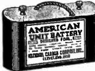
Consists of four regular size, 2 1/2 by 6-inch dry cells, connected together and sealed in an airtight container. This method of construction greatly prolongs the life of battery. Binding post connections, handle for carrying; can be used as an "A" battery. Tests 6 volts, 22 to 30 amperes. Size, 10 1/2 by 2 1/4 by 7 inches. Shipping weight, complete, 10 pounds. \$1.95
