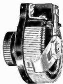
Designed especially to regulate power tube filament current. Heat-resisting, molded base, 2 1/4 inches diameter, with two concentric resistance windings which can be arranged to give four separate values of: 2.5 ohms, 1.2 amperes; 3.5 ohms, 1.2 amperes; 1.5 ohms, 2.5 amperes; 6 ohms, 1/2 ampere. Shipping weight, 1 pound. **\$3.00**
