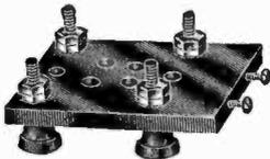
For panel or table mounting. Arranged so rheostat may be mounted between tube and panel. Bakelite construction. Binding post connections. Phosphor bronze contact springs. A convenient mounting for one or more tubes. Shipping weight, 6 ounces. **\$2.42**
