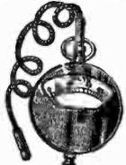
This is a special Voltmeter with a scale reading 0 to 50 volts. It will show the actual condition of your "B" battery. Tests 22 1/2 or 45-volt batteries. Polished nickel case about the size of a watch; fitted with 8 inch connecting cord. Shipping weight, 5 ounces. 97¢
