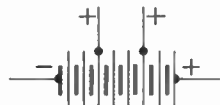
BATTERY IN SERIES. The total voltage equals the sum of the voltages of all the cells.
